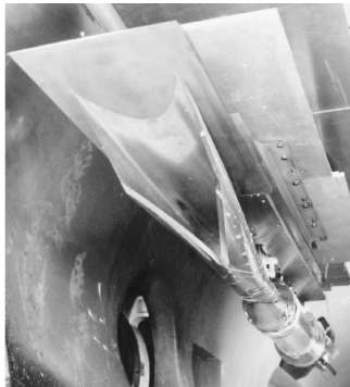
Figure 1.3: Rectangular to Elliptical Transition (REST) model with notched cowl (Smart 1999)
