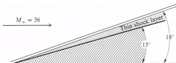
Figure 2.2: Thin shock layer (Anderson 2006)
