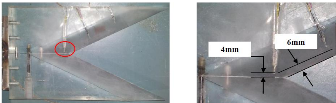
Figure 4.5: Location of functioning thermocouple for experiments
