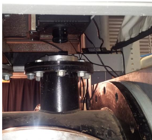
Figure 4.12: Tunnel test section closed, with IR camera focused on experimental model through Calcium Fluoride optical access window
