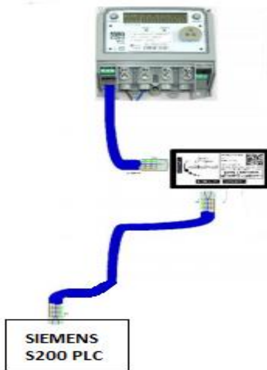
Figure 3. 2: EDM1 Modbus Translator designed by Smart Building Services (source: - Smart Building Services, 2012)
