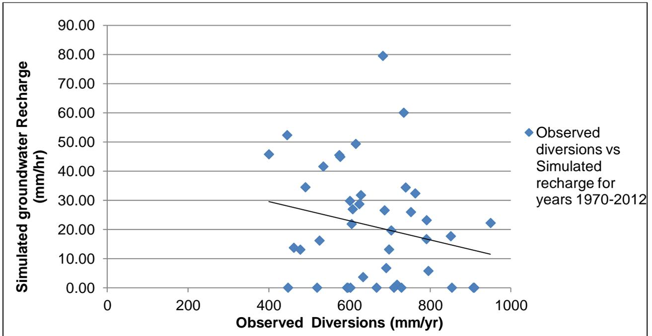
**Figure 5.4 Correlation between groundwater recharge and irrigation diversions**
