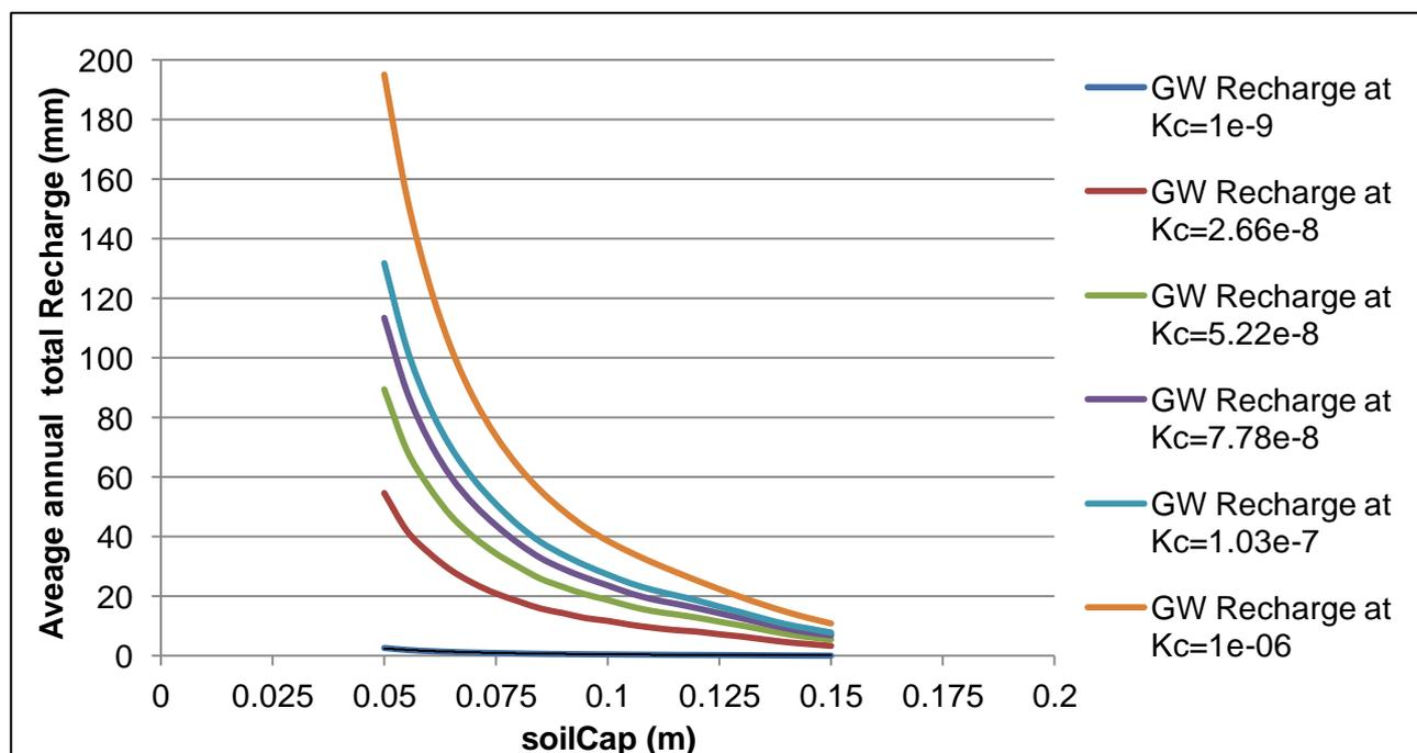
Figure 5.8 Sensitivity of groundwater recharge to soilCap
