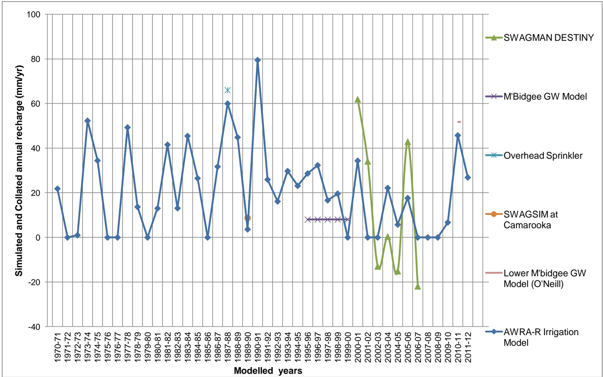
Figure 5.7 Simulated groundwater recharge estimates fitted with existing data
