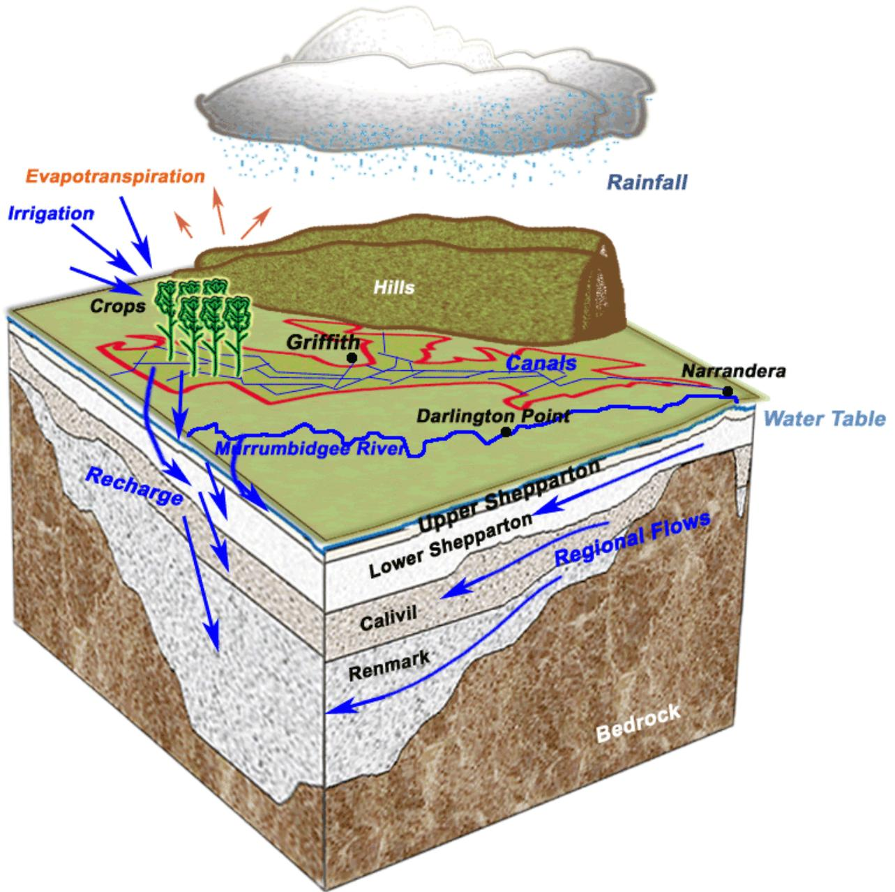
Figure 3.6 Schematic of the MIA hydrogeological systems (Khan et al. 2004)
