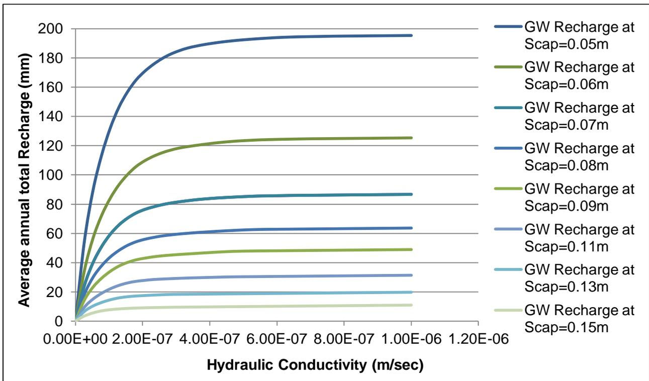
**Figure 5.9 Sensitivity of groundwater recharge to hydraulic conductivity**
