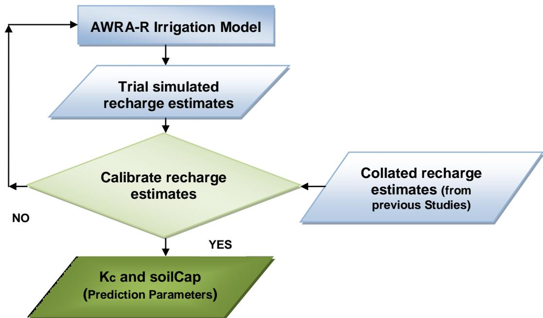
**Figure 4.3 Flow chart for calibration of recharge estimates**
