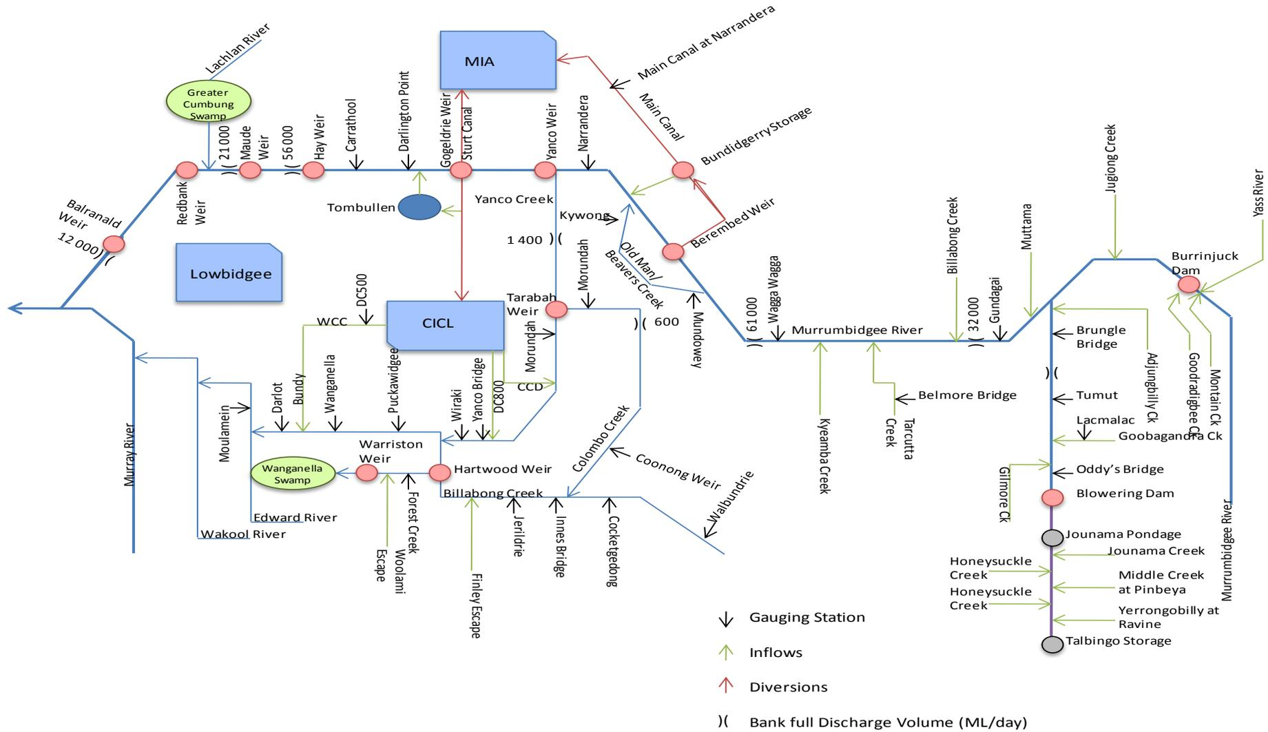
Figure D.1 Schematic showing distribution of Water resources in the Murrumbidgee Catchment (Sinclair Knight Merz 2011)
