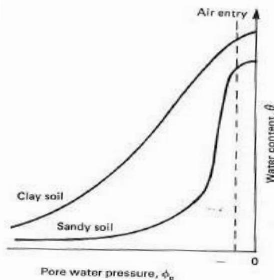
**Figure 2.6 Soil-Moisture retention curves for different soils (Hillel 1980)**
