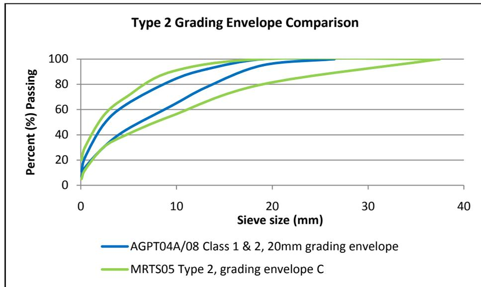
**Figure 2-1** AGPT04A/08 and MRTS05 Type 2 grading envelope comparison.
