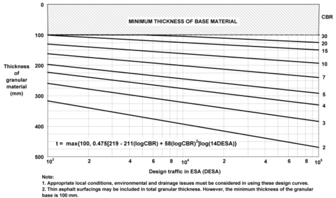
**Figure 12.2: Example design chart for lightly-trafficked granular pavements with thin bituminous surfacings**
