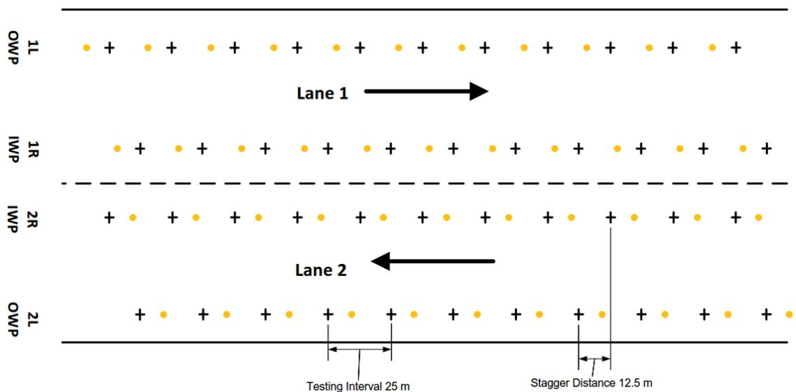
**Figure 4-1** Typical FWD staggered testing layout.
