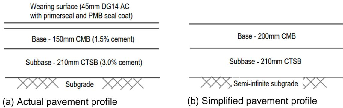
**Figure 4-7** Typical pavement profile simplification for CIRCLY design analysis
