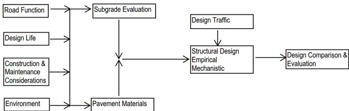
**Figure 2-3** Pavement design process (Austroads, AGPT02/12)
