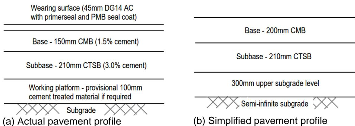
**Figure 4-2** Typical pavement profile simplification adopted for back-analysis.
