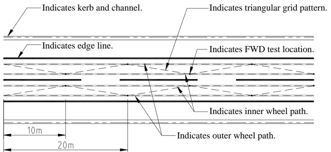
**Figure 3-6** FWD proposed testing layout
