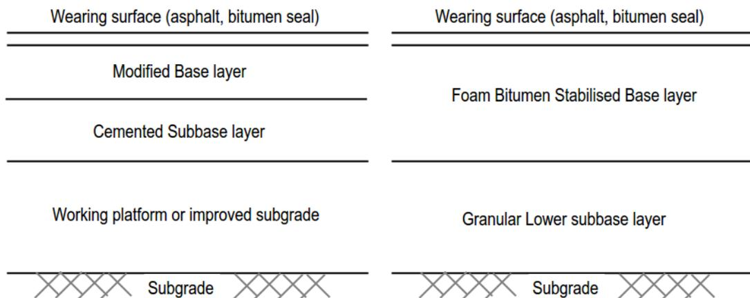
**Figure 2-4** Example pavement structures
