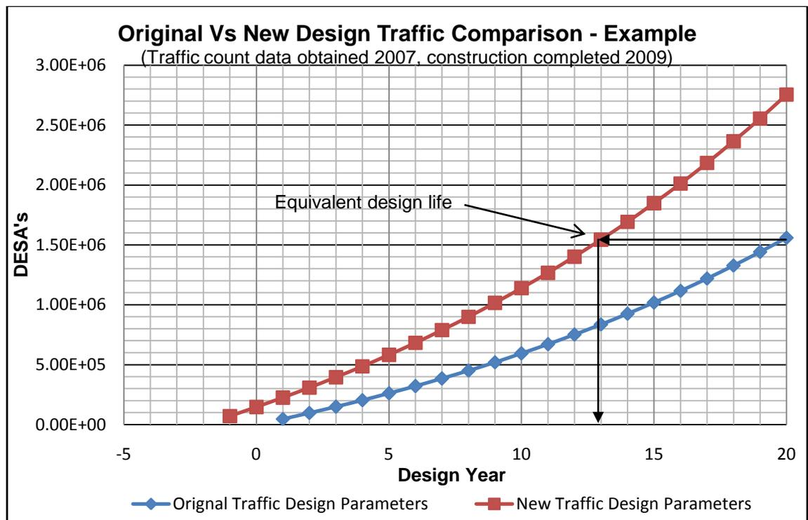
**Figure 4-8** Example of the effect of modified traffic design parameters
