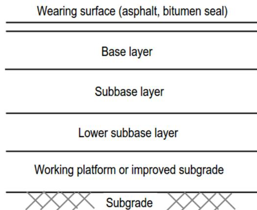
**Figure 2-2** A typical pavement profile.
