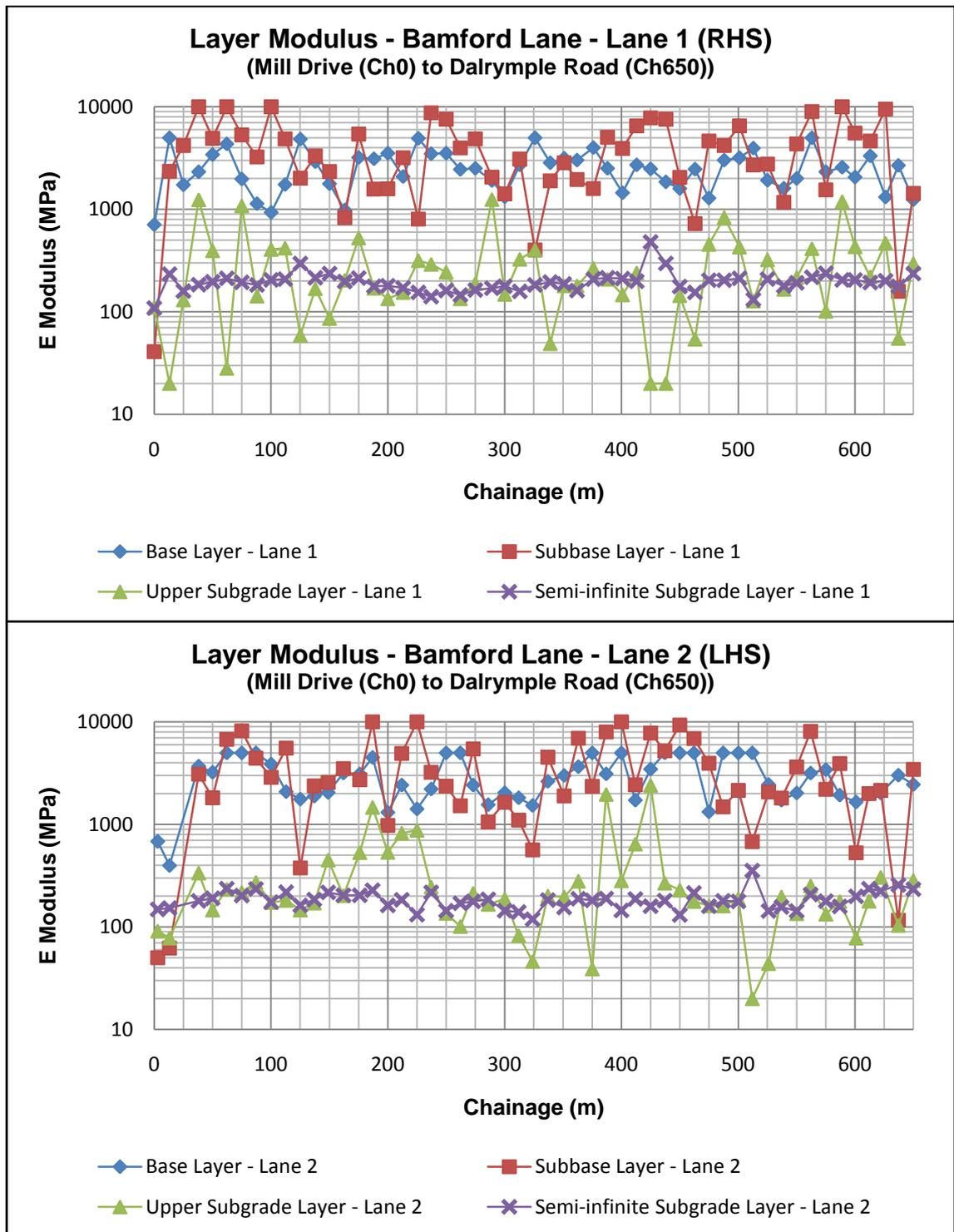
Figure 4-5 Bamford Lane layer modulus
