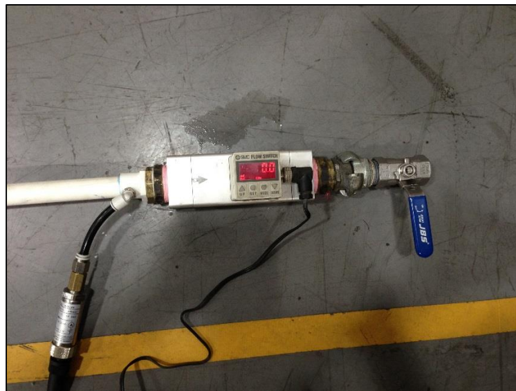
Figure 3-5 Leaf Blower Test - Flow Meter, Pressure Sensor and Ball Valve
