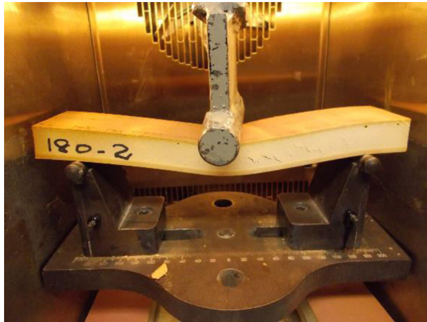
Figure 4.48 Failure of the specimen at 180°C
