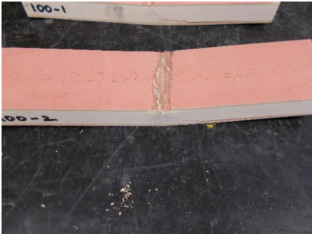
Figure 4.44 Failure mode of the specimen at 100°C
