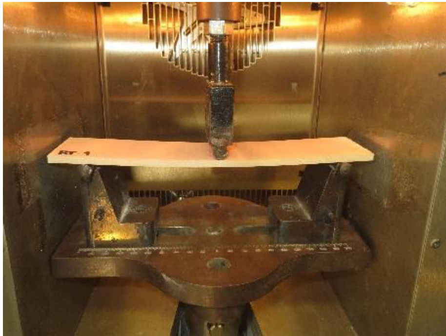
Figure 3.6: Flexure Test Set-Up
