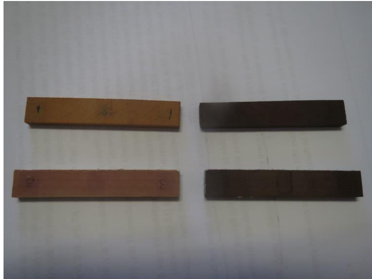
Figure 5.1 Skin Specimens before and after DMA
