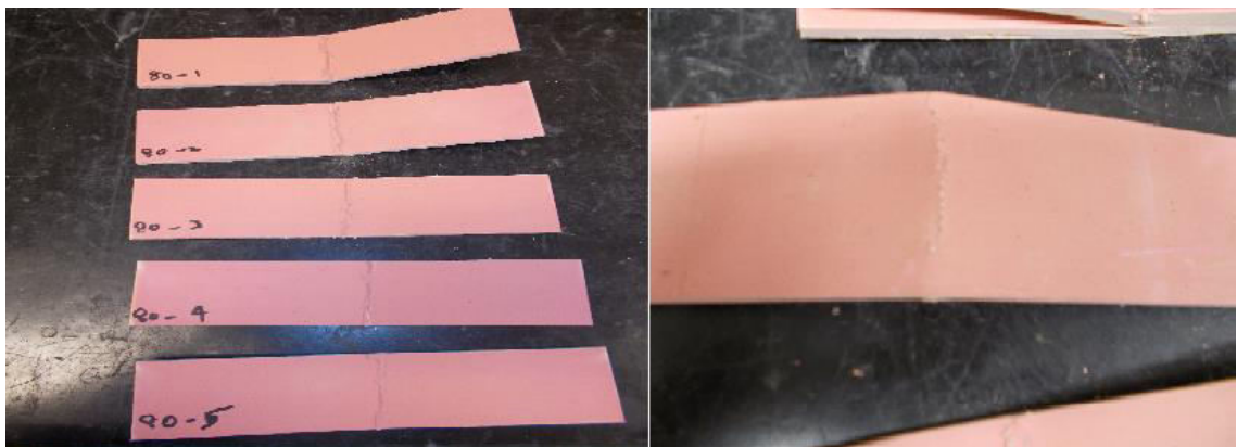
Figure 4.21 Compression and Tension cracks on the specimen at 80°C
