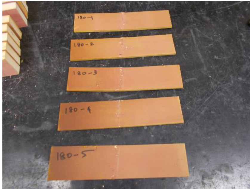
Figure 4.28 Failure on the compression side of the specimen at 180°C
