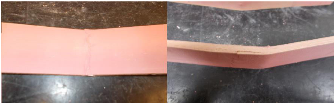
Figure 4.25 Compression and Tension cracks on the specimen at 120°C
