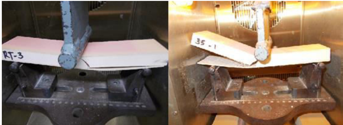
Figure 4.38 Failure modes at 21°C and 35°C
