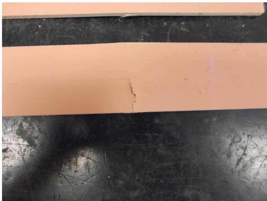
Figure 4.15 Cracks on the tension side of the skin at 35°C
