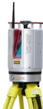
Figure 3. The Riegl VZ-400 – a waveform processing scanner. (Reigl 2014).
