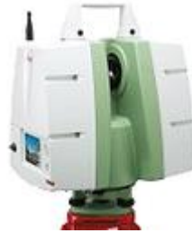
Figure 1. The Leica Scanstation c10 – a time-of-flight scanner. (Leica 2010).
