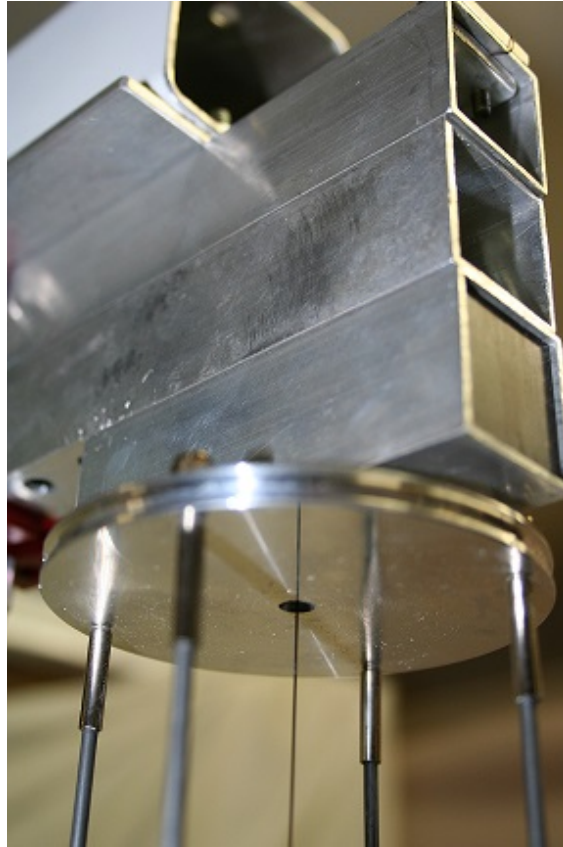
Figure 5.5: Drive Unit Engagement fingers and Guide wire, Ian Saxby 2014
