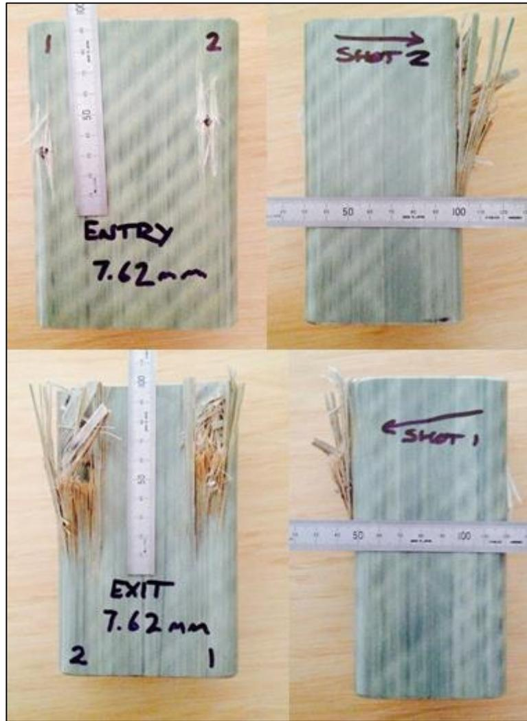
Figure 108. Resultant ballistic damage (external).
