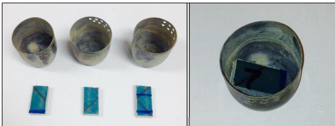
Figure 63. D-spar calcination samples and crucibles.
