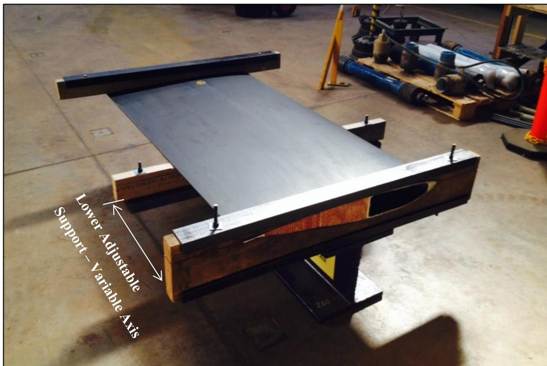
Figure 45. Lower adjustable support axis.
