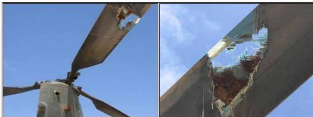
Figure 22. RPG damage to a CH-47 aft rotor blade.
