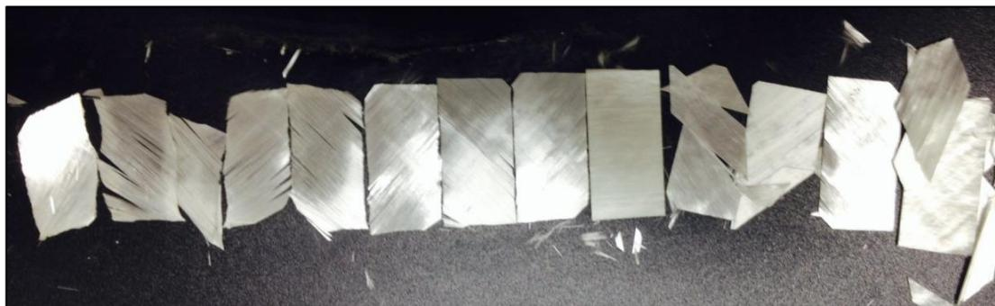
Figure 68. D-spar plies post separation demonstrating fragility.
