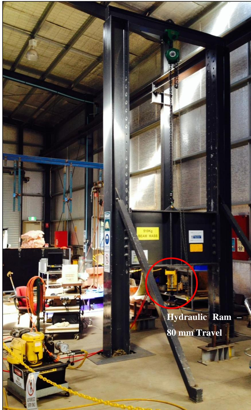
Figure 36. CEEFC 200 Tonne hydraulic test press (USQ CEEFC 2014).
