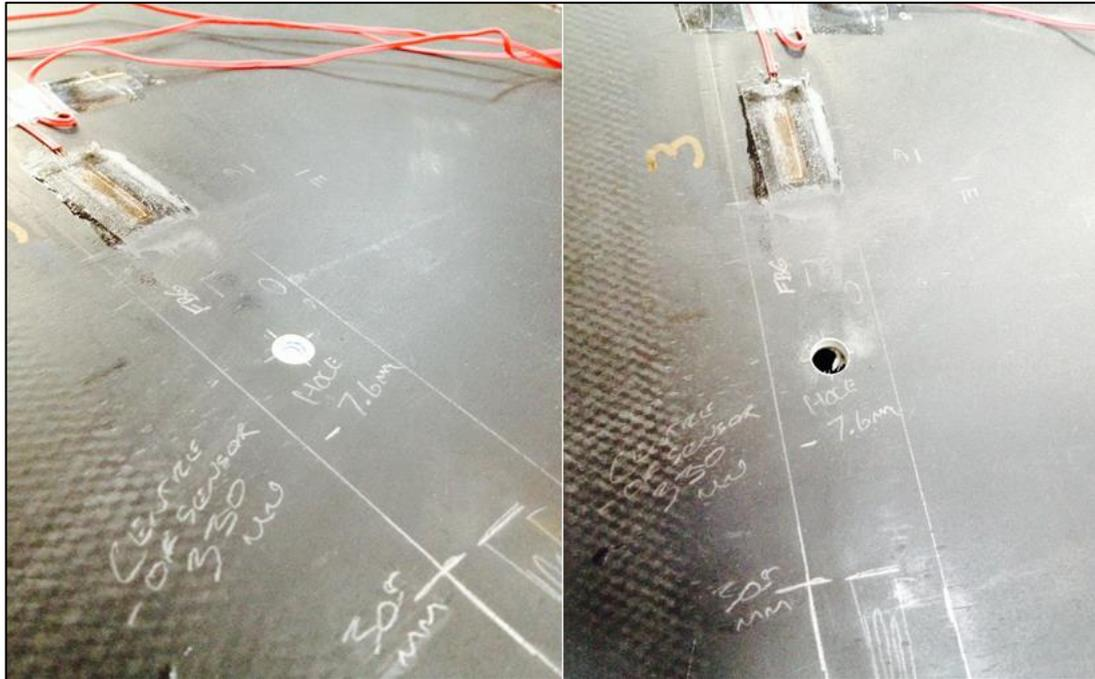
Figure 113. Hole 1 at 3.0 mm depth and full thickness.
