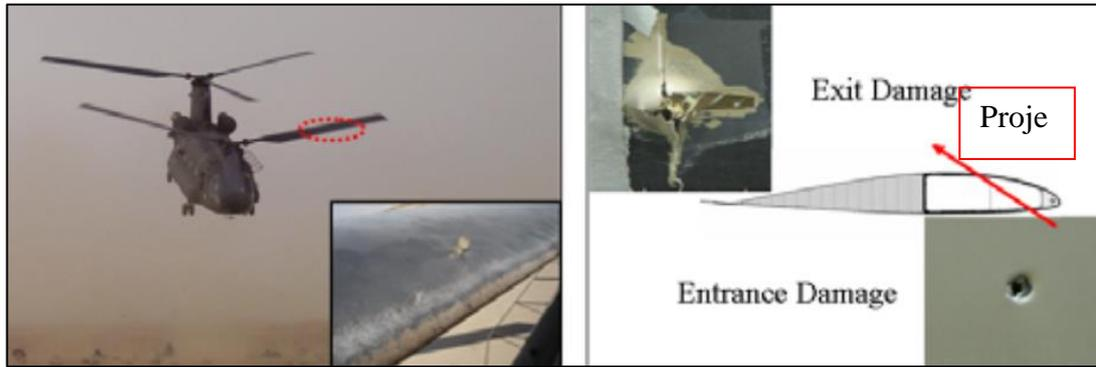
Figure 21. Typical battle damage due to small arm fire (Cline C et al. 2011).
