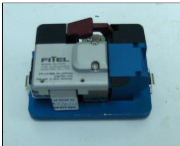
Figure 90. The Vitel high precision fibre cleaver.
