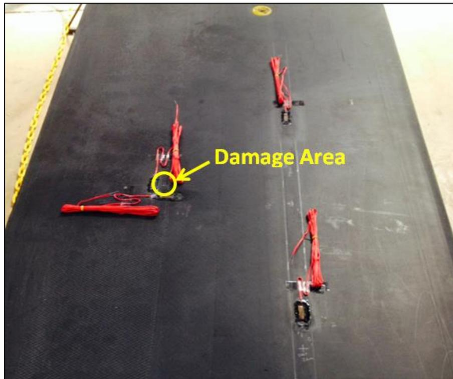
Figure 106. Impact damage location with strain gauges.
