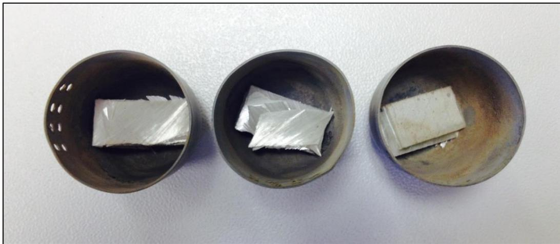
Figure 66. Three D-spar samples post calcination.
