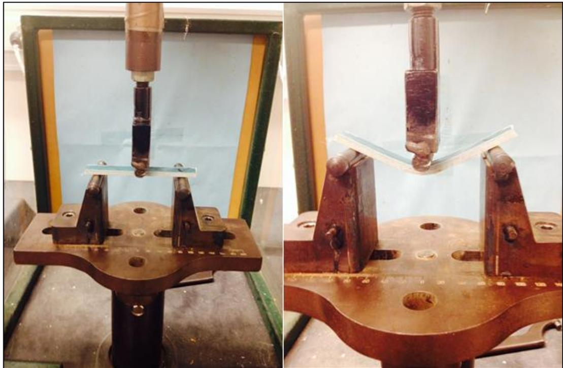
Figure 54. Flexural test close up view.
