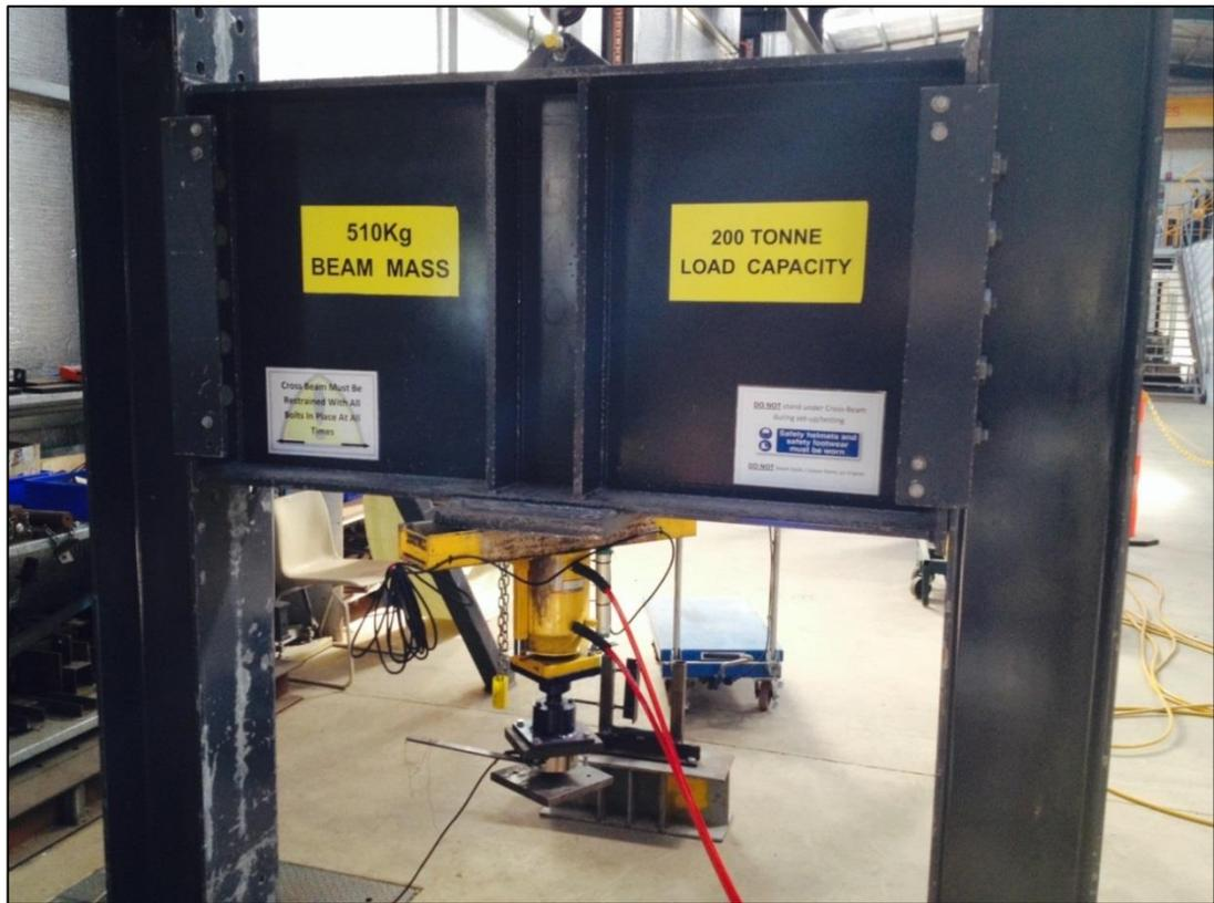
Figure 37. Hydraulic press cross beam (USQ CEEFC 2014).
