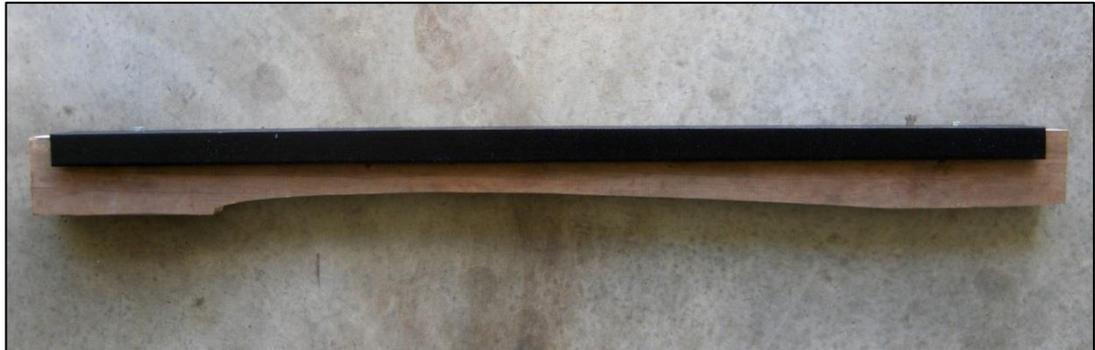
Figure 41. The upper load plate.
