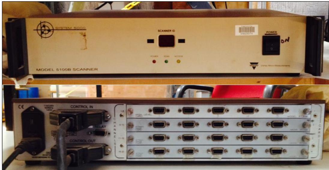
Figure 100. StrainSmart System 5000 (5100B) data acquisition system.
