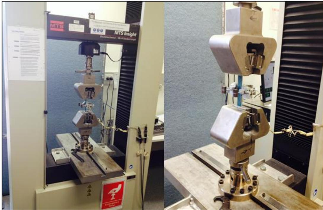
Figure 60. MTS Insight tensile testing machine.
