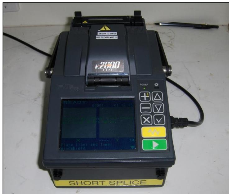
Figure 91. The Vitel v. 2000 s175 fusion splicing machine.
