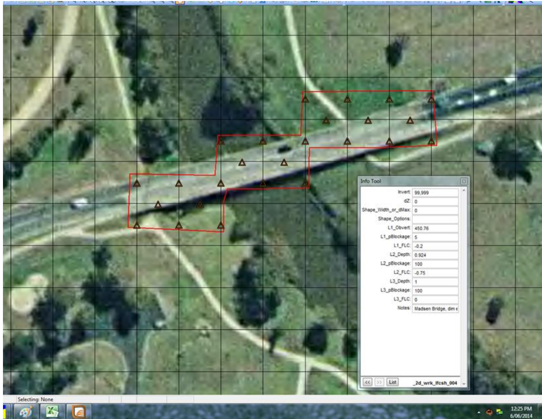
Figure 2.6 - O.O. Madsen Bridge flow constriction in TUFLOW
