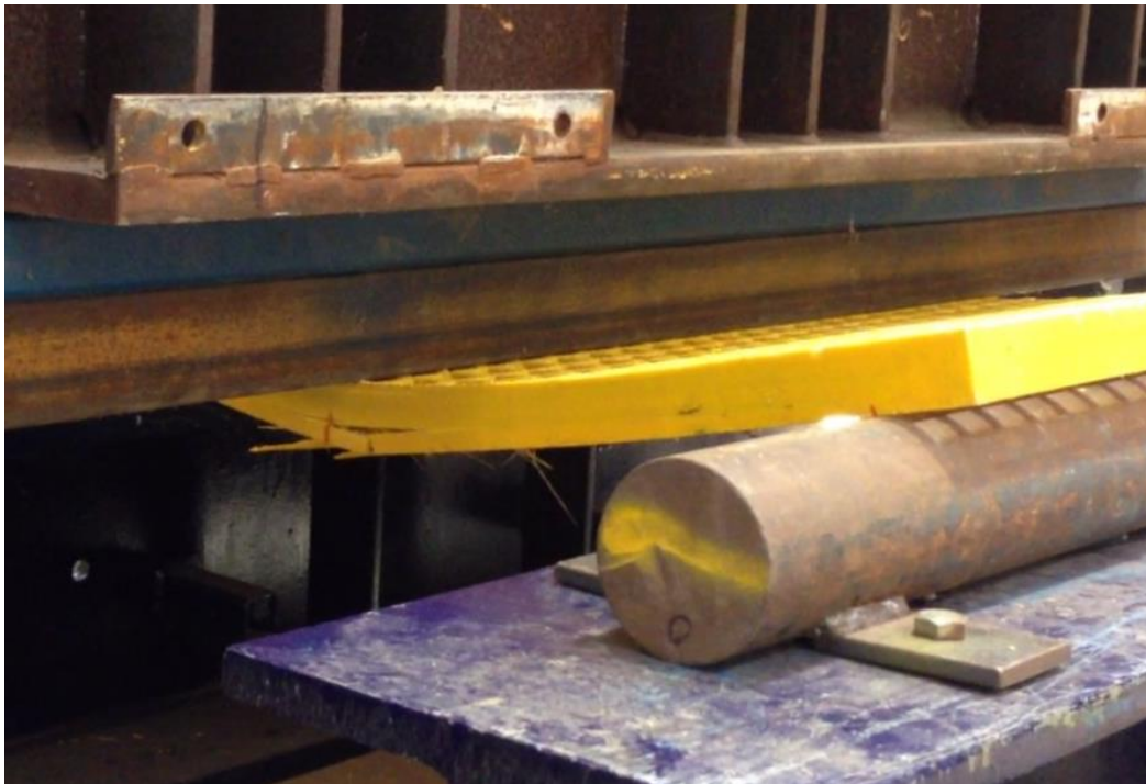
Figure 23 - Failure of line loading test panel (Nicol, Lachlan. 2014)
