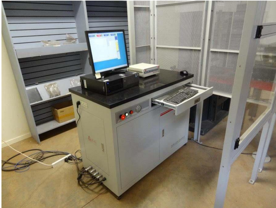
Figure 16 - Computer used to record compressive testing data (Nicol, Lachlan. 2014)
