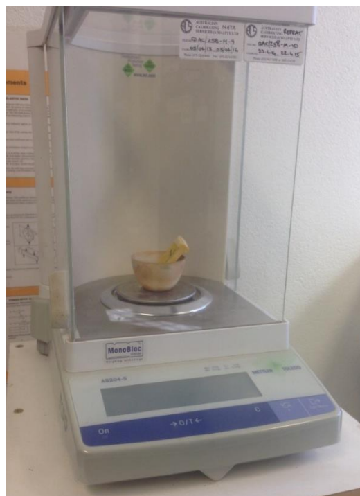
Figure 17 - Weighing of the crucible and the grid sample (Nicol, Lachlan. 2014)
