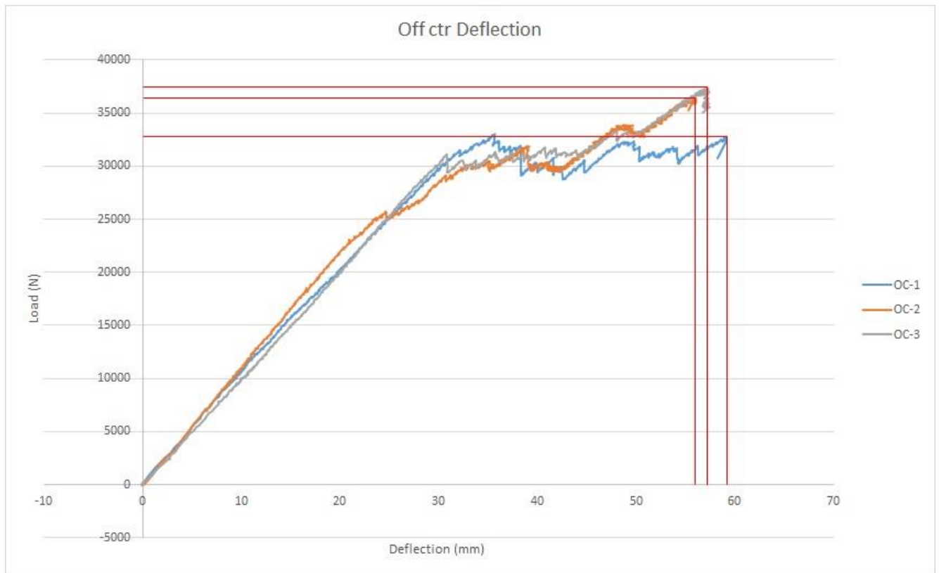
Figure 26 - Deflection results for off centre concentrated load
