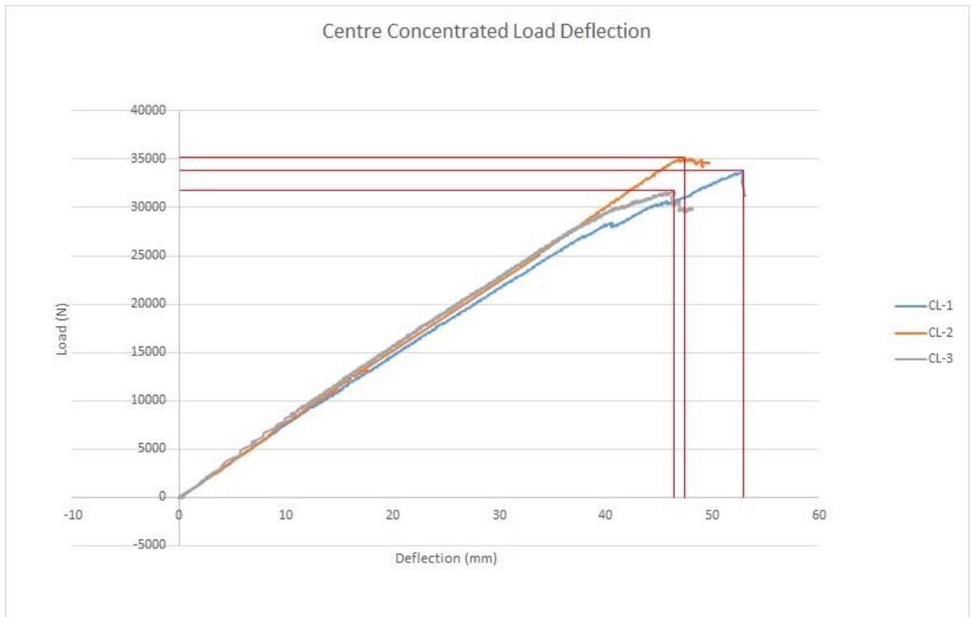
Figure 24 - Deflection results for centred concentrated loading
