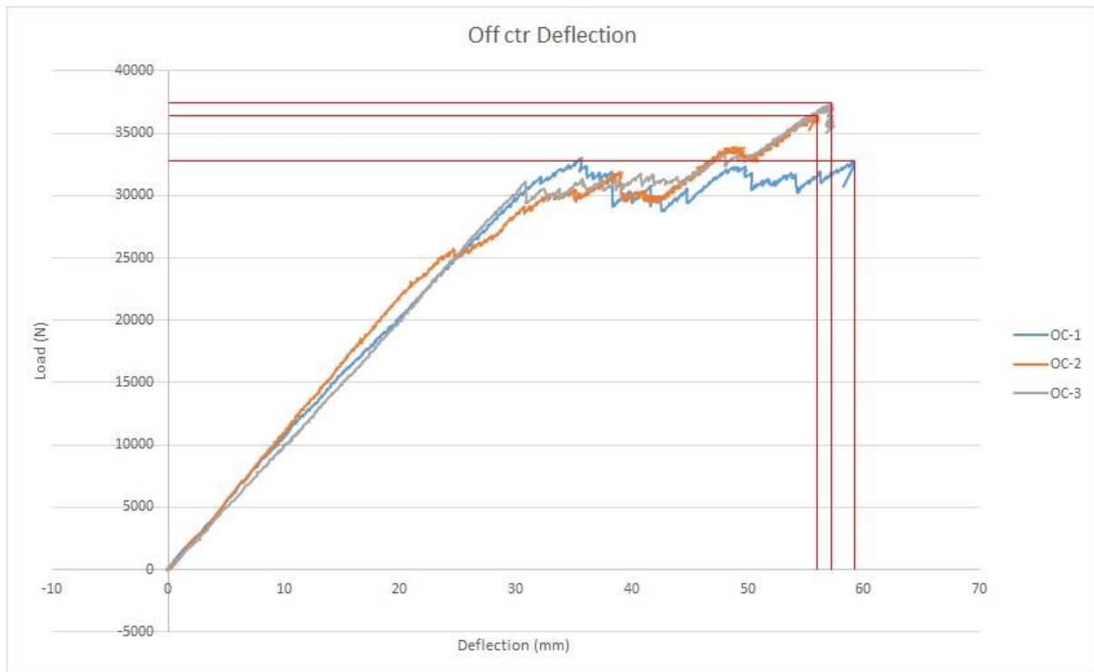
Off centre concentrated load deflection results (3 records)
