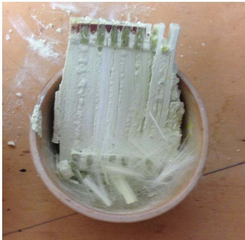
Figure 33 - Burnt out FRP web containing 'filler material' and glass fibres (Nicol, Lachlan. 2014)
