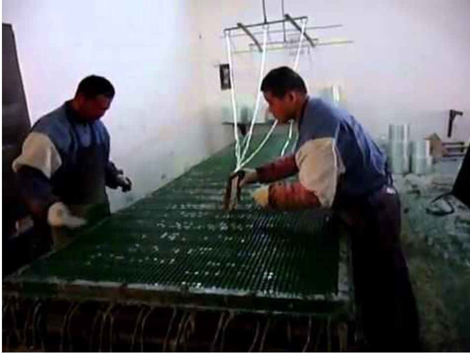
Figure 5 - Moulded FRP grid manufacturing process (ZarnitsaTeam, 2011)
