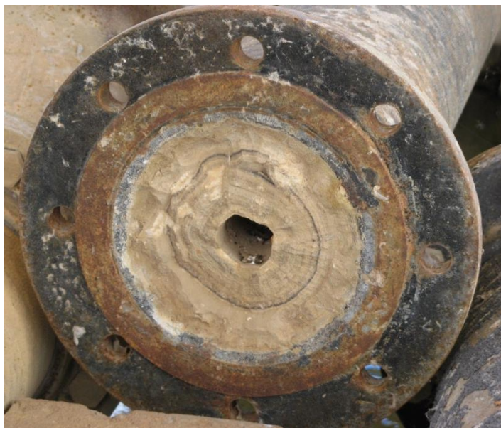
Figure 7.3. Mineral build-up on the inside of a pipe at Winton (Ryan, I 2014, supplied photograph, 25 March)
