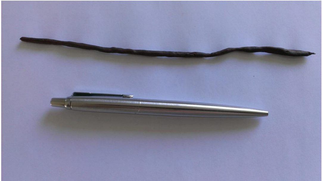
Figure 5.7. Soil sample rolled into a fine thread
