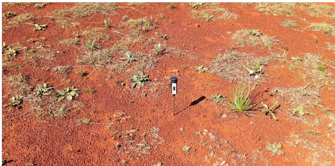
Figure 5.13. Soil surface temperature measurement on a bare earth area
