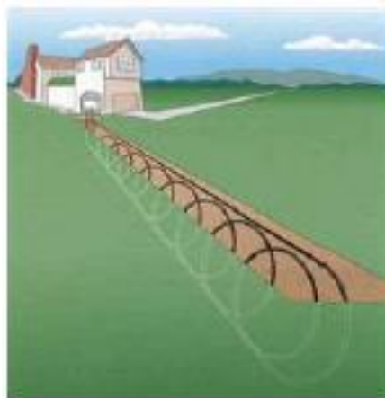
Figure 2.5. Horizontal expanded coil pipe loop system (Klaassen 2006)
