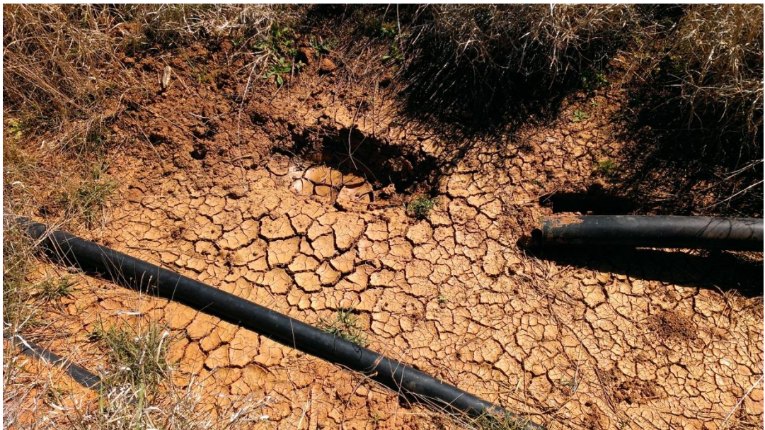
Figure 5.8. "Cracking clay" behaviour exhibited on-site
