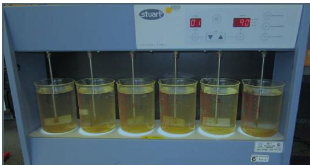
Figure 3.1- Jar testing apparatus (Manthey, 2014)
