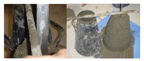
Figure 5.5 - Slump Test
