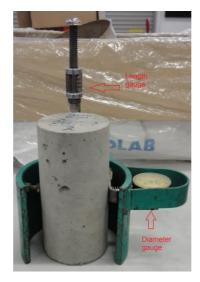
Figure 5.8-Cylinder diamensions measurement
