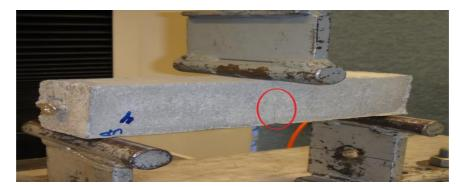
Figure 5.16- Flexural strength test on standard sample
