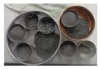
Figure 2.3 – Aggregate size
