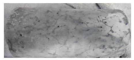
Figure 5.12- Mapping crack at 77 days
