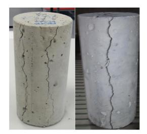
Figure 5.10 – Cracked sample after load was applied
