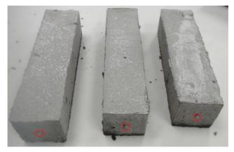
Figure 3.4 – Mortar bars with stainless steel screw as studs
