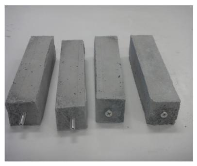
Figure 3.7 – Second batch ASTM C1260 testing
