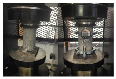
Figure 5.14 - Compressive Strength Test
