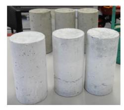
Figure 5.7 -Cylinders ready for tensile strength testing
