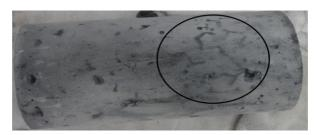
Figure 5.11- Beginning of mapping crack at 49 days
