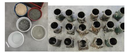
Figure 5.2 - Aggregates and moulds
