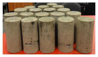
Figure 5.6 - Specimen after takign out of the mould
