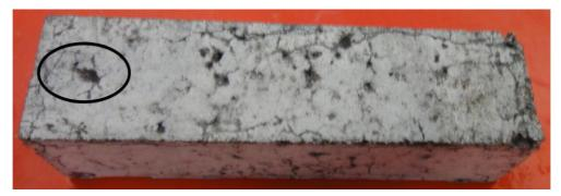
Figure 5.13 - Cracks forming from voids
