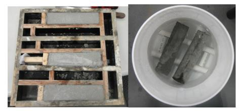
Figure 3.3 - Samples in the mould and later placed in NaOH solution
