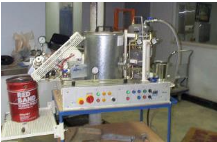
Figure 3-3: WLB10 Laboratory scale foamed bitumen machine (Kendall et al. 2001)
