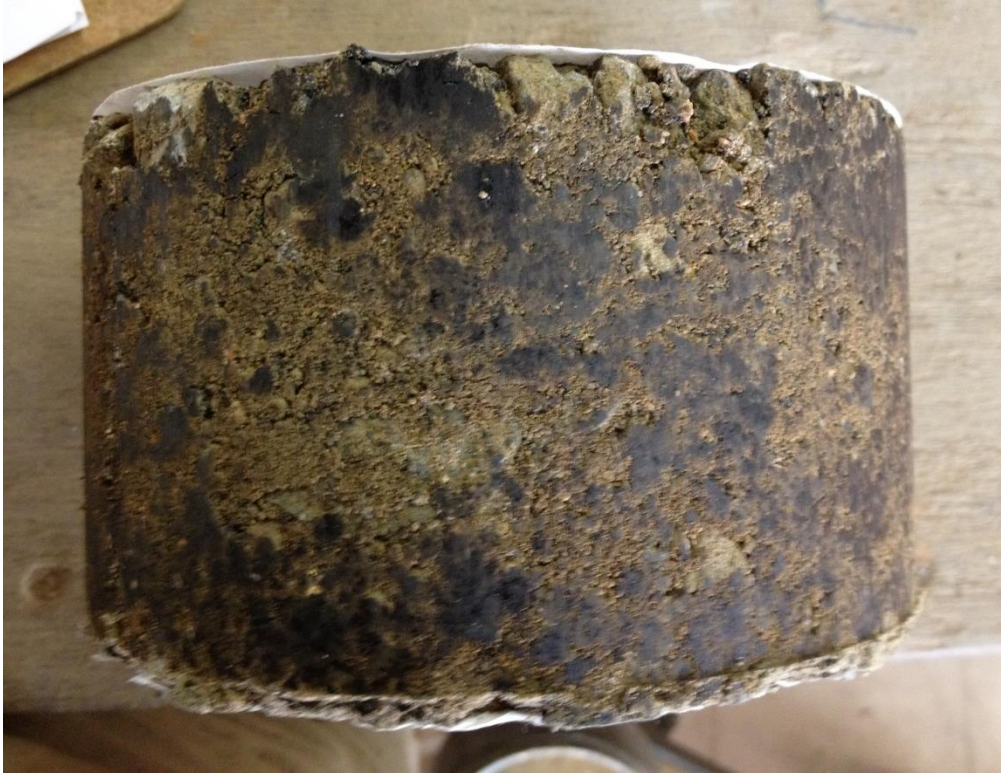
Figure 3-5: Foamed bitumen briquette
