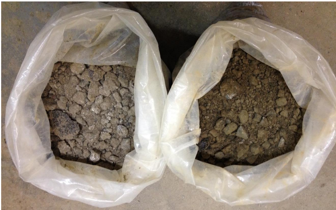
Figure 3-4: Roadbase material before (left) and after (right) addition of foamed bitumen.
