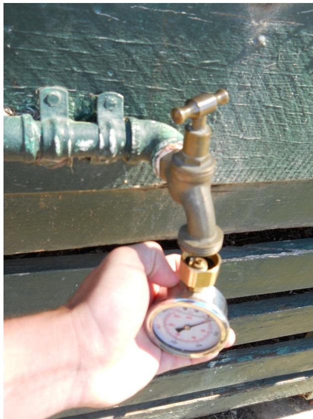
Figure 3.35: 32mm tap - Too large for pressure gauge connection.
