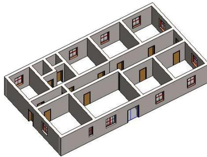
Figure 6- Manual Survey BIM of Strathneath Homestead
