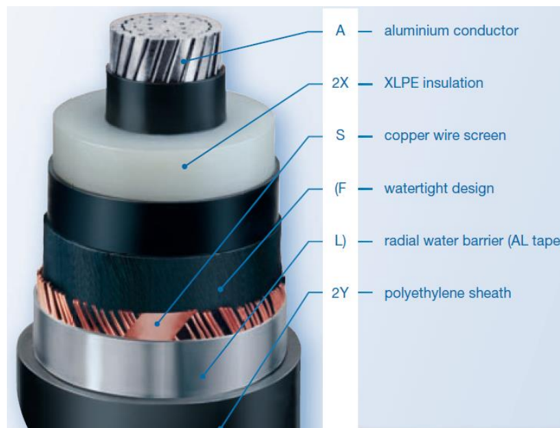
Figure 2.5 – Single Core XLPE Cable (NKT cables, 2009)
