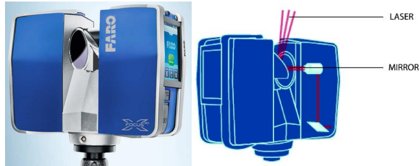
Figure 2.9 The Faro Focus 3DX330 and laser deflection (source Faro )
