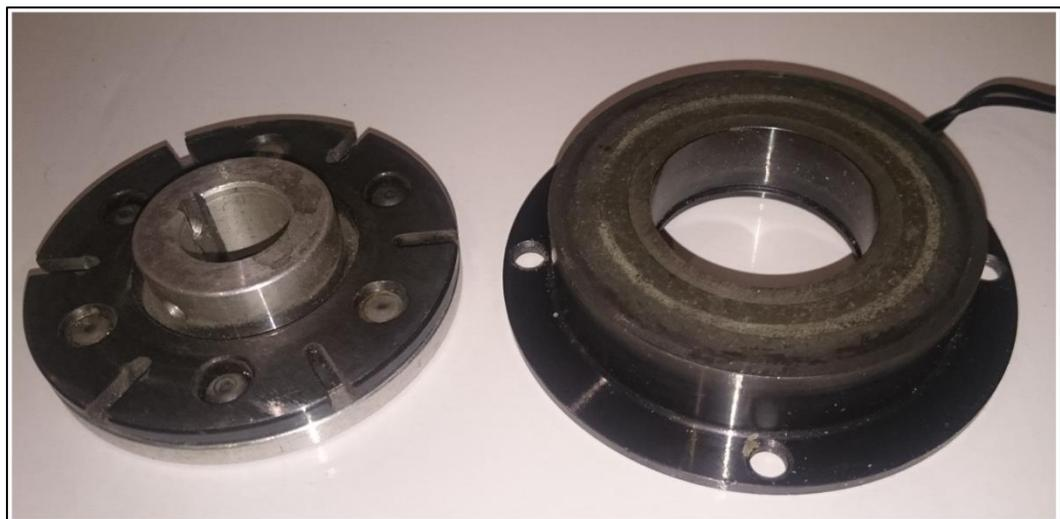
Figure 5-15: Electromagnetic Brake Pictured Apart
