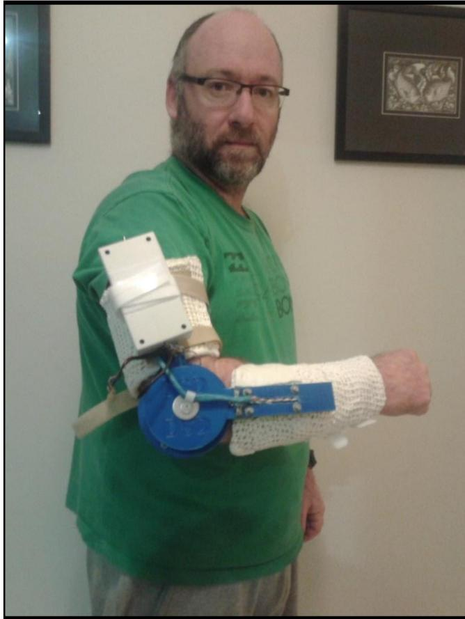
**Figure 6-50: DSD with Electronic Box Secured with Velcro**
