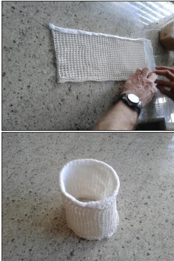
**Figure 6-48: Splint Material before and after Forming**
