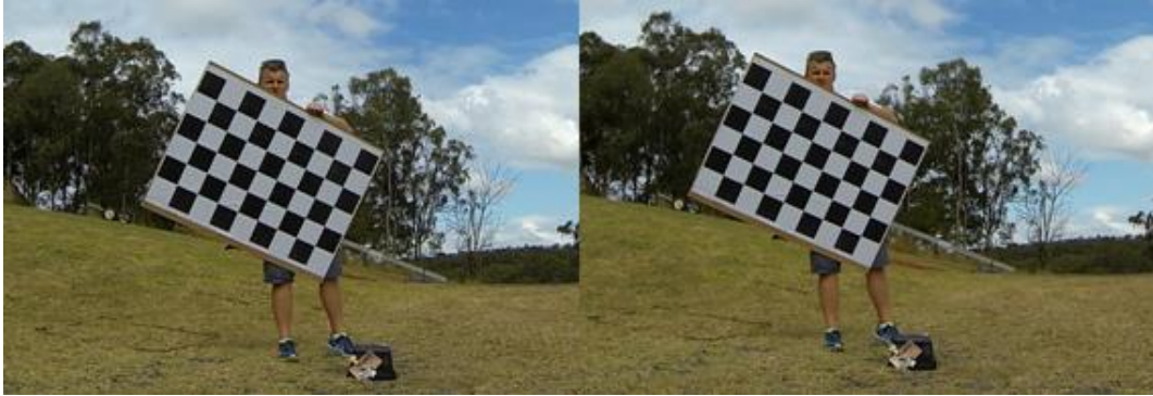
Figure 4.6 Sample of calibration images from dynamic trials
