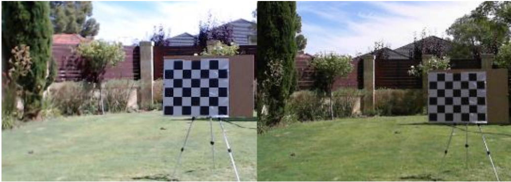
Figure 4.1 Comparison between Logitech C920(left) and Microsoft LifeCam Studio(right) images.
