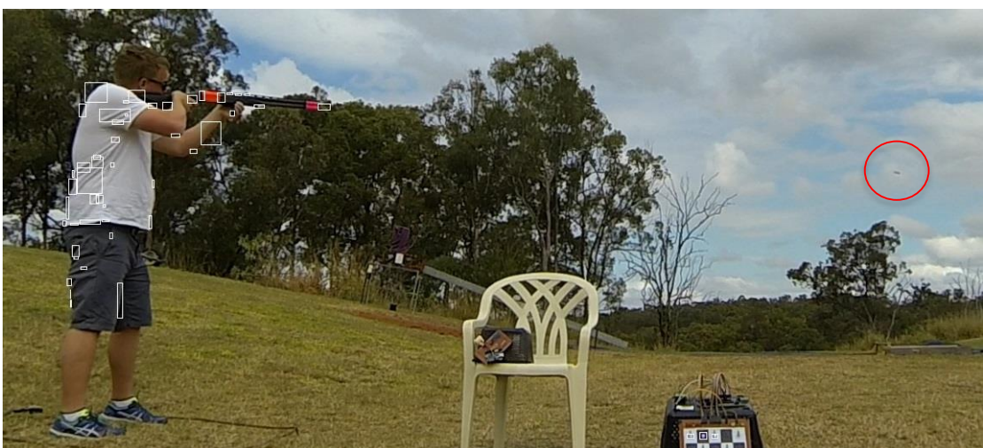
Figure 6.4 Frame 5 of the test images with bounding boxes around areas that were segmented as foreground. The red circle shows the target location.
