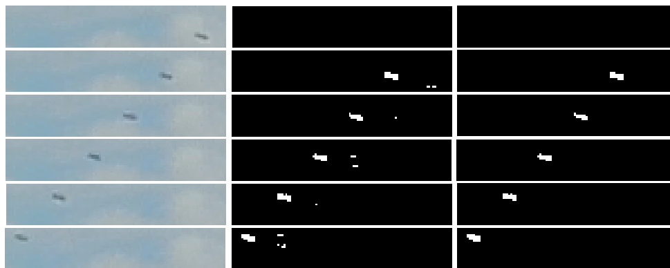
Figure 6.6 The stages the image sequences go through as part of GetTargetLoc.m. From left to right – original pixels, subtracted and thresholded pixels, pixels after noise filtering.
