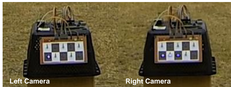
Figure 6.7 Camera synchronization test circuit set to illuminate 10 LEDs in 1/60 s showing the left camera leads the right in this trial by 0.2 frames.
