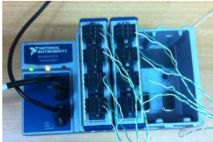
Figure 25 - NI cDAQ-9174 Used for Thermocouple Interrogation
