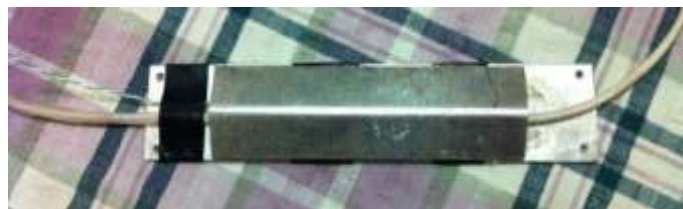
Figure 36 - Aluminium Encasing of FBG Sensor
