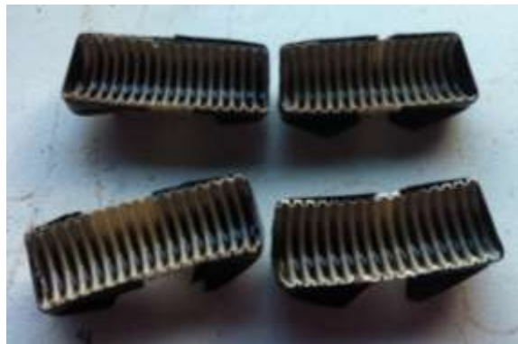
Figure 49 – Modified Concrete Capsule Moulds
