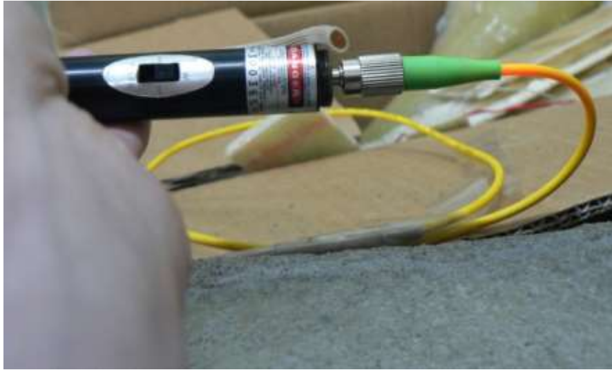
Figure 52 - Replica Fibre Shown to Survive Pouring and Compaction
