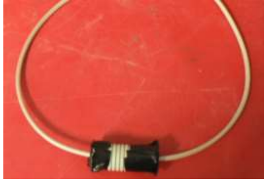
Figure 35 - Method of Encasing FBG Sensor in Concrete Capsule Moulds
