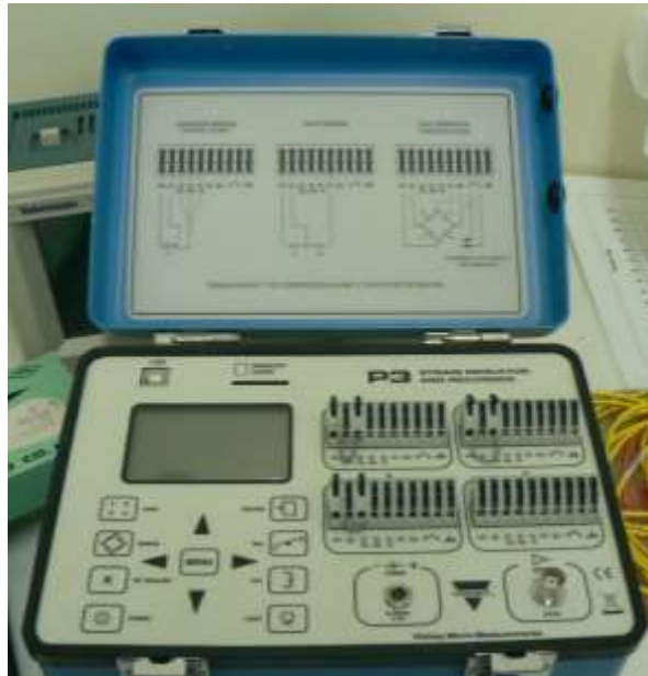
Figure 28 - Strain Gauge Interrogator Unit
