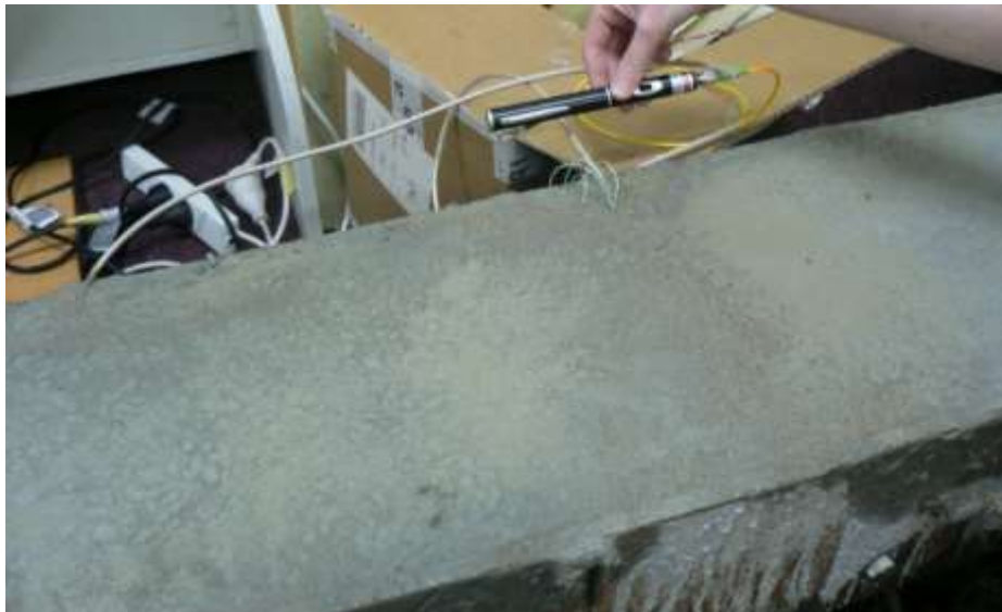
Figure 53 - Proof Replica Fibre is embedded in Concrete Beam
