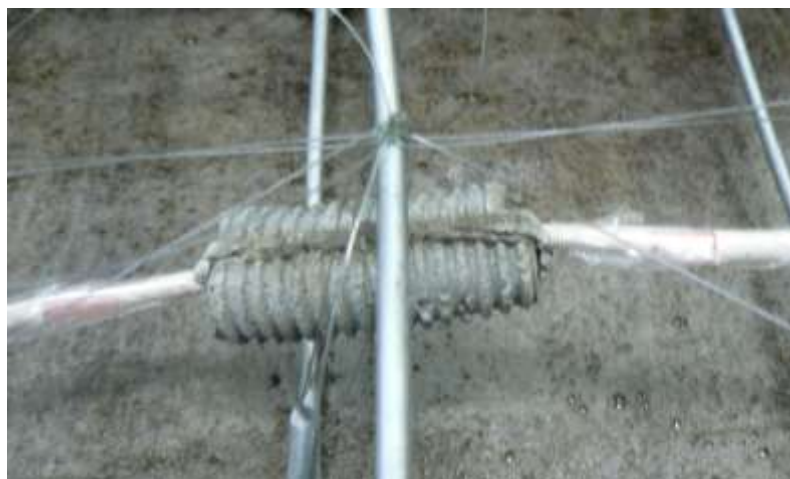
Figure 51 - Replica Fibre Tied in Position Using Fishing Line
