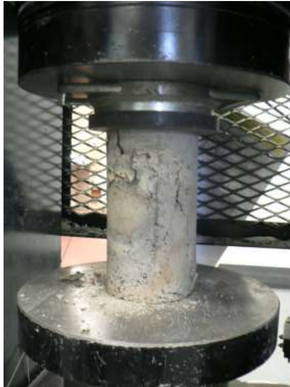
Figure 67 - Concrete Cylinder under Compression Tests at Failure Load
