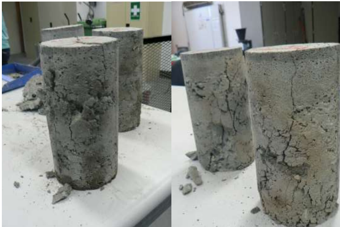
Figure 68 - Failure Planes of Control and Heated Concrete Cylinders
