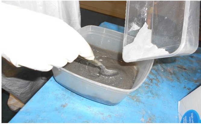
Figure 3.7 - Adding the fillers to the resins and combining well.
