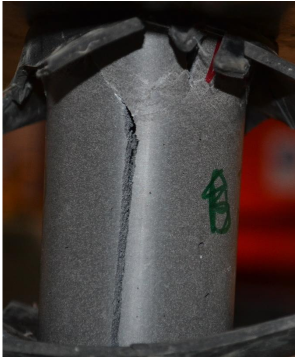
Figure 5.5 - Possible splitting failure of specimen for mix design 1:1.2:0
