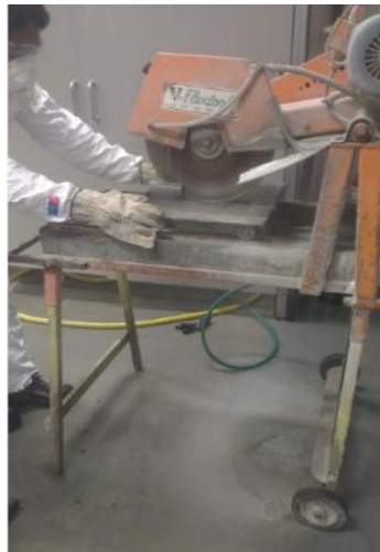
Figure 3.9 - Wet Saw in Z1.101 used to cut the samples.
