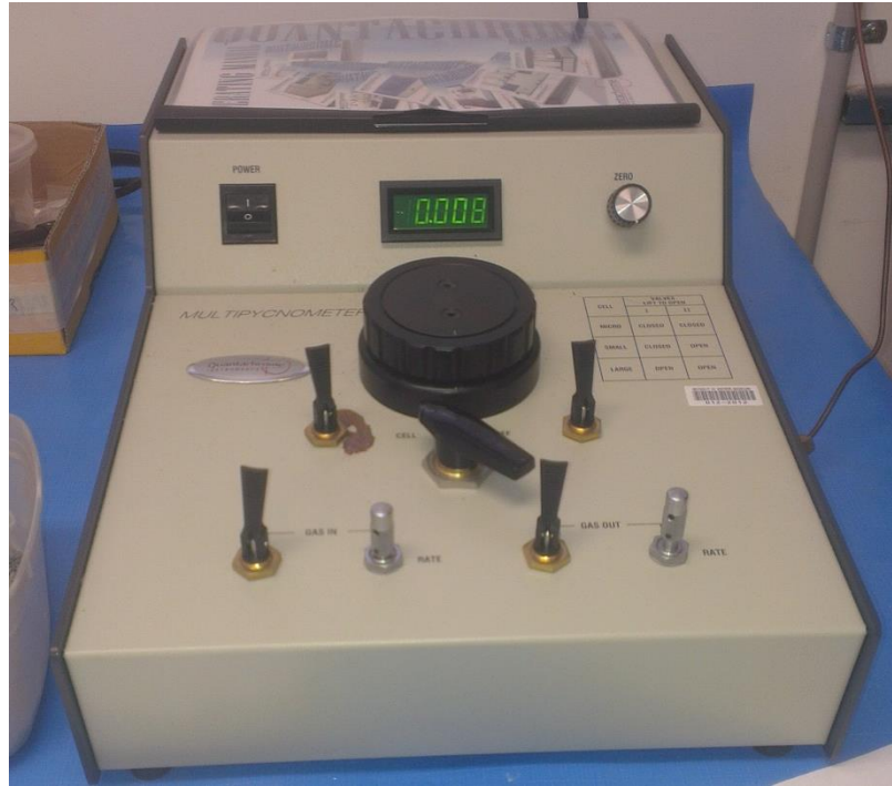
Figure 3.4 - Multipycnometer used to measure the density of the aggregate.
