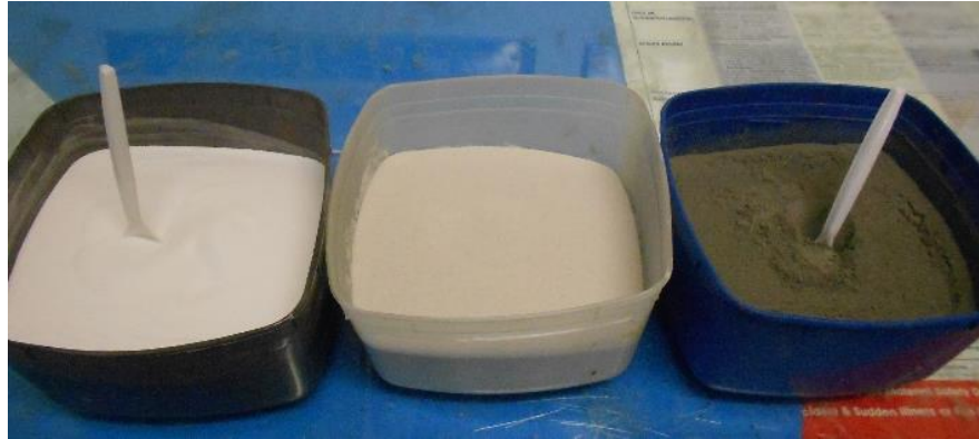
Figure 3.3 - Fillers used in the mix; (right to left) Hollow Microsphere Filler, Fire Retardant Filler and Fly Ash
