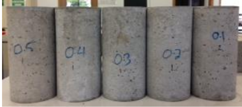
Figure 6.1: Compressive specimens at varied dosages (0.5% - 0.00115% fibre dosage left to right)
