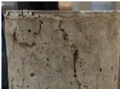
Figure 6.8: Thinner cement mortar top capping
