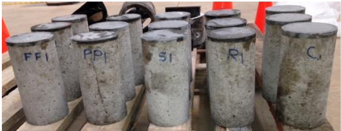
Figure 5.1: Compressive specimens (Forta Ferro, polypropylene, steel, ReoShore 45 and control left to right)
