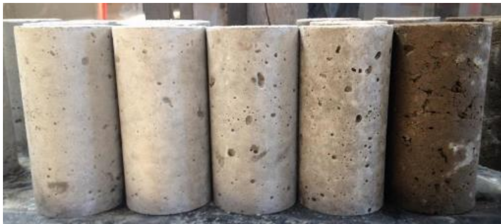
Figure 4.1: Compression specimens (1%, 2%, 6%, 10%, 20% oil contamination left to right)
