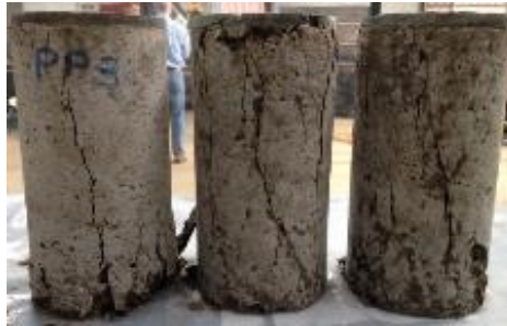
Figure 5.8: Shear failure of polypropylene fibre-reinforced specimens
