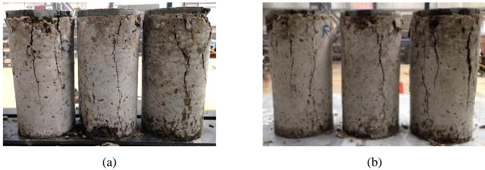
Figure 5.7: Splitting failure of control (a) and ReoShore 45 fibre-reinforced (b) specimens
