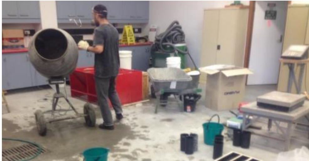
Figure 3.10: Mixing concrete batches
