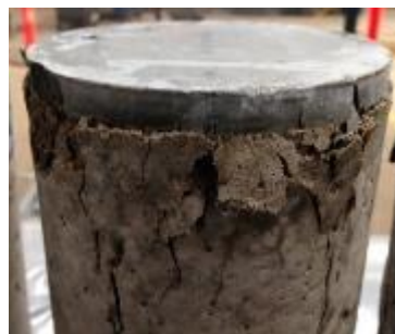
Figure 5.10: Cement mortar capping causing crushing
