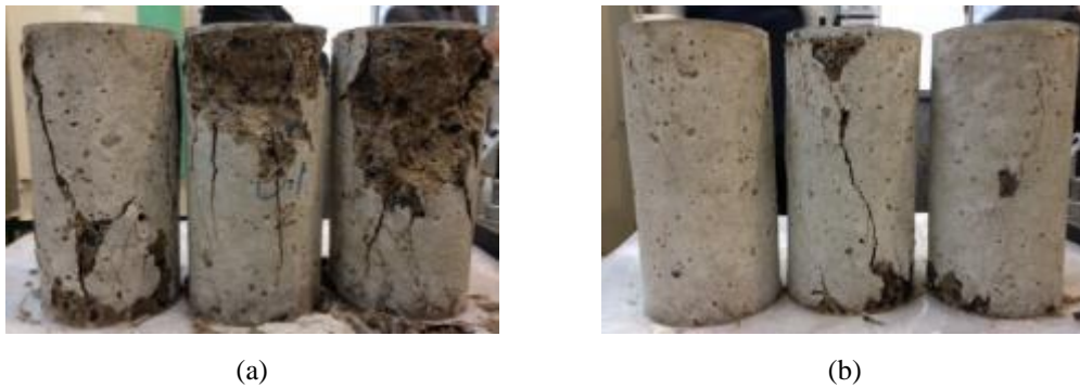
Figure 6.7: Splitting/conical failure of 0.00115% (a) and splitting/shear failure of 0.5% (b) SFRC specimens
