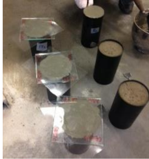
Figure 3.12: Cement paste application
