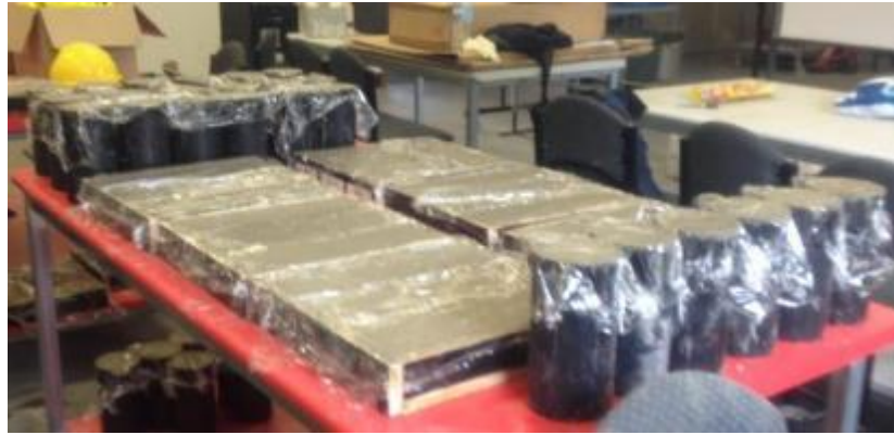
Figure 3.13: Specimens before mould removal
