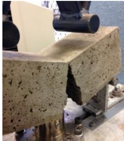
Figure 5.17: Control flexural failure behaviour
