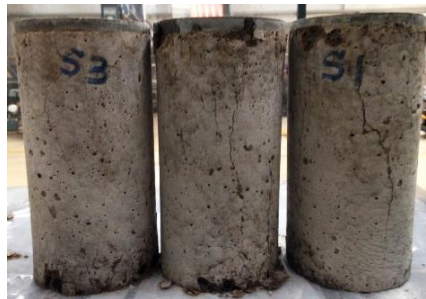
Figure 5.9: Decreased cracking of steel fibre-reinforced specimens
