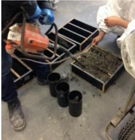
Figure 3.11: Use of immersion vibrator
