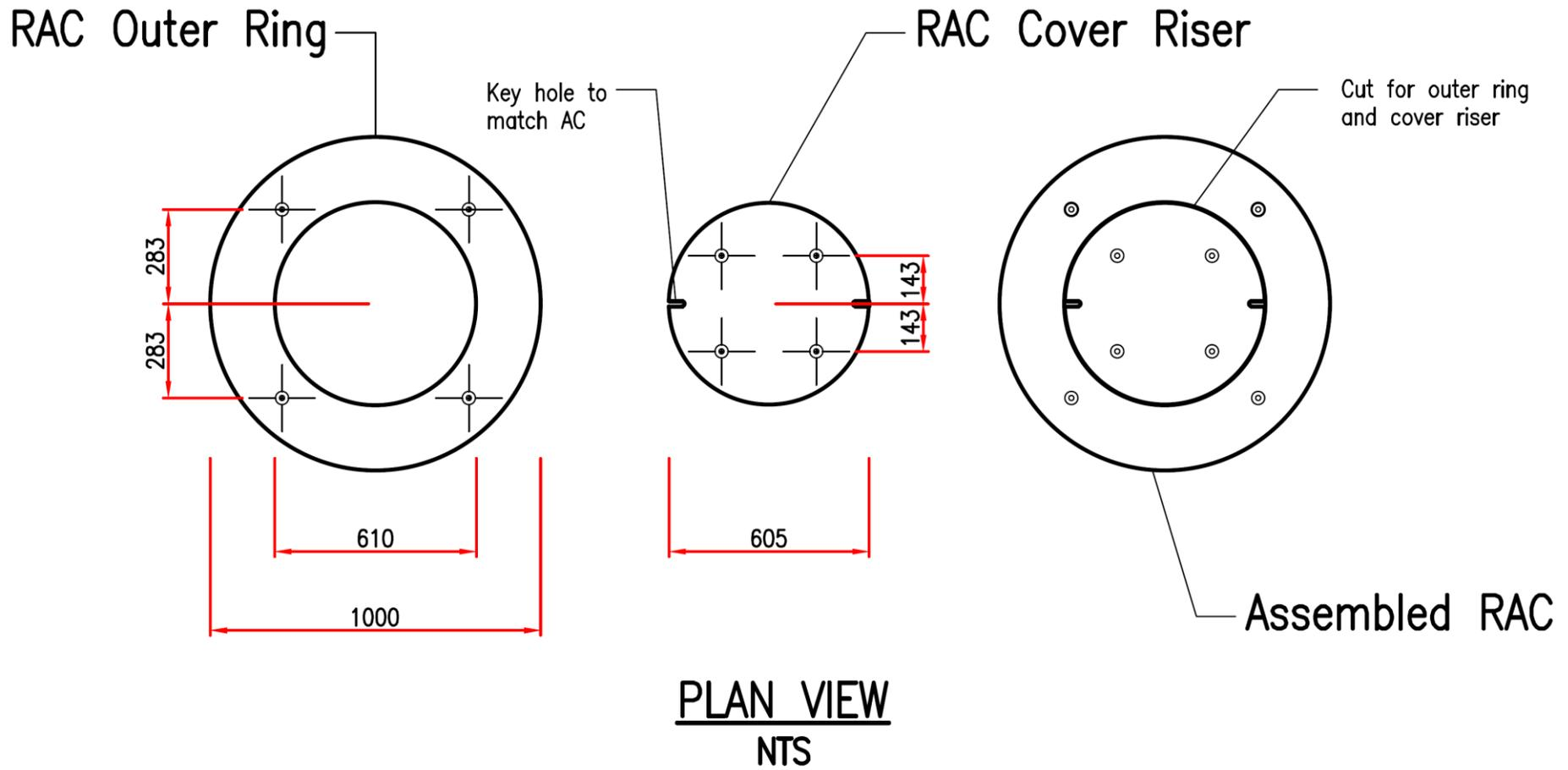
Figure 4.17(a): RAC detailed design drawing.
