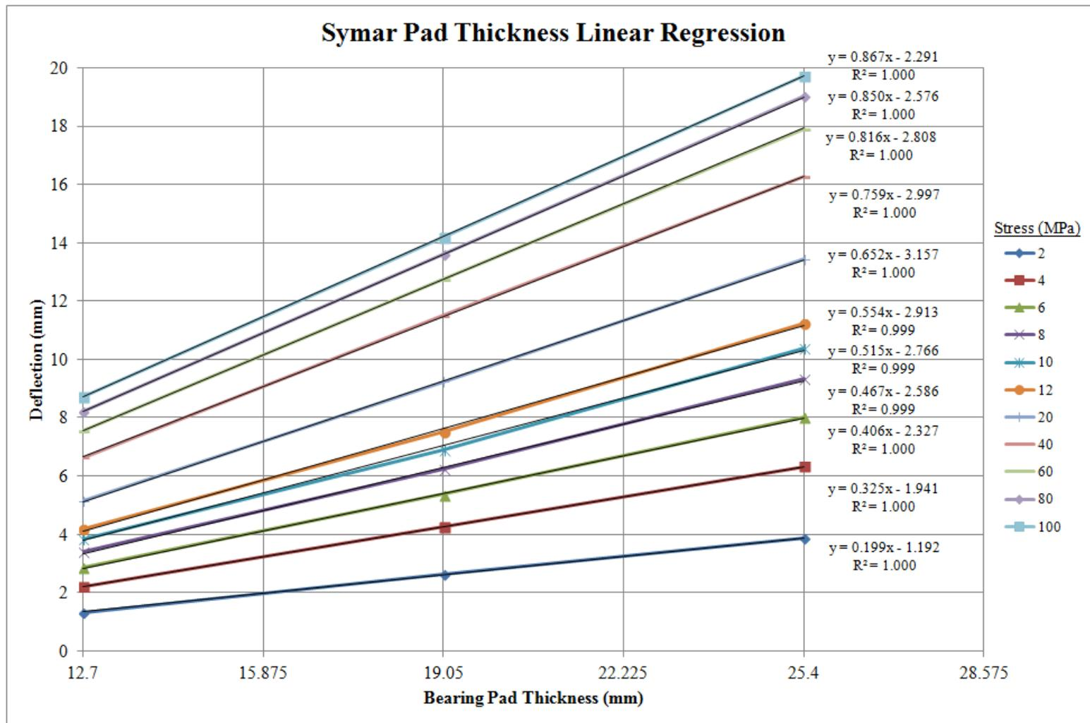
**Figure 4.1:** KN Rubber Symar Bearing Pad linear regression of deflection verse thickness.
