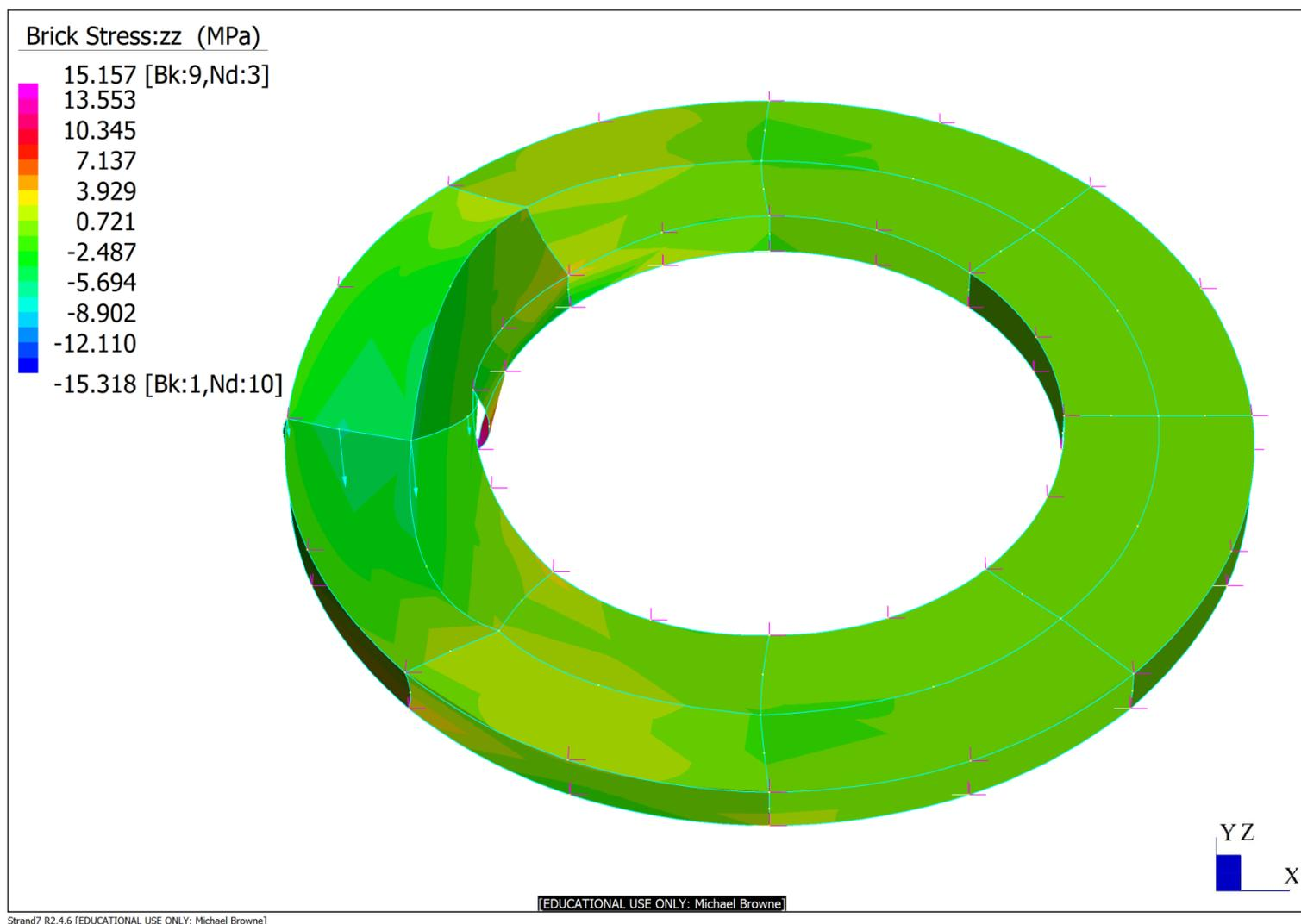
**Figure 4.16:** 50.0 mm RAC load cases 6 stress distribution and deflection scale 5.0 %.
