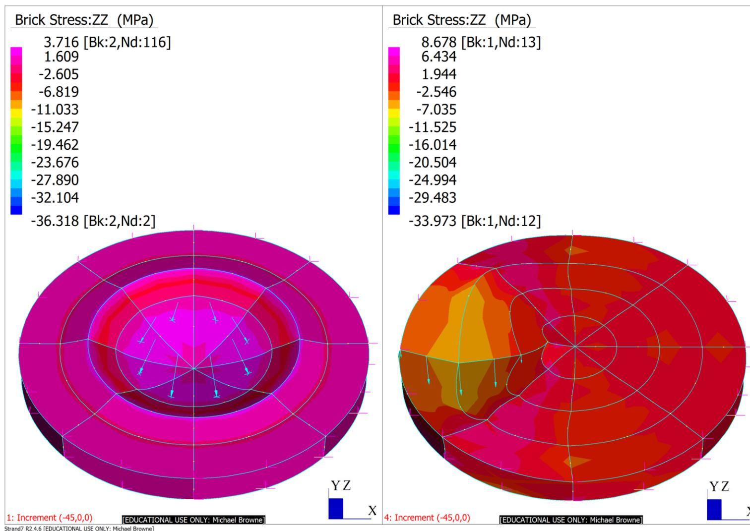
**Figure 4.15:** 50.0 mm RAC load cases 1 (left) and 2 (right) stress distribution and deflection scale 10.0 %.
