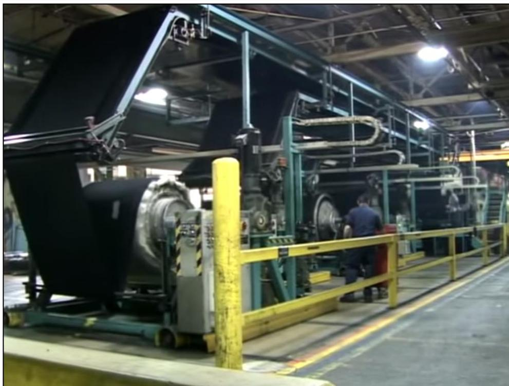
**Figure 3.5:** Curing or vulcanisation of the rubber on a continuous press (KN Rubber LLC 2013).
