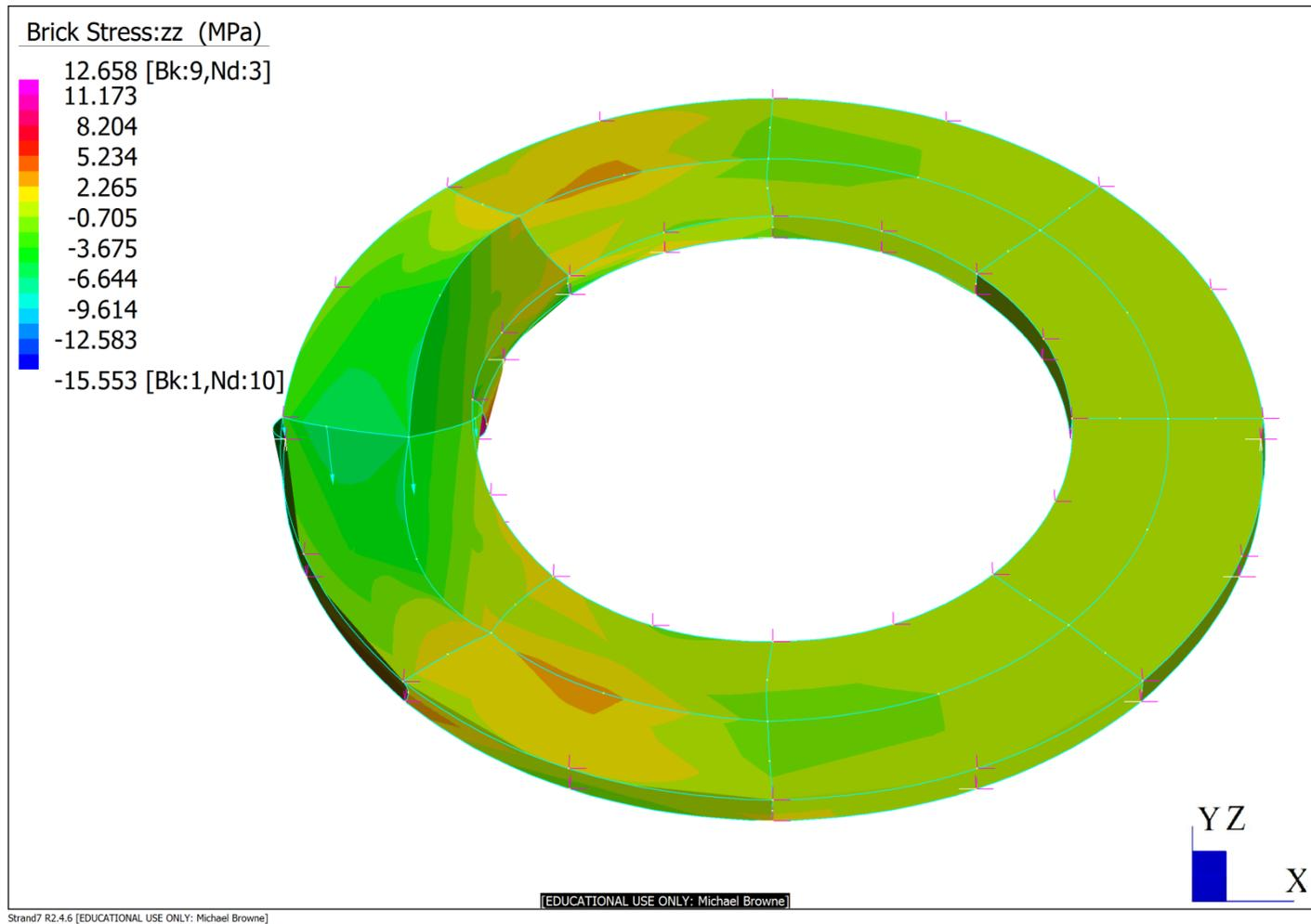
**Figure 4.14:** 30.0 mm RAC load cases 6 stress distribution and deflection scale 5.0 %.
