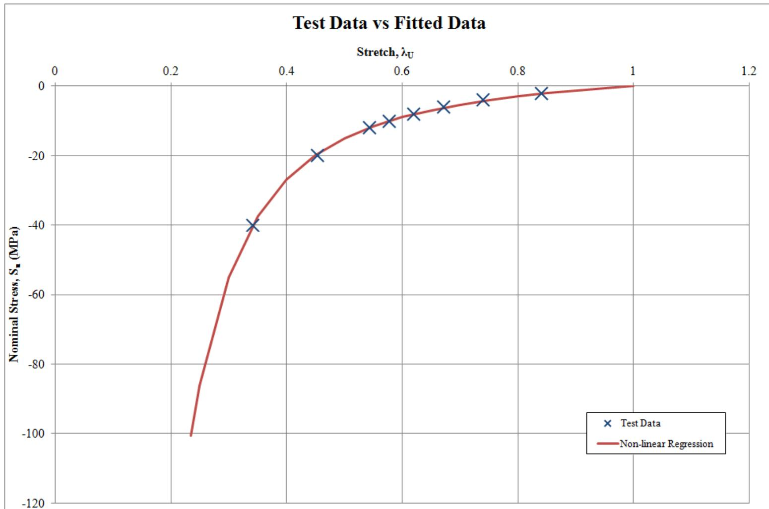
**Figure 4.4:** Comparison of test data with the fitted curve for 50.0 mm specimen.
