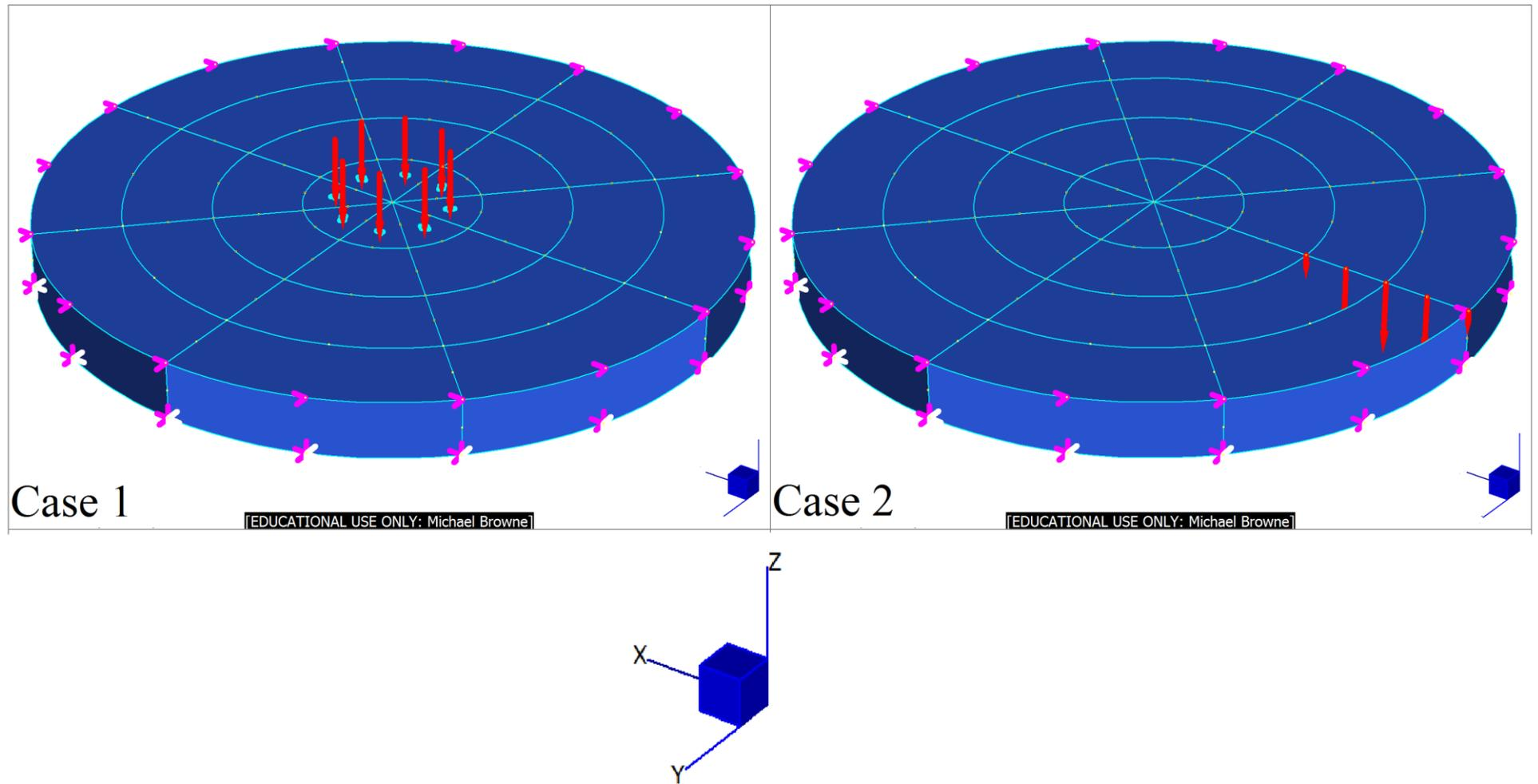
**Figure 4.10:** Load cases 1 and 2, and model restraints for the cover raiser in both 30.0 mm and 50.0 mm thicknesses.
