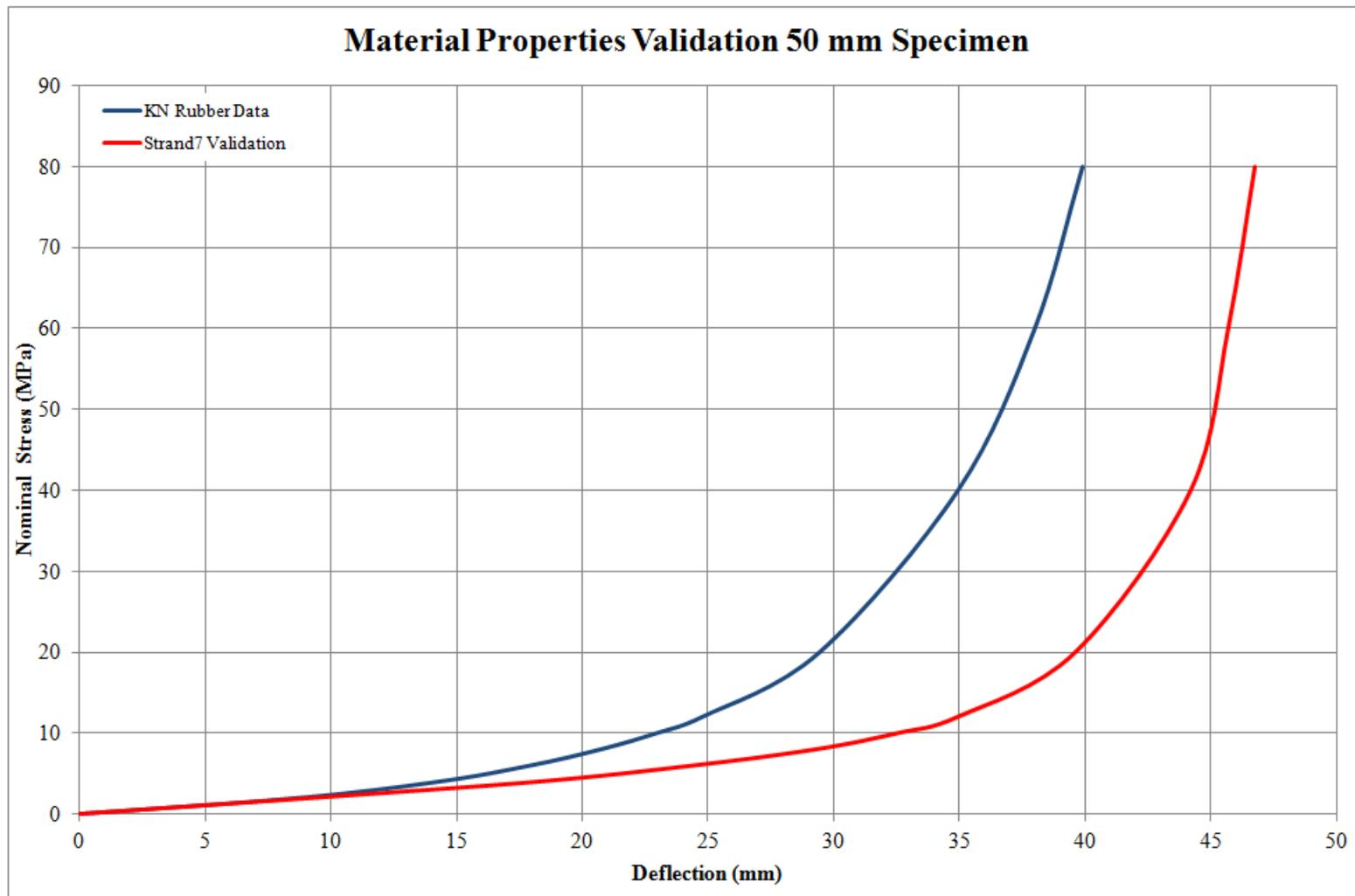
**Figure 4.7:** Material properties validation plot showing KN Rubber extrapolated data and Strand7 results for a 50.0 mm specimen.
