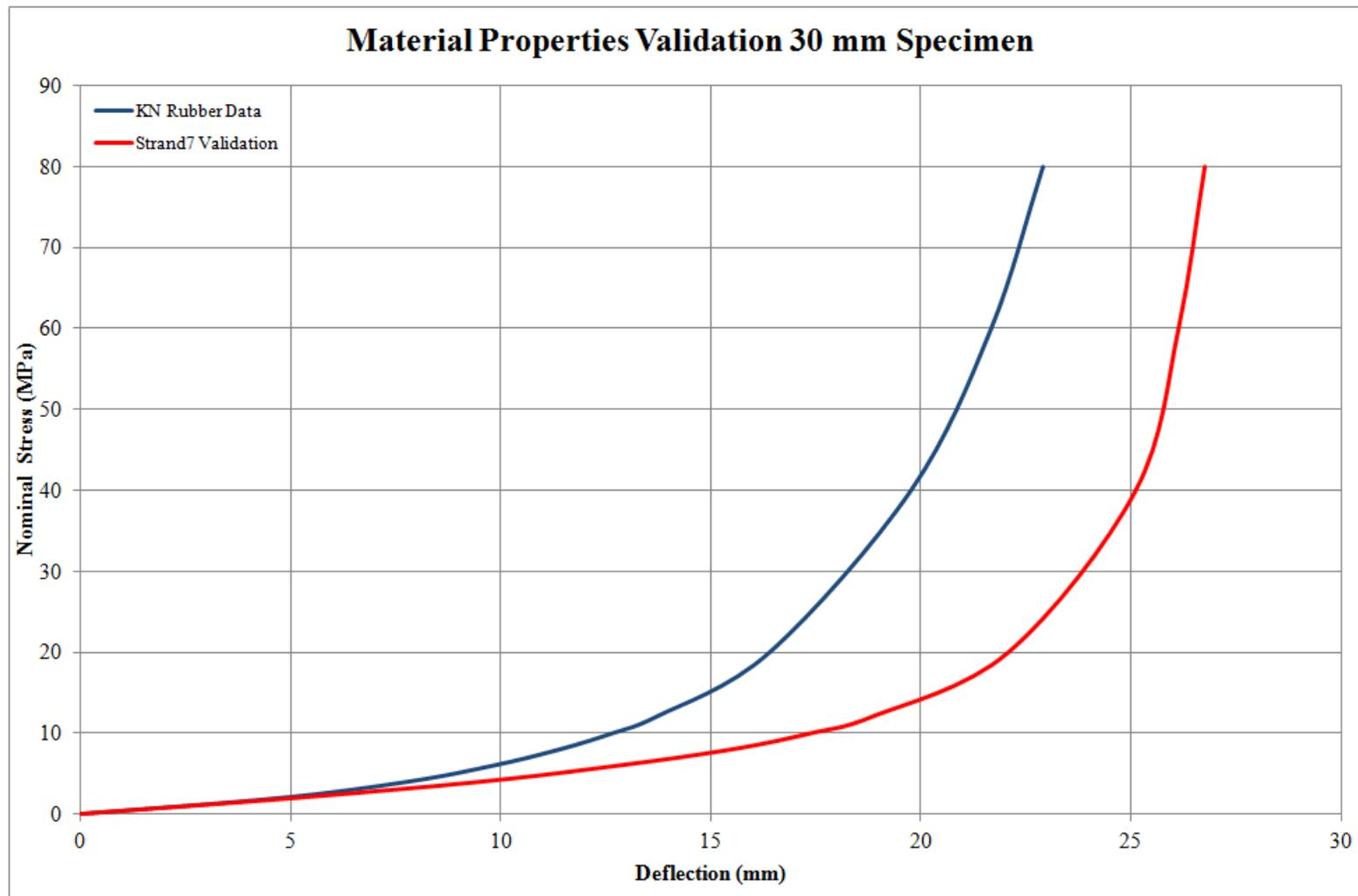
**Figure 4.6:** Material properties validation plot showing KN Rubber extrapolated data and Strand7 results for a 30.0 mm specimen.
