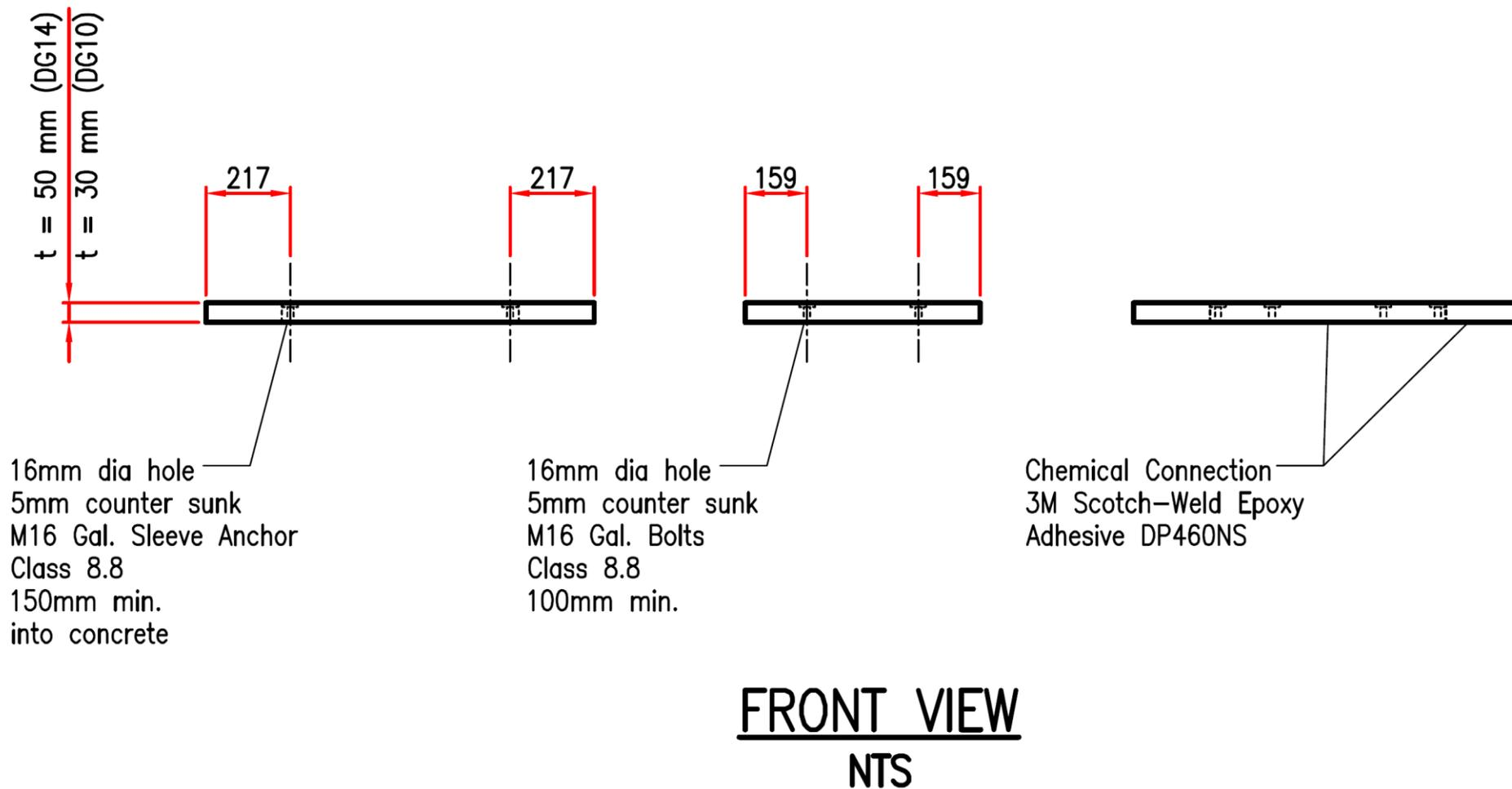
Figure 4.17 (b): RAC detailed design drawing.
