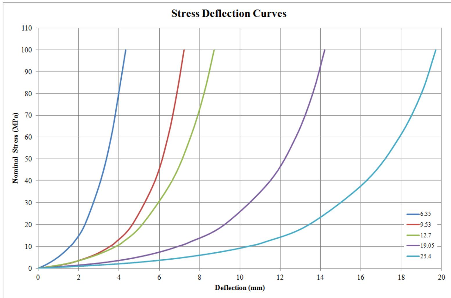
**Figure 3.6:** KN Rubber Symar Bearing Pad stress deflection curves for the XP Bearing Pad (KN Rubber technical brochure, 2015).
