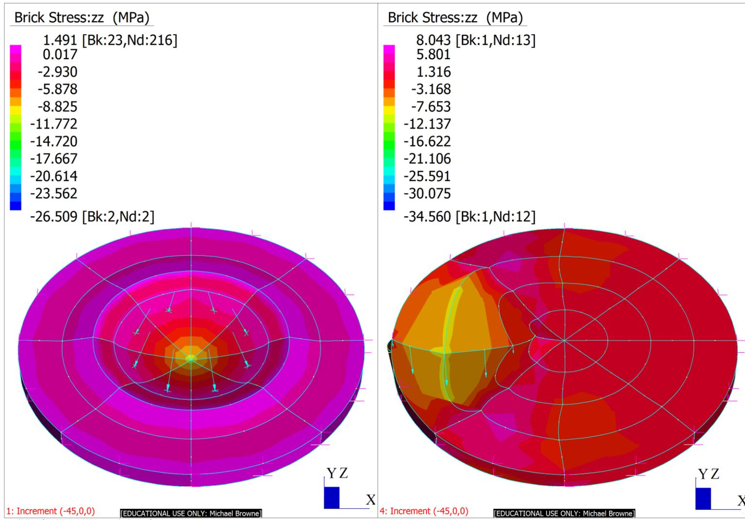
**Figure 4.13:** 30.0 mm RAC load cases 1 (left) and 2 (right) stress distribution and deflection scale 10.0 %.
