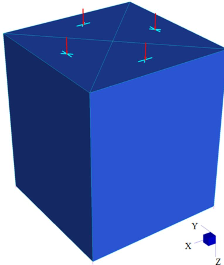
**Figure 4.5:** Material properties validation model, 30.0 mm thick specimen shown.
