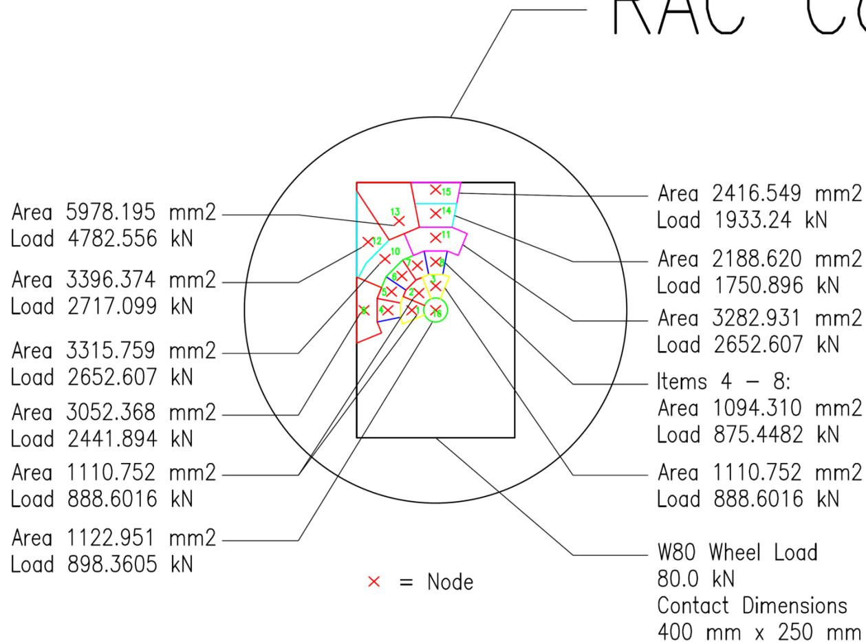
Figure F.3: Area load equivalent calculations for RAC cover riser, W80 wheel load.
