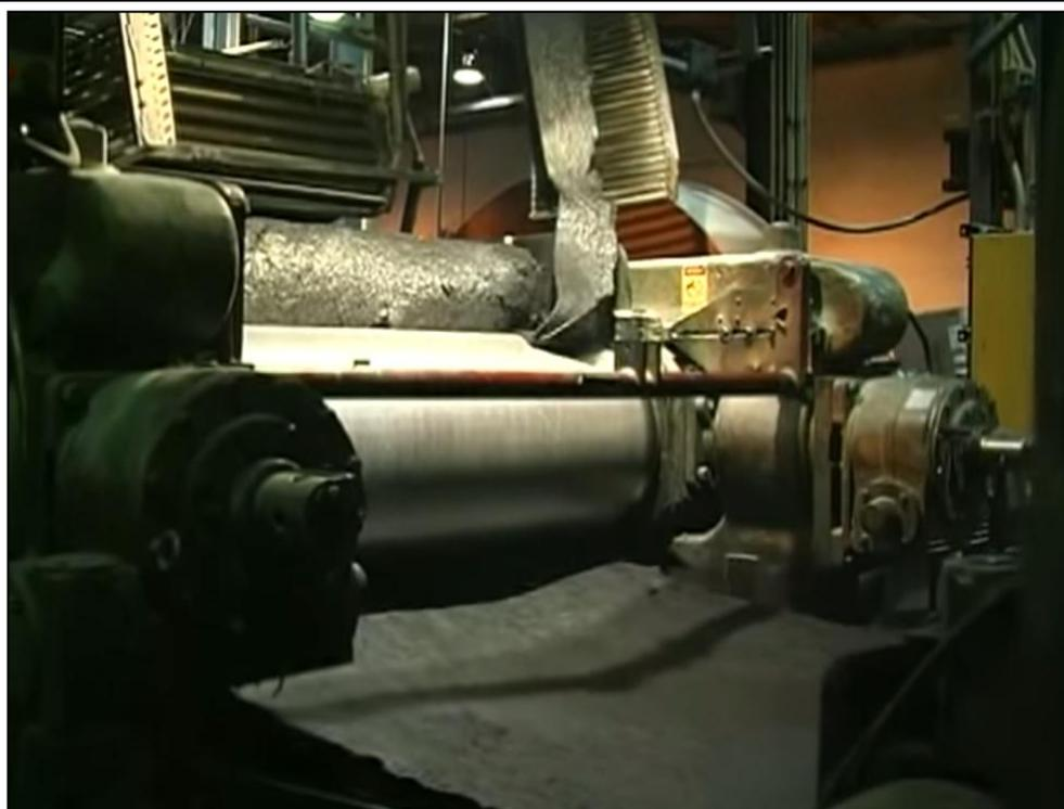
**Figure 3.4:** Calendaring processing into an uncured rubber roll (KN Rubber LLC 2013).
