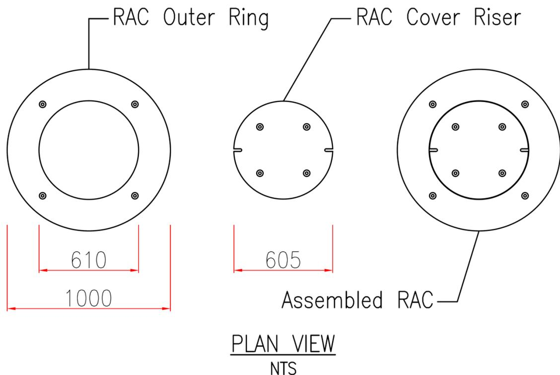
**Figure 3.1:** RAC outer ring, cover riser and assembly.
