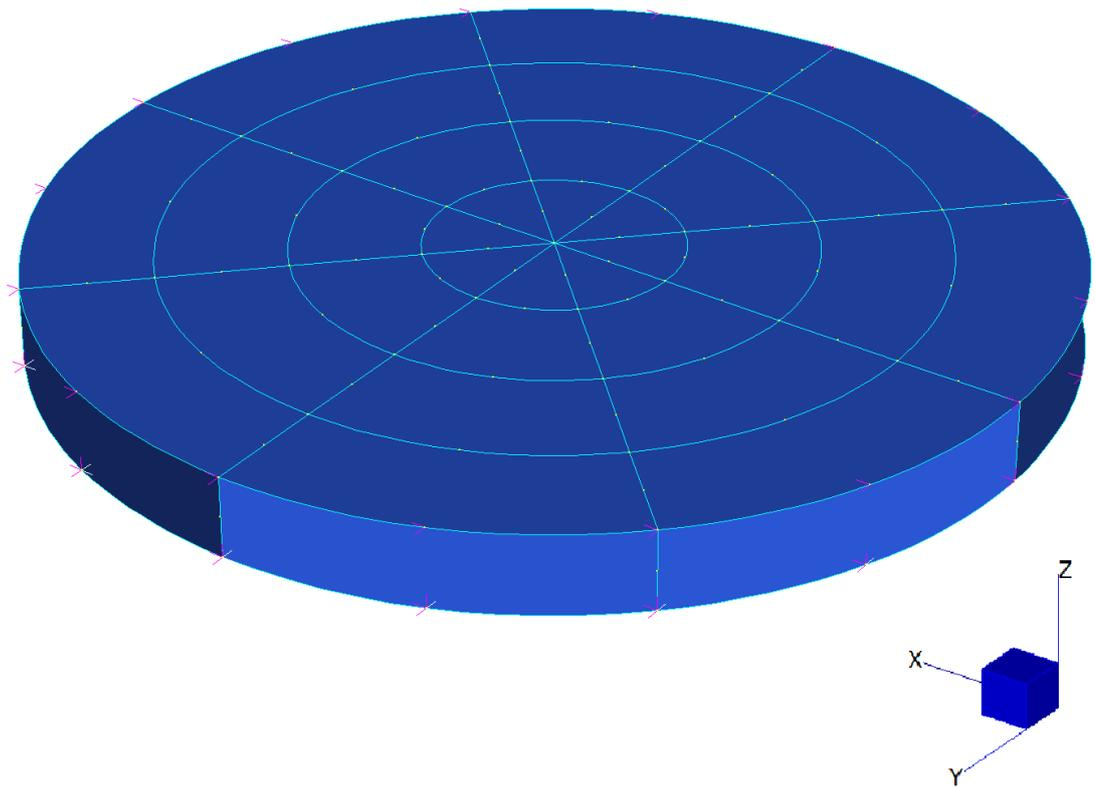
**Figure 4.8:** RAC cover riser model geometry in Strand7.
