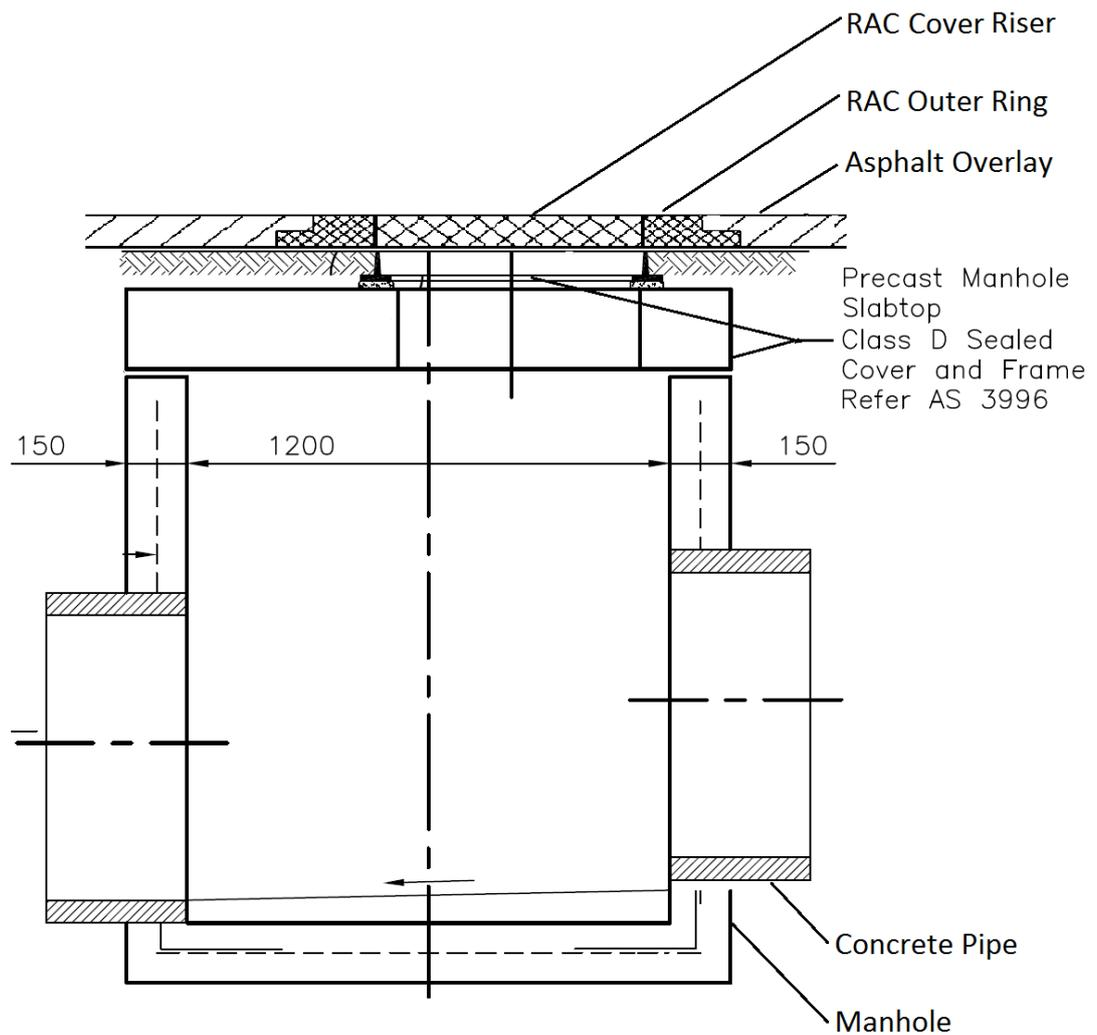
**Figure 5.1:** Diagrammatic sectional view of RAC installed onto a stormwater AC and MH.
