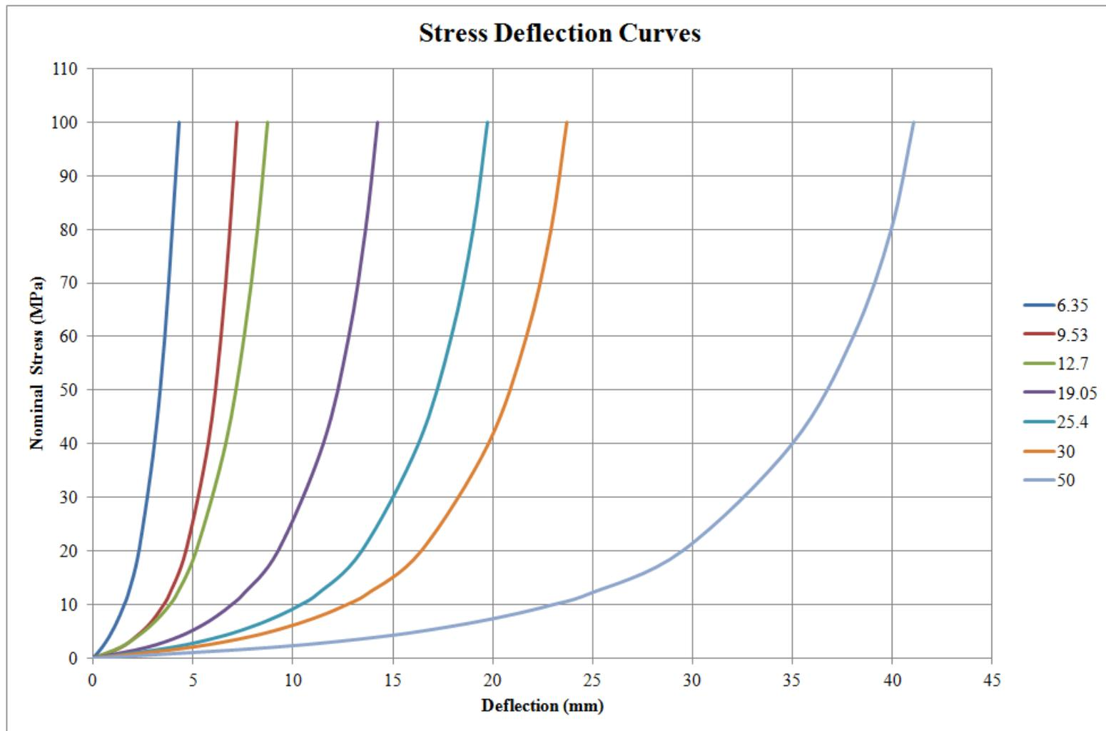
**Figure 4.2:** KN Rubber Symar Bearing Pad stress deflection curves including extrapolated 30.0 mm and 50.0 mm thicknesses.
