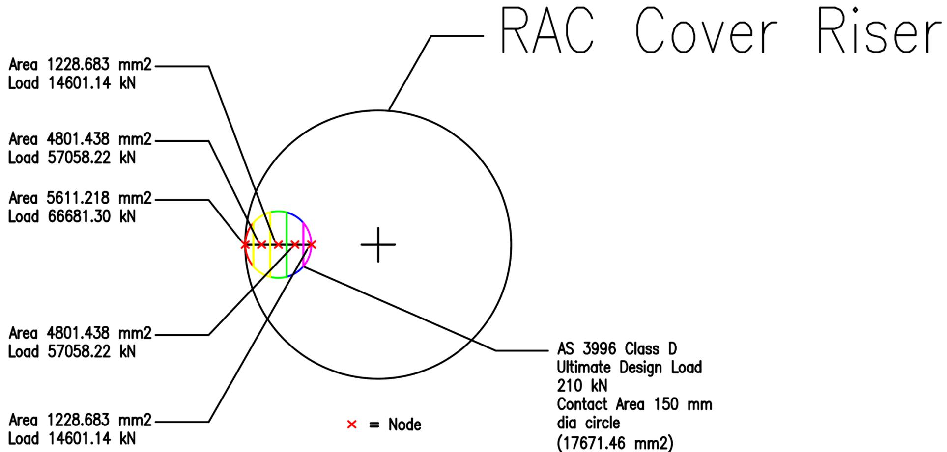
Figure F.1: Area load equivalent calculations for RAC cover riser, 210.0 kN load.
