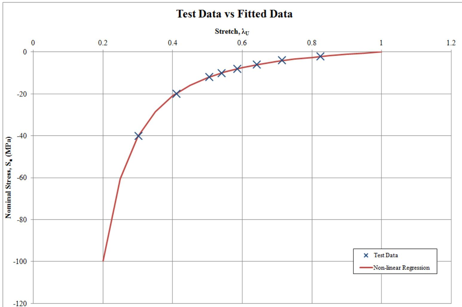
**Figure 4.3:** Comparison of test data with the fitted curve for 30.0 mm specimen.
