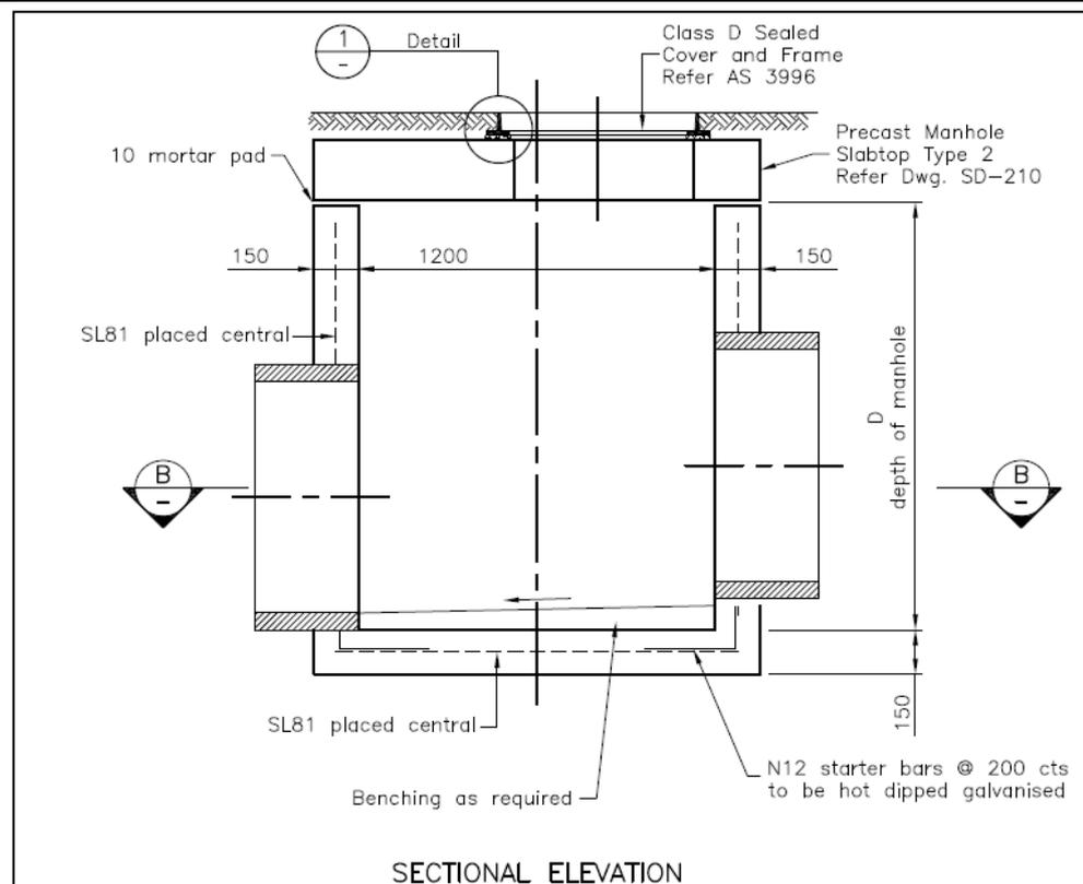
**Figure 1.2:** TCC Type 2 Stormwater MH (TCC Standard Drawing SD-205 C, 2012).
