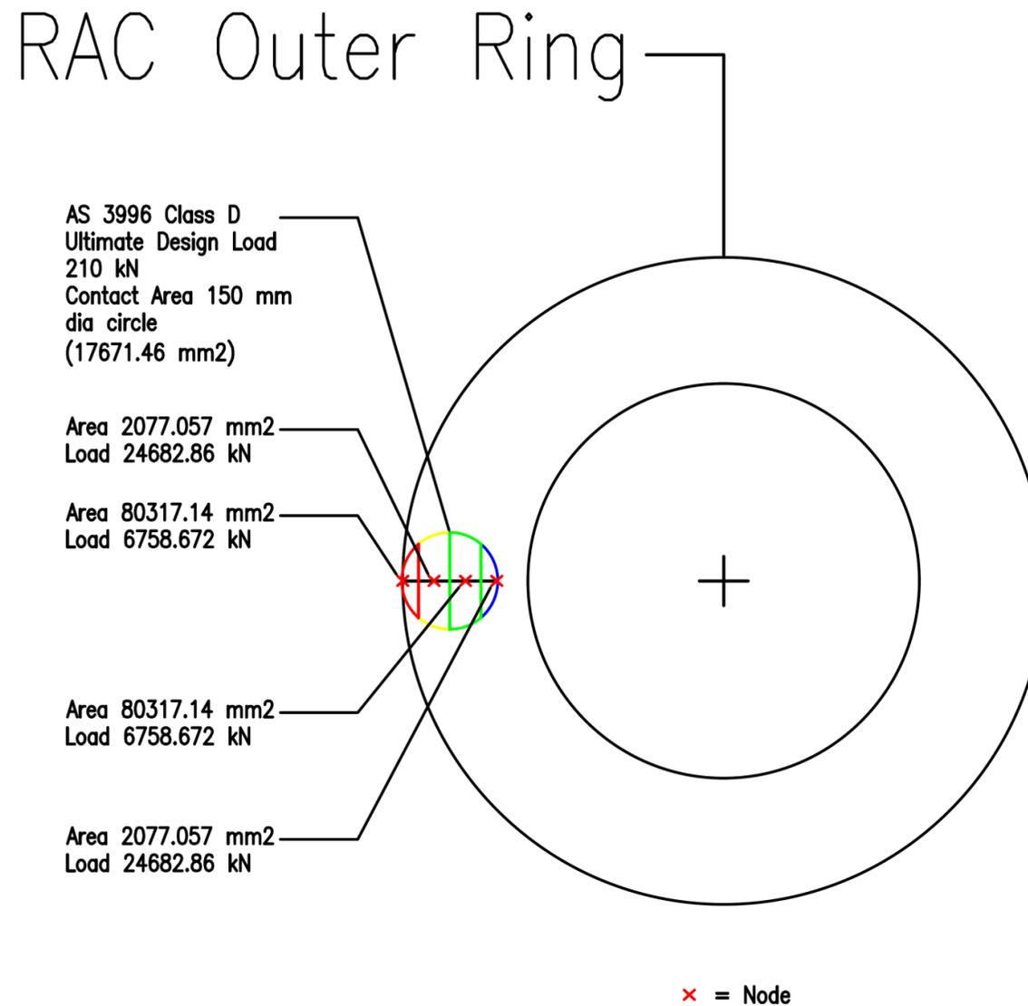
Figure F.2: Area load equivalent calculations for RAC outer ring, 210.0 kN load.
