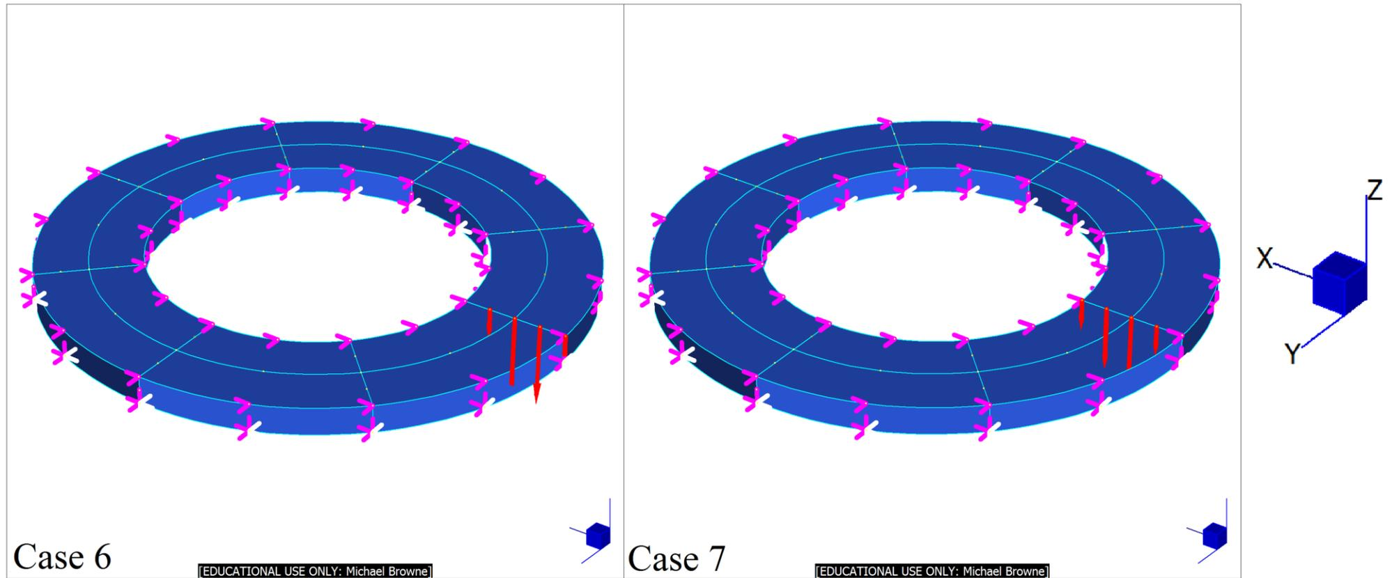
**Figure 4.12:** Load cases 6 and 7, and model restraints for the outer ring in both 30.0 mm and 50.0 mm thicknesses.
