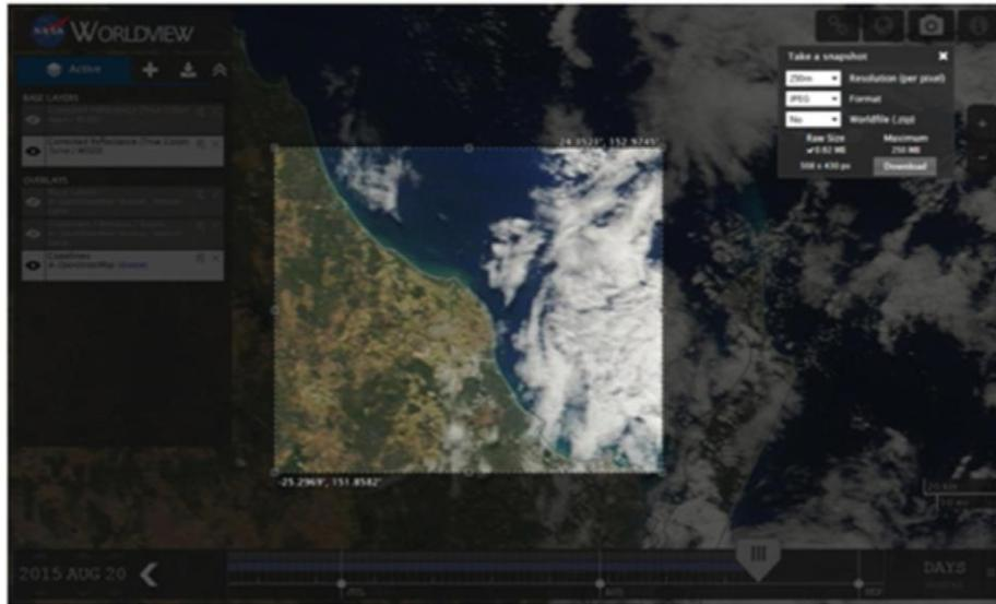
Select the area by adjusting the box. All unshaded areas will be downloaded. Resolution should be 250m (if image file is too large this can be adjusted higher), format should be KMZ and a zip is not required.
