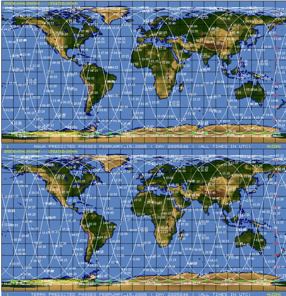
Figure 2.2: Example path of the Aqua satellite (top) and Terra satellite (Bottom) during the same time period. (NASA, 2005)
