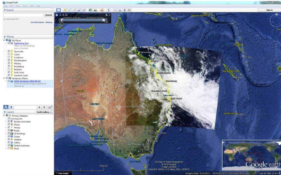
Figure 5.20: Screenshot of Tropical Cyclone Ita satellite image overlaying the Google Earth Globe. Notice the shape of the image once it has been geo-rectified by the GIS software.
