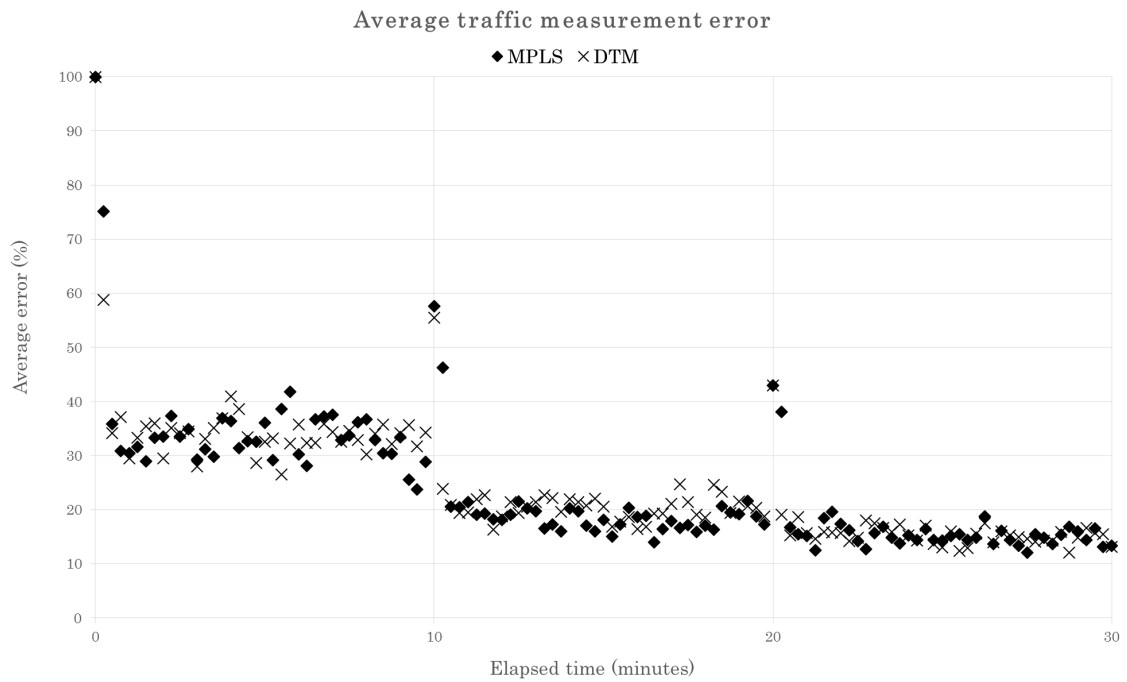
Figure 5.5: Network performance measurements — Average percent demand error
