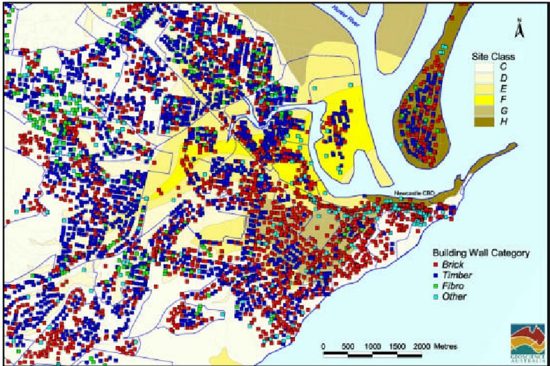
Figure 41: Building Wall Construction Type (Source: GA, 2002)
