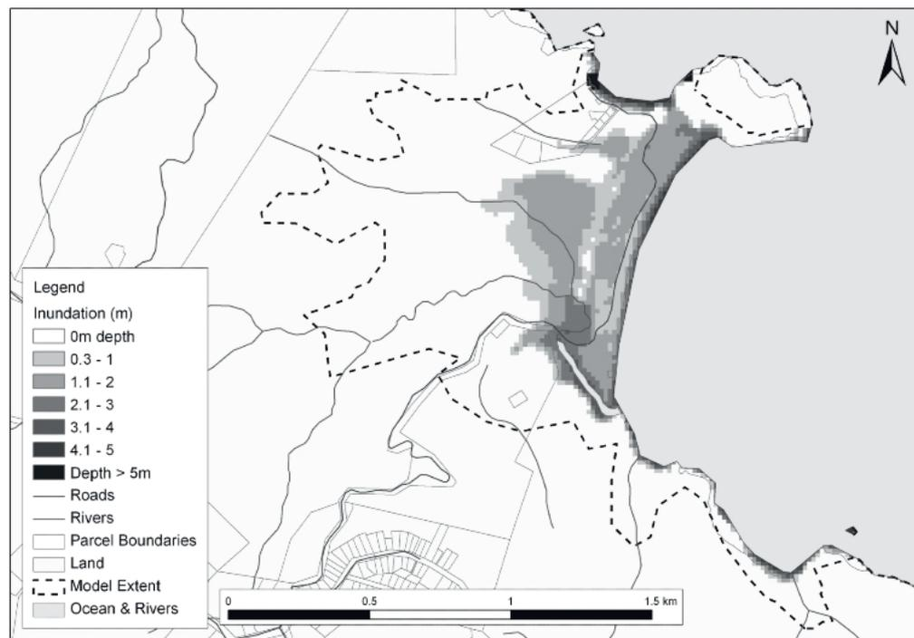
Figure 25: Example RiCOM Inundation Model - New Zealand (Source Lane et al. 2011)
