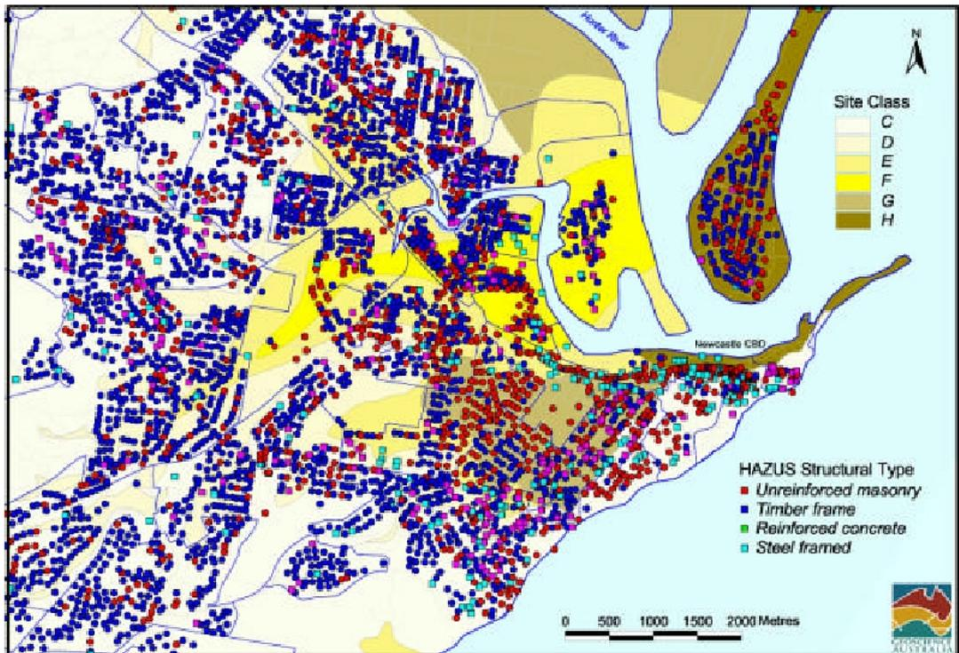
Figure 42: Building Wall Construction Type (Source: GA, 2002)
