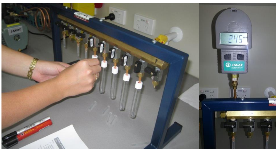
Figure 3.19: Vacuum apparatus set-up to vacuum gas sample vials prior to use (NCEA Laboratory)
