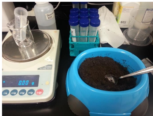
Figure 3.18: Soil sample mixing and removal for further analysis
