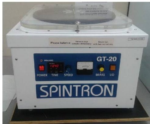
Figure 3.23: Centrifuge machine used to separate soil solids from extraction liquid prior to filtration
