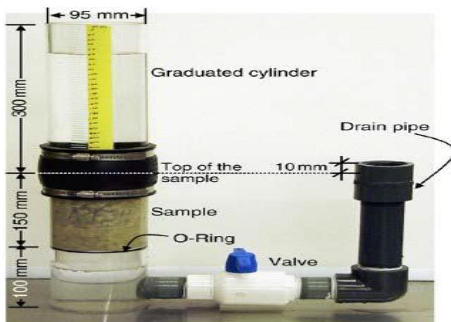
Figure 11: Permeability testing by the falling head method (Neithalath, et al., 2006)
