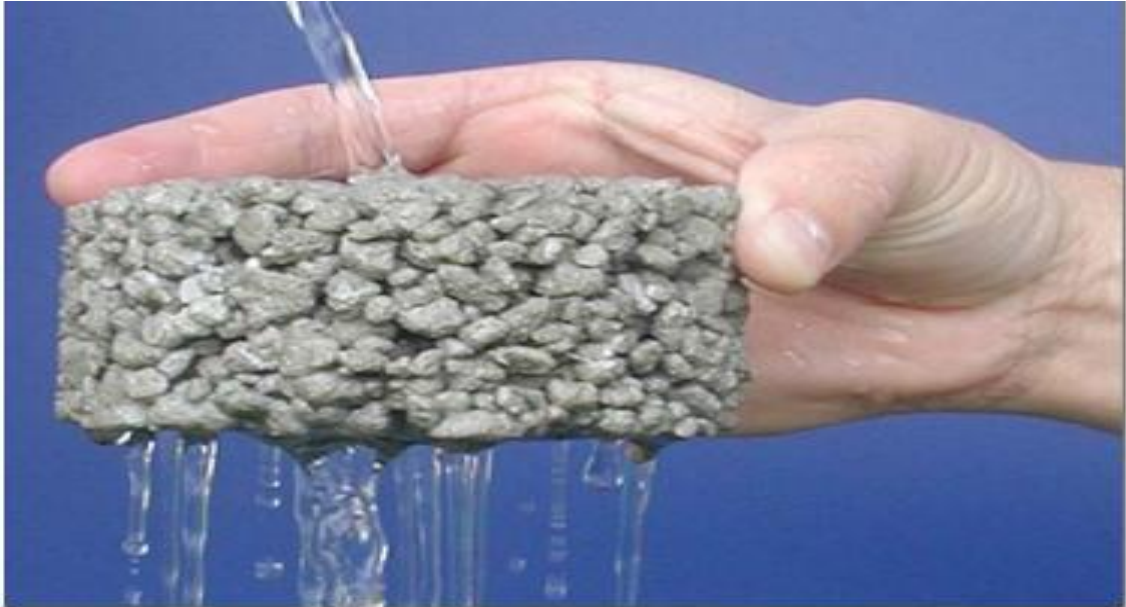
Figure 2: This picture depicts the porous structure of a permeable concrete sample, thus revealing its relation to permeability (Yukari, 2009).
