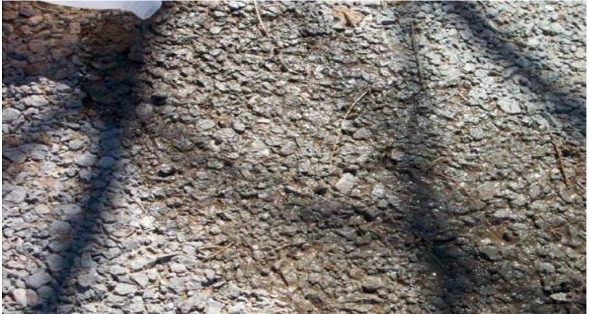
Figure 4: Permeable concrete showing blocking of the pores termed clogging (Tennis, et al., 2004)
