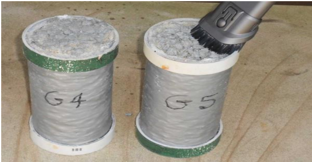
Figure 17: Vacuuming sample after clogging with sand
