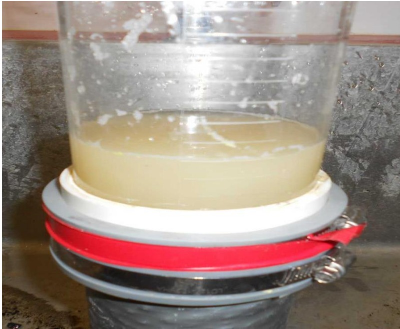
Figure 15: Using sand as a sedimentation type. The picture above represents the effect sand has on water turbidity.
