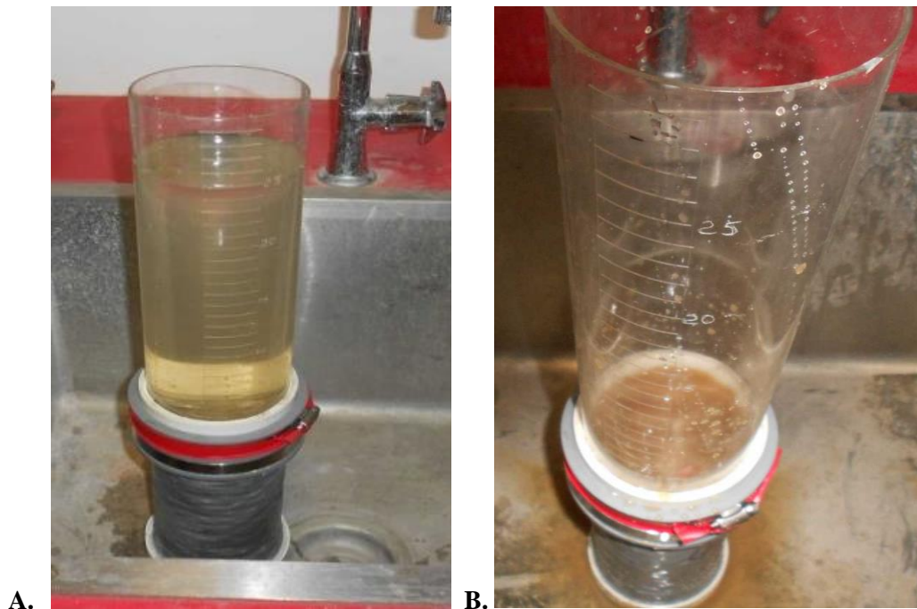
Figure 12: A. Contaminating the sample with 0.5m of stormwater water was poured in quickly to allow head to build up. B: contaminating the samples by pouring the equivalent of 0.5m of dirty water, but at a slower rate to keep the head of water below 50mm. These photos were taken in the USQ laboratory during testing.
