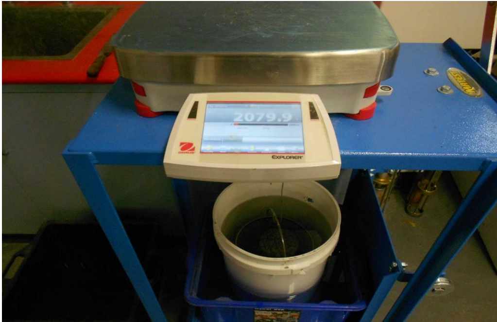
Figure 10: Finding the submerged weight of a sample by placing sample in a bucket of water for 60 minutes then taking a reading from the scale
