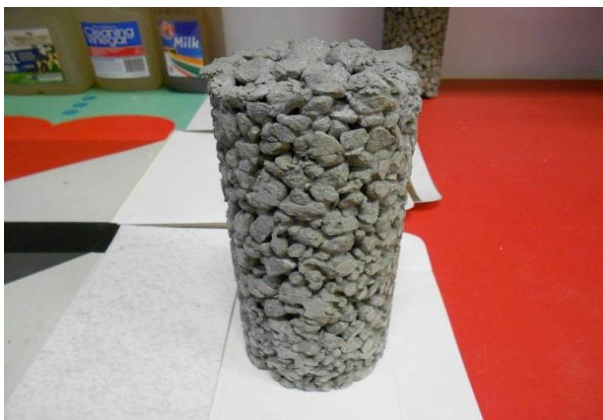
Figure 3: Shows the different appearance and surface of permeable concrete (left) compared with conventional concrete on the (right) photos from USQ laboratory
