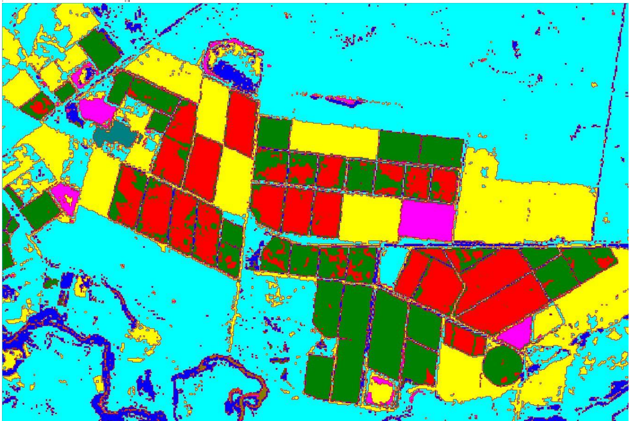
Figure 4.11: Enlarged ENVI supervised segmented result of eight classes from user predefined class set (Exelis 2012)
