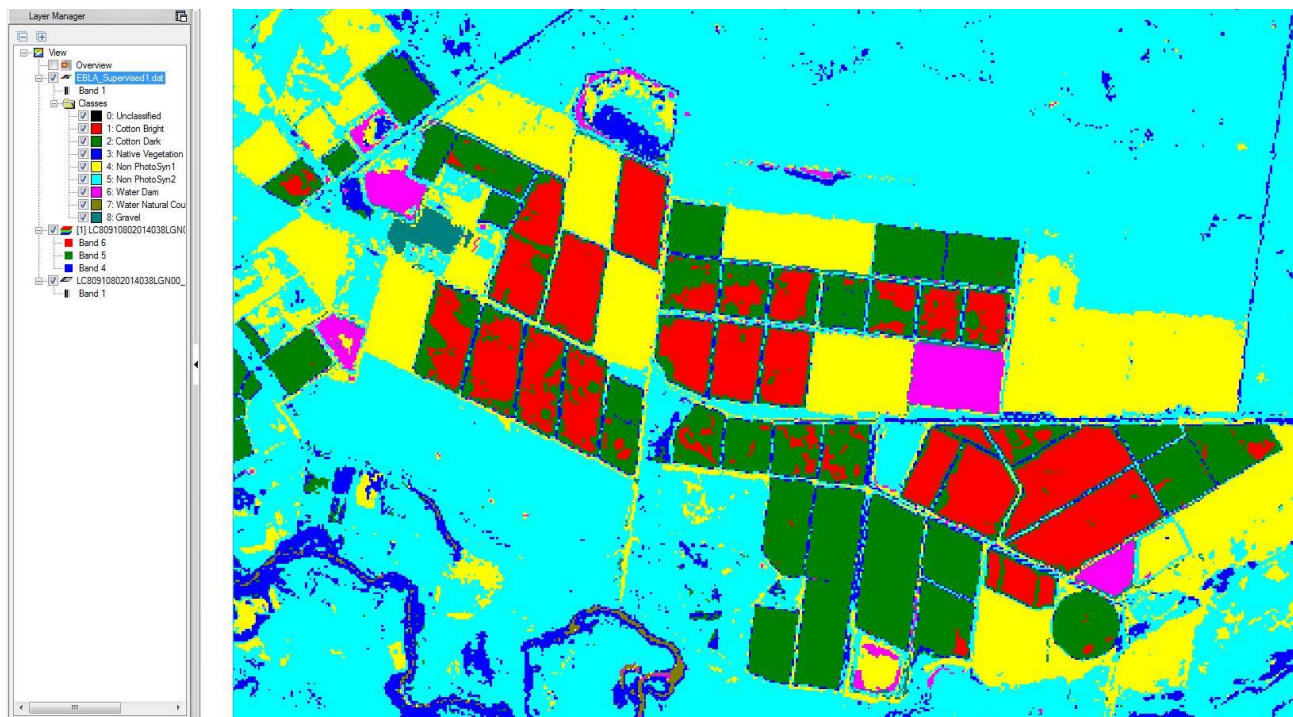
Figure 4.10: ENVI supervised segmented result of eight classes from user predefined class set (Exelis 2012)
