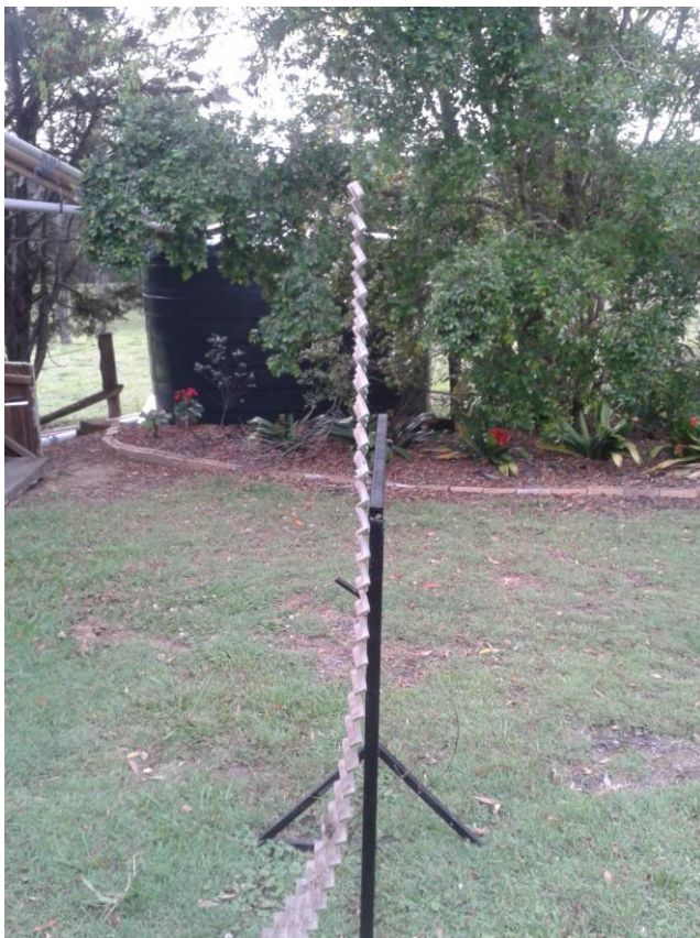
Figure 26 Expanded Mesh Obstruction set-up
