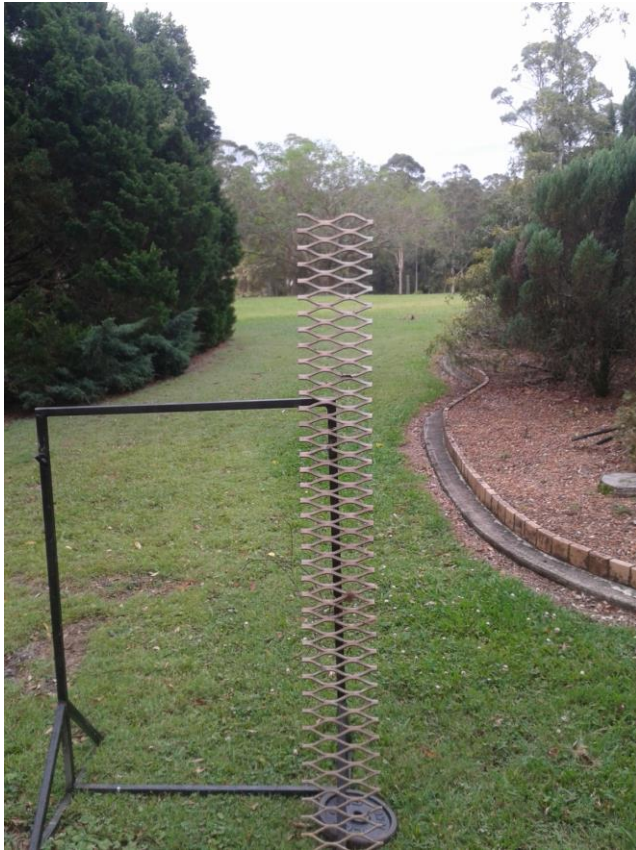
Figure 25 Expanded Mesh Obstruction set-up
