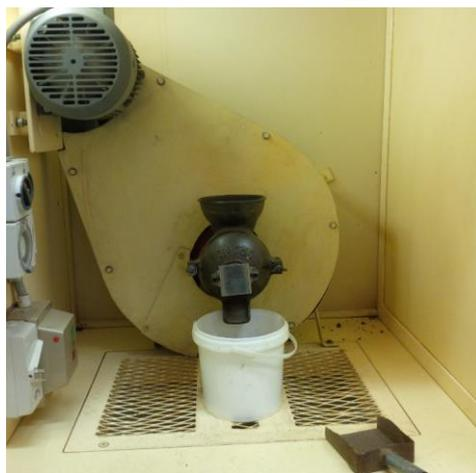
Figure 3.2: Soil Grinder at the DAFF facility Tor St, Toowoomba
