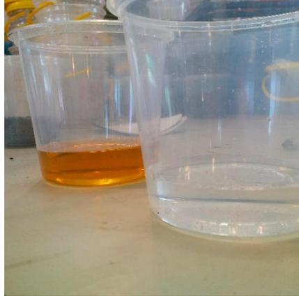
*Figure 3.9: Visual comparison of filtered effluent (background) with leachate (foreground)*
