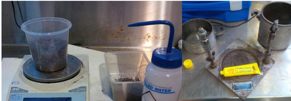
Figure 3.3: Acquiring OMC gravimetrically left, part of the Proctor test apparatus right
