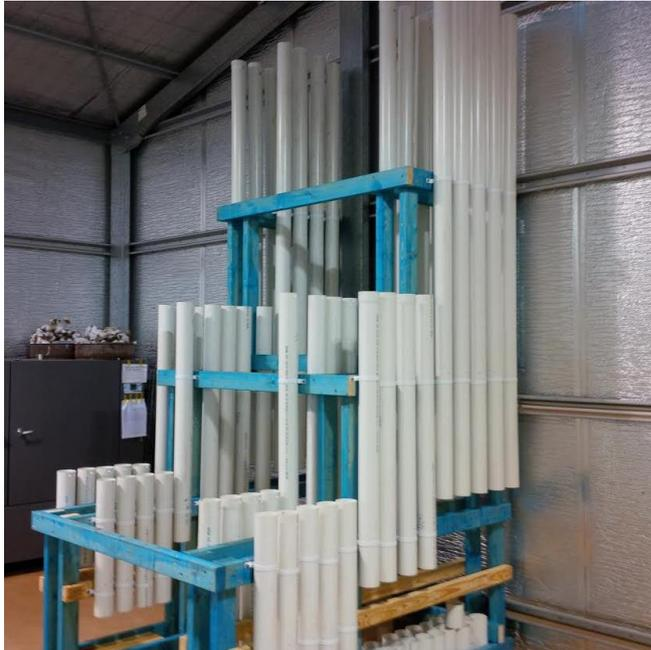
*Figure 4.2: PVC reservoirs for the purpose of ponded head containment*
