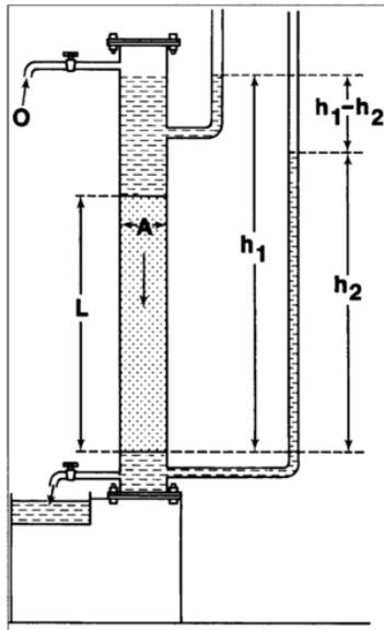
Figure 2.1: Apparatus used by Darcy to develop Darcy's law (Darcy, 1856)
