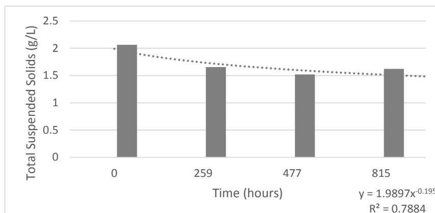
Figure 5.3: Total Suspended Solids TSS (g/L) measured at different time intervals. Time point zero, is that of the effluent, the other time points are that of the leaching fluid.
