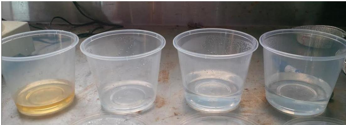
*Figure 5.2: Colour comparison of leachate (right) with effluent (left). Time intervals of sample collection are 0, 259, 477 and 815 hours (left to right) after application of head to cores*
