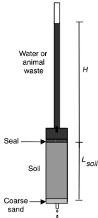
Figure 2.4: example of filtercake experimental apparatus used by Cihan, Tyner and Wright (2006)
