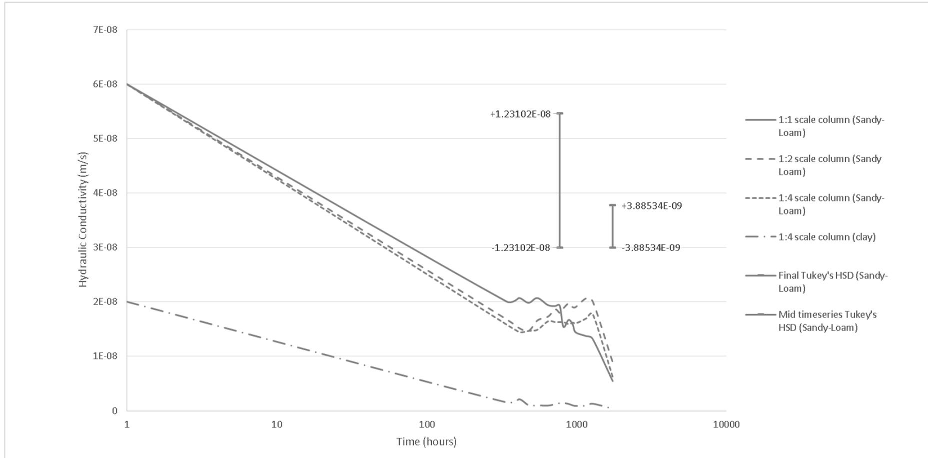
Figure 5.4: Comparison of hydraulic conductivity between effluent leachate column scales
