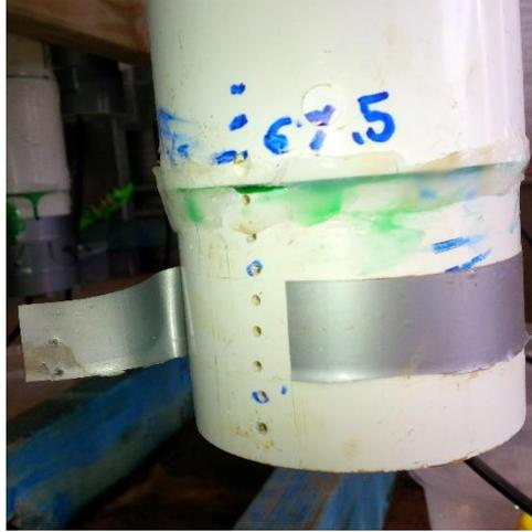
*Figure 3.10: Determination of the lower boundary of the saturated zone*
