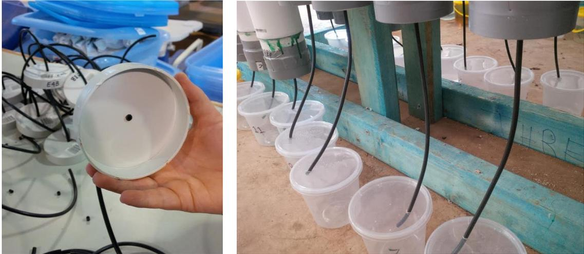
Figure 3.7: (left to right) attaching tube to endcap, anti-evaporation system once installed.
