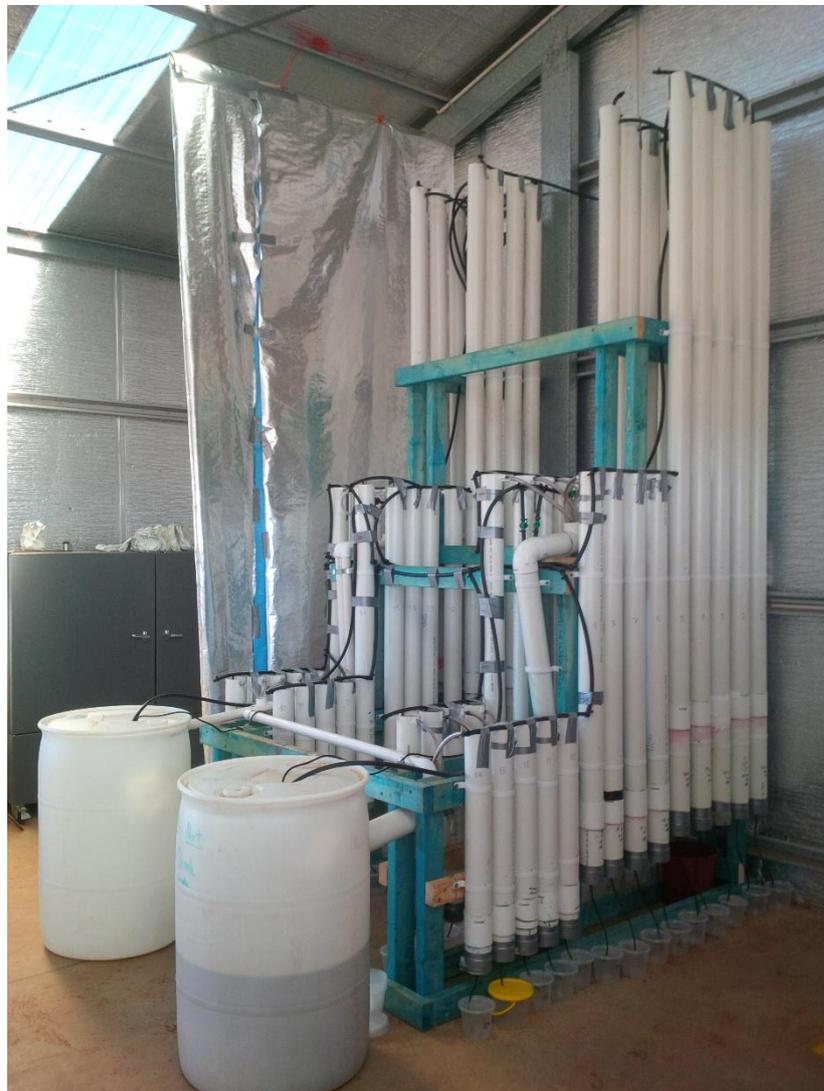
*Figure 3.1: Complete assembly of effluent leachate apparatus*
