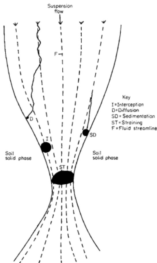
Figure 2.3: Methods of colloidal entrainment (Vinten & Nye 1985)
