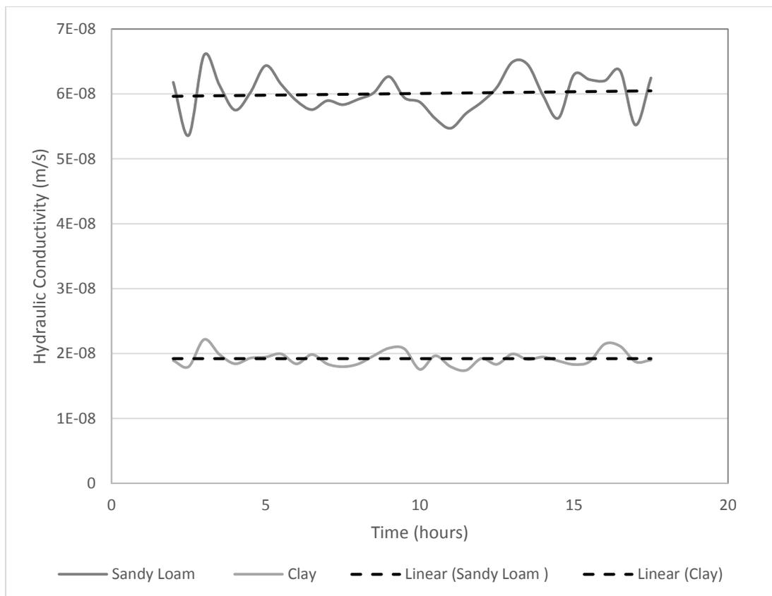
Figure 5.1: Comparison curve of flux of soils subjected to calcium chloride leachate
