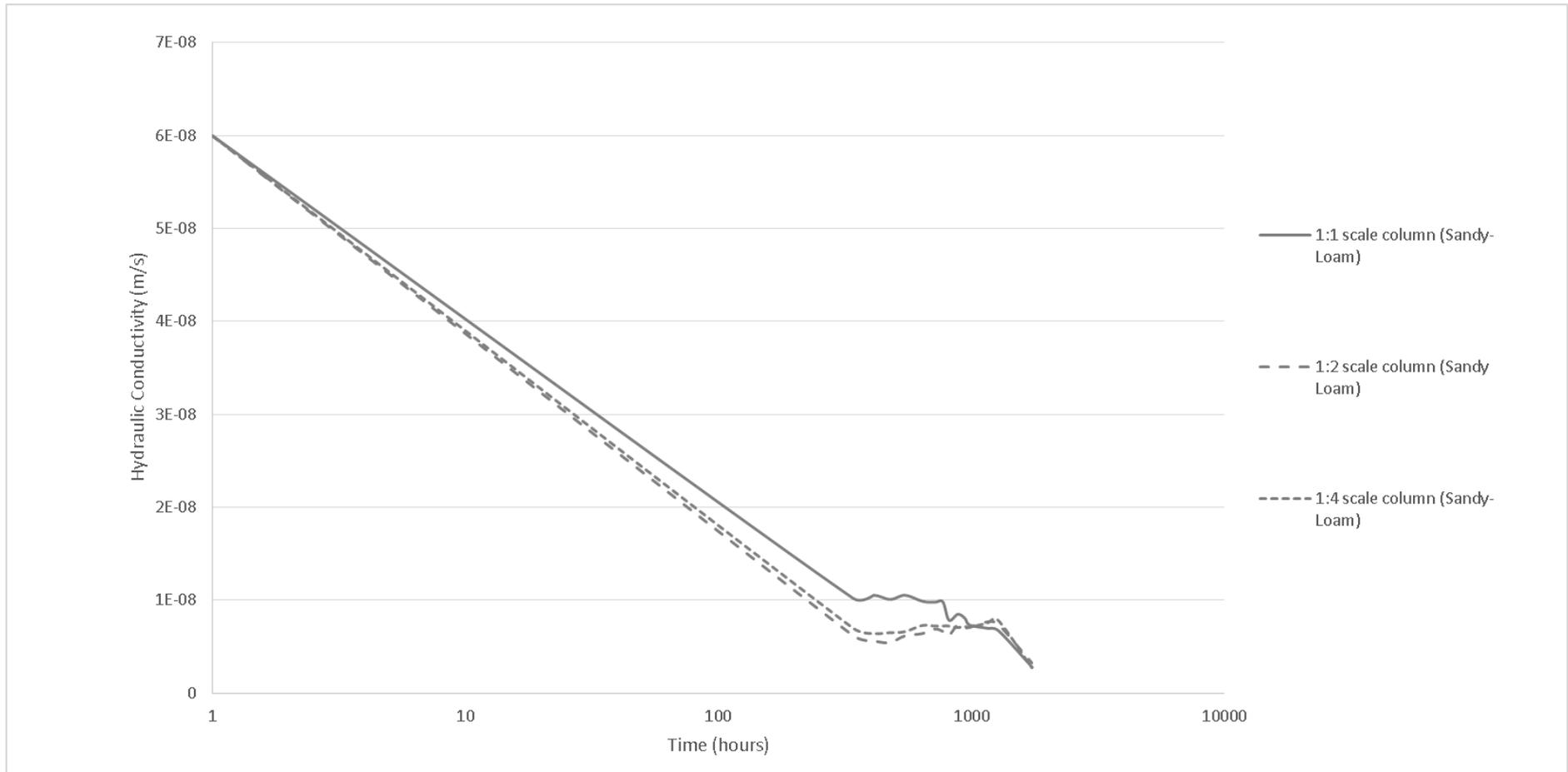
Figure 6.2 Speculative hydraulic conductivity with hydraulic ratio adjusted according to filtercake theory
