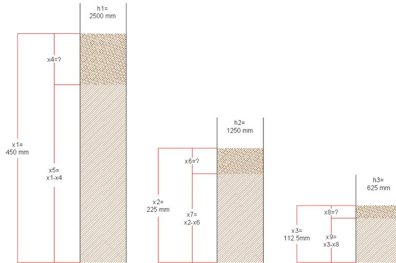
Figure 6.1: Diagram of depth of pore blockage layer expected between scales
