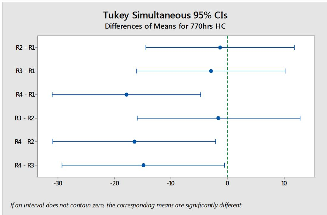
Therefore the sandy-loam column results, at the 770hour mark, are not significantly different. However the 1:4 clay column result is significantly different from the sandy-loam results.
