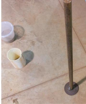
*Figure 3.4: Compaction plate and rod*
