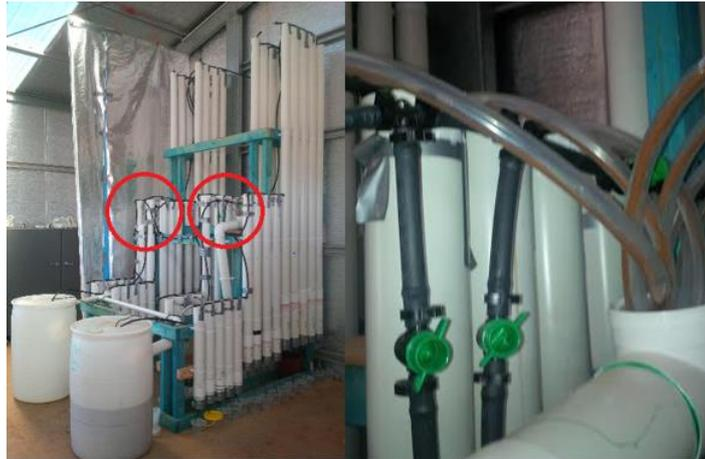
*Figure 4.5: Independent flow regulation valves*
