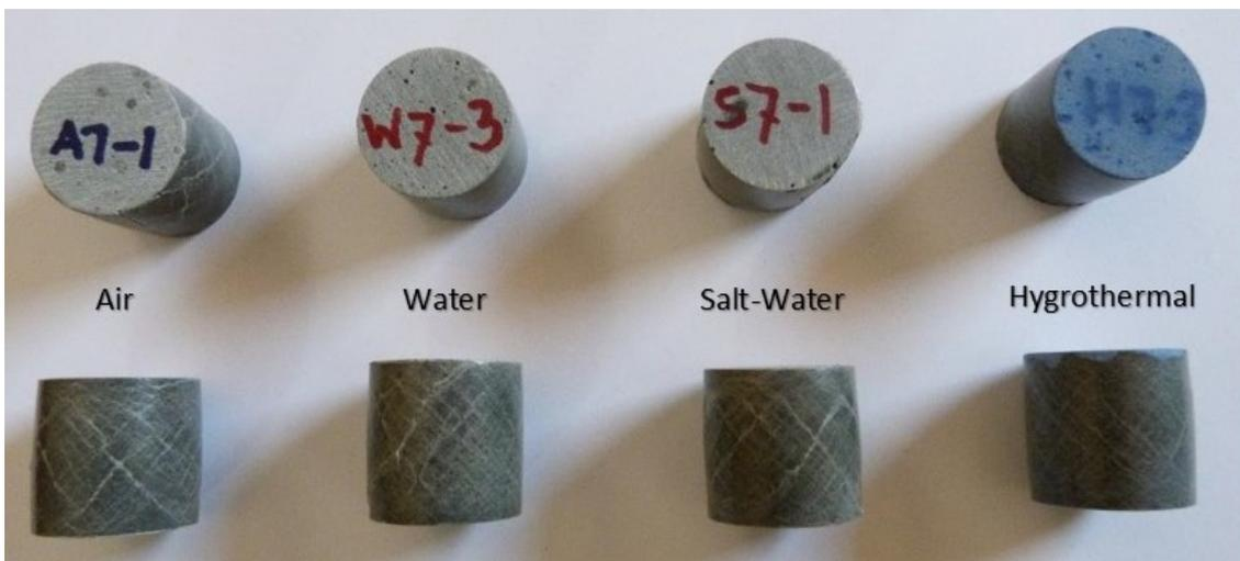
Figure 5.22: Compression Samples at 7 Days
