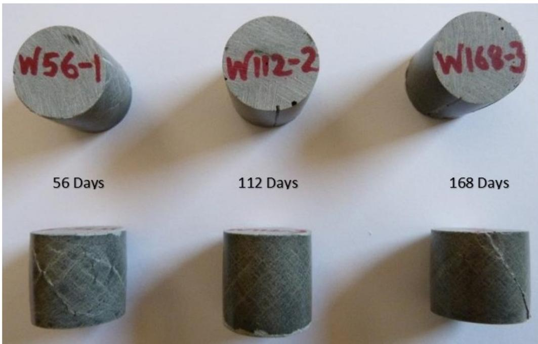
Figure 5.8: Water Environment Compression Samples at Increasing Duration (56 to 168 Days)
