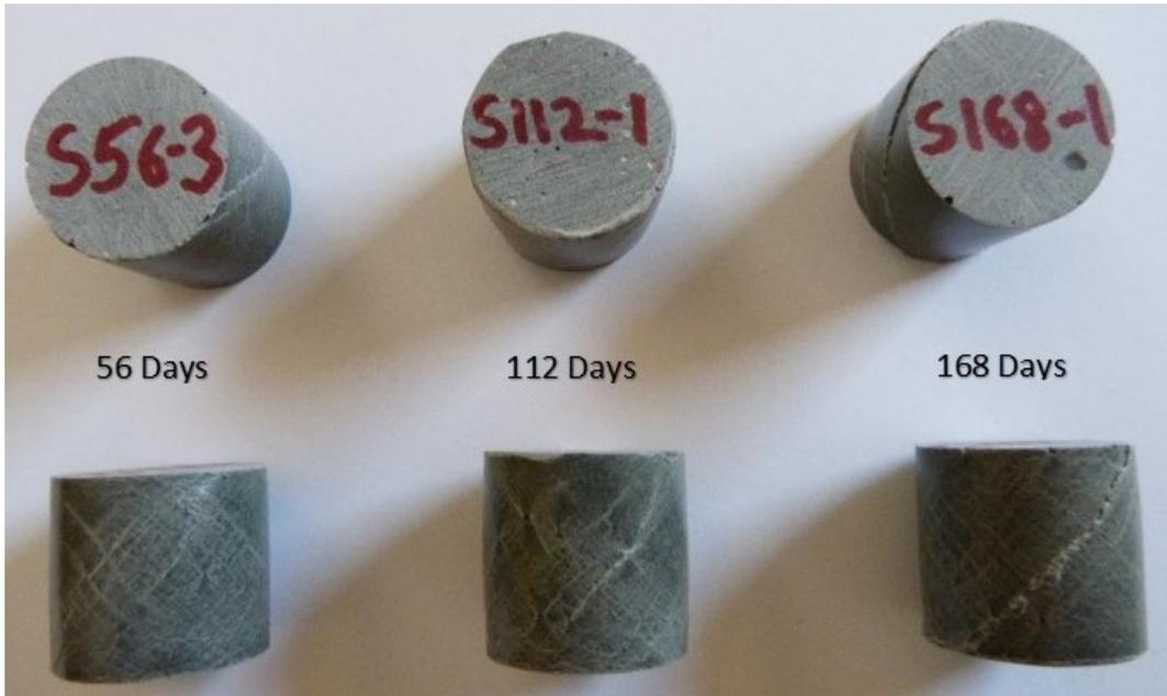
Figure 5.13: Salt-Water Environment Compression Samples at Increasing Duration (56 to 168 Days)
