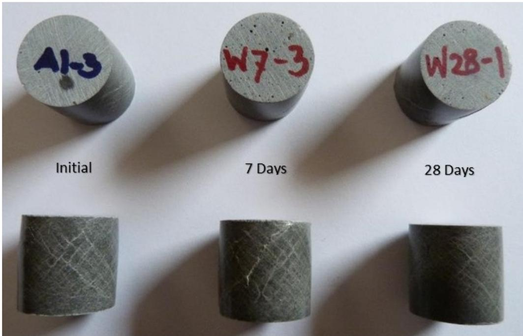
Figure 5.7: Water Environment Compression Samples at Increasing Duration (Initial to 28 Days)
