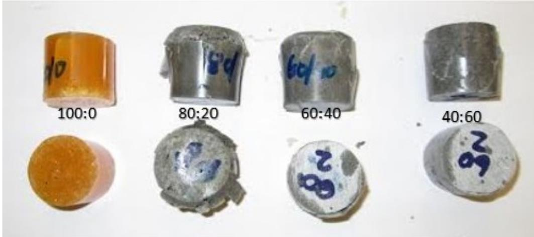
Figure 4.15: 60°C Compression Samples of Increasing Light-Weight Particulate Filler Percentage
