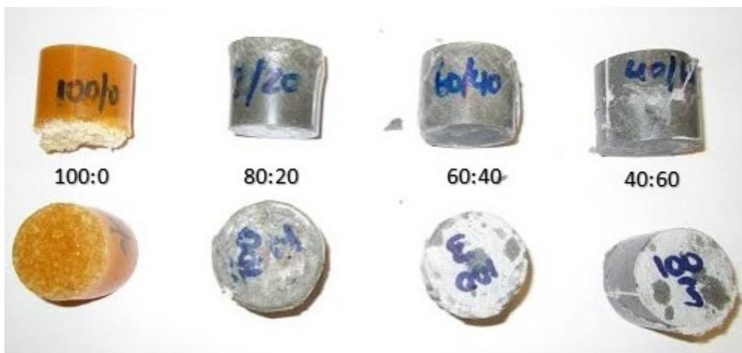
Figure 4.13: 30°C Compression Samples of Increasing Light-Weight Particulate Filler Percentage
