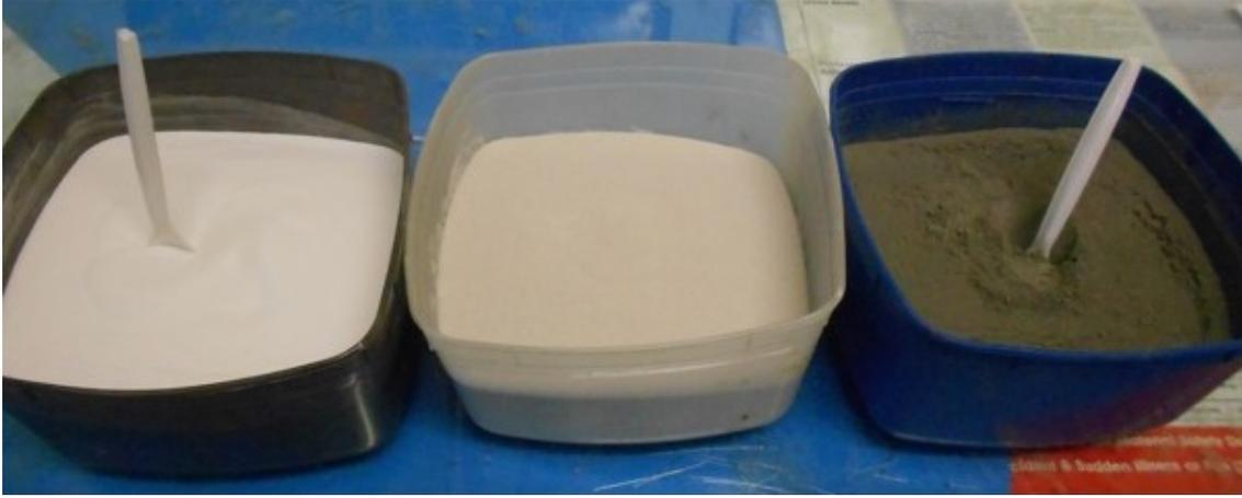
Figure 3.2: Hollow Microsphere, Fire Retardant and Fly Ash Respectively
