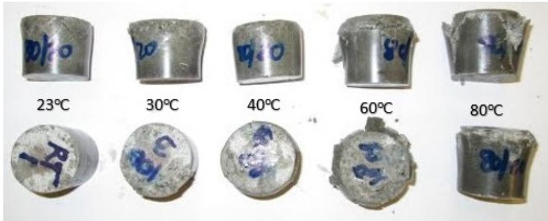
Figure 4.5: 80:20 Epoxy to Filler Ratio Compression Samples at Increasing Temperatures
