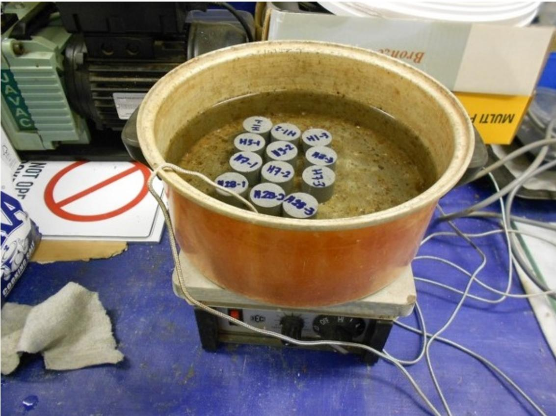
Figure 3.10: Samples in the Hydrothermal Environment
