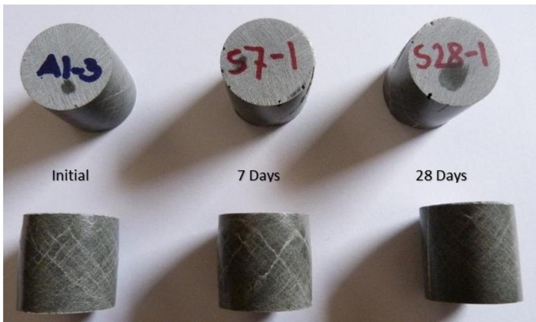
Figure 5.12: Salt-Water Environment Compression Samples at Increasing Duration (Initial to 28 Days)
