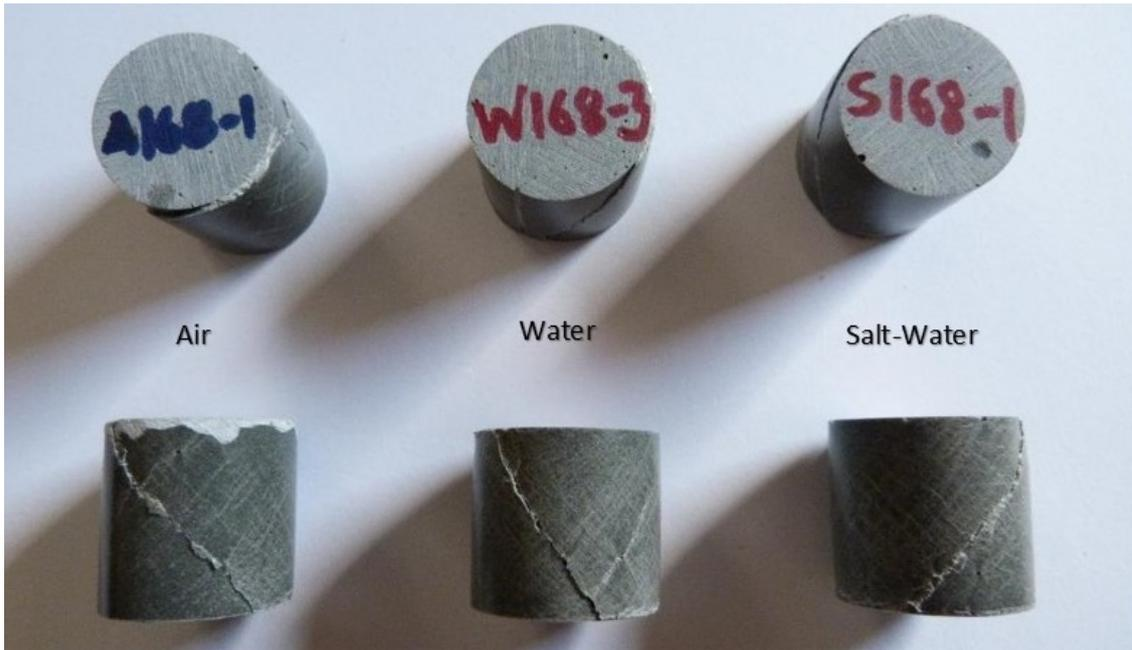
Figure 5.26: Compression Samples at 168 Days
