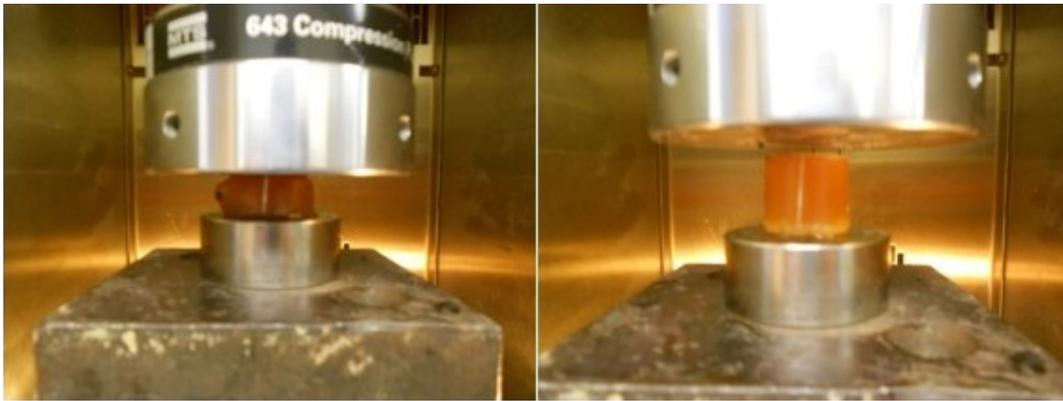
Figure 4.2: Compression Test of 100% Epoxy Resin at 60°C
