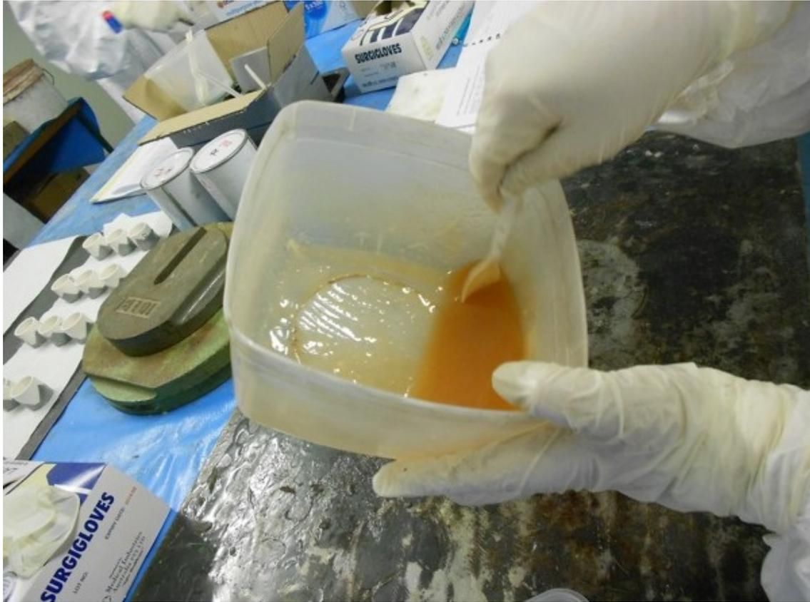
Figure 3.5: Epoxy Resin Materials Being Mixed Together
