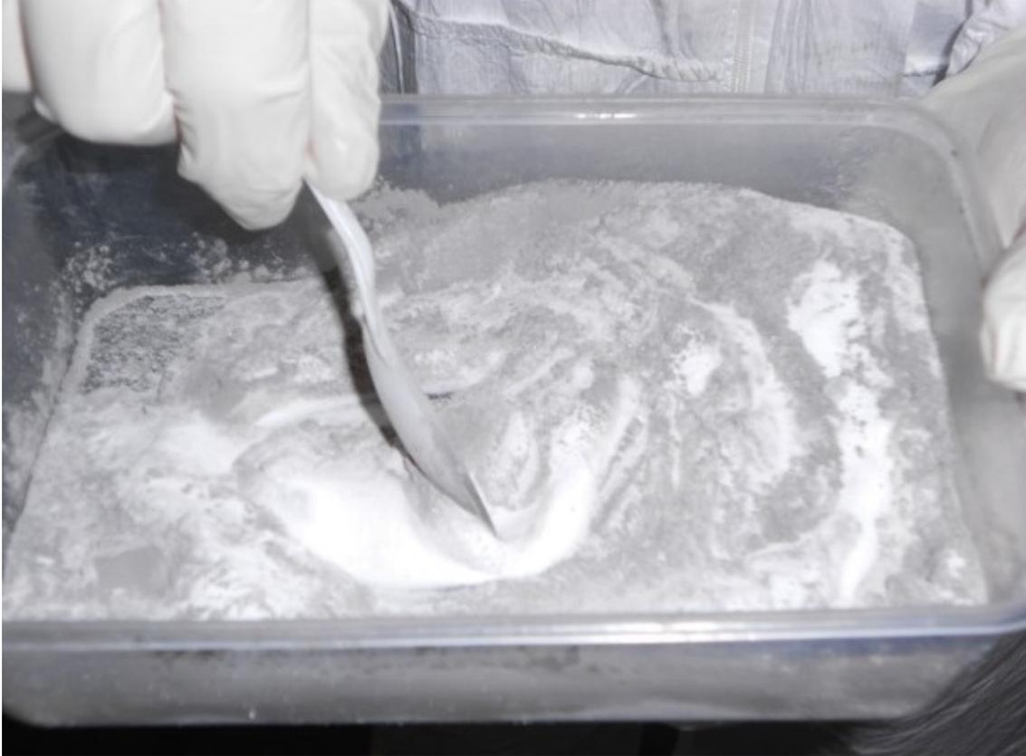
Figure 3.6: Light Weight Particulate Filler Materials Being Mixed Together
