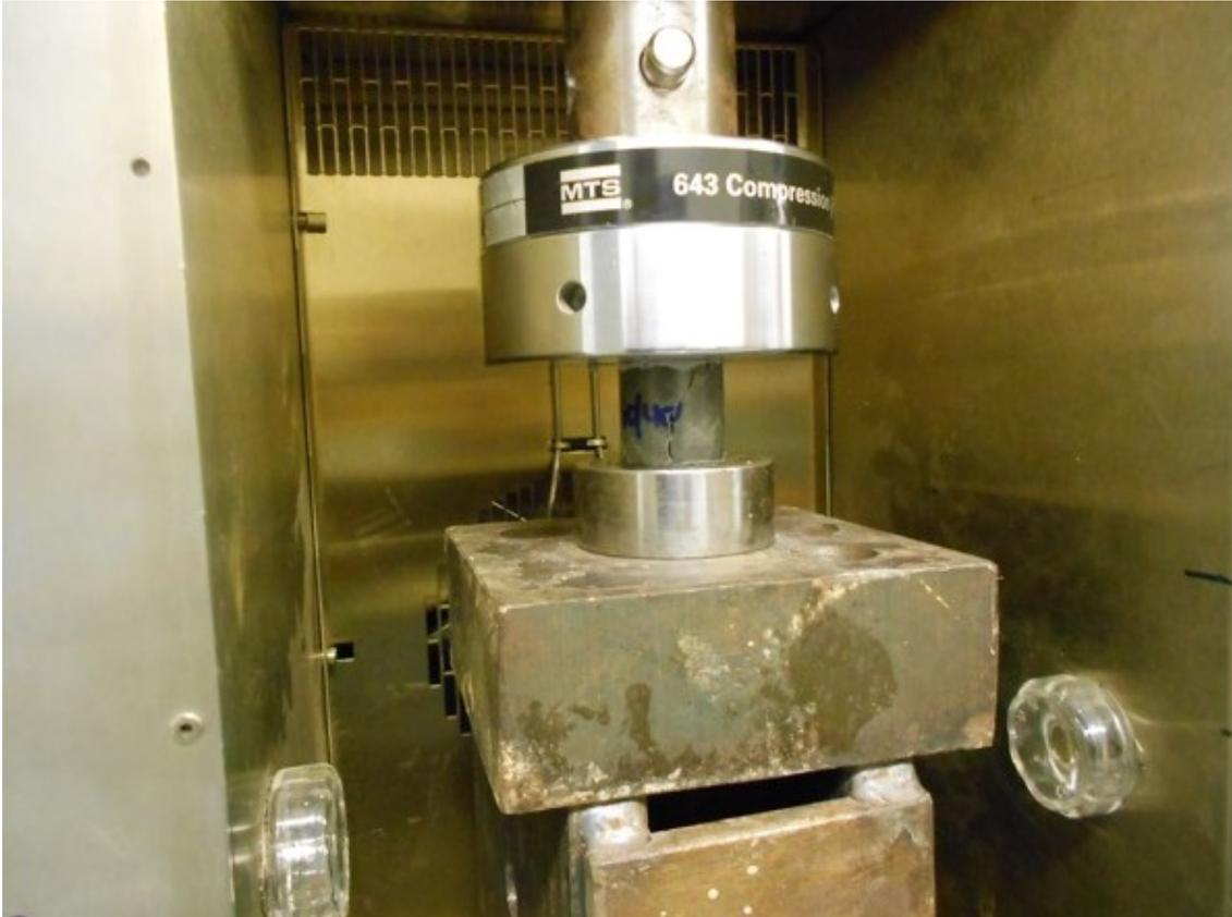
Figure 3.12: Epoxy Resin to Filler Ratio 40/60 Being Tested at Room Temperature
