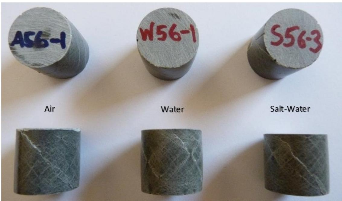
Figure 5.24: Compression Samples at 56 Days
