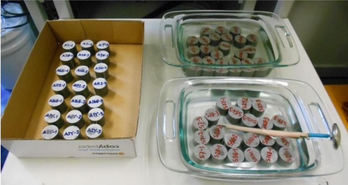
Figure 3.9: Samples in Air (Left), Water (Top Right) and Sea Water Environment (Bottom Right)
