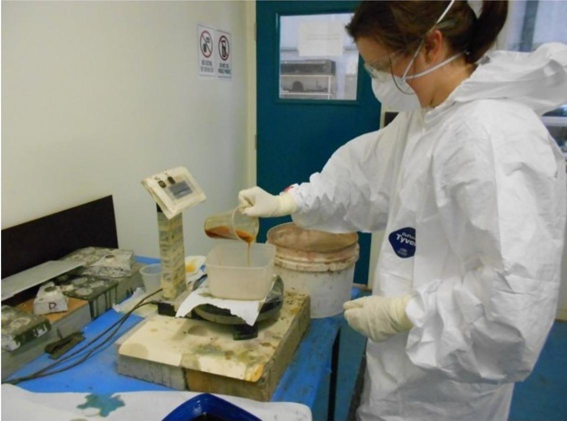
Figure 3.4: Measuring Part B into the Container Containing the Pre-Measured Part A
