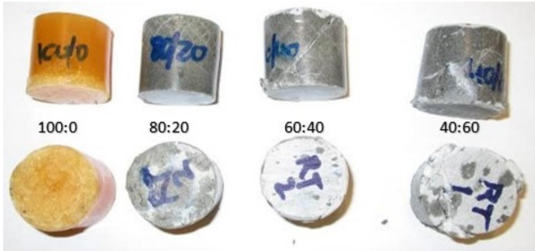
Figure 4.12: Room Temperature Compression Samples of Increasing Light-Weight Particulate Filler Percentage
