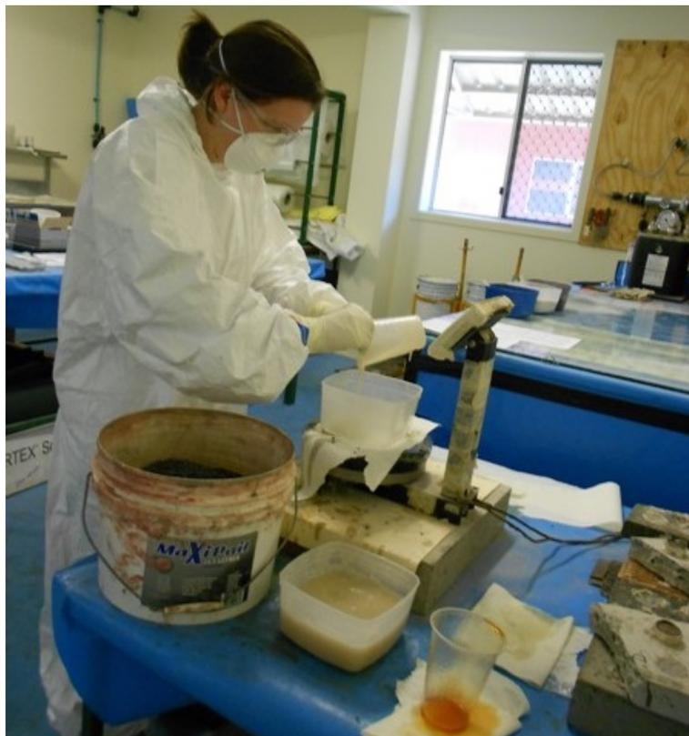
Figure 3.3: Measuring Part A into 2L Container
