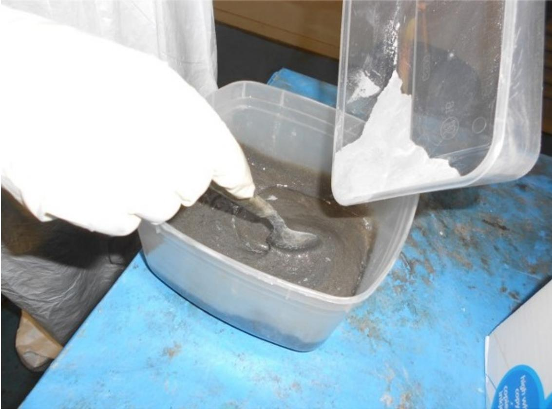
Figure 3.7: Combining Light Weight Filler and Epoxy Resin
