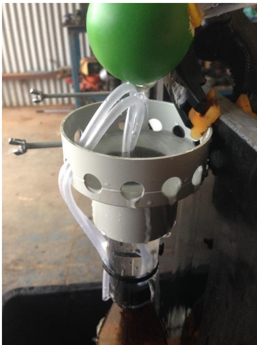
Figure 7-9 flow duration indicator being tested with a 1.6L/min flow rate
