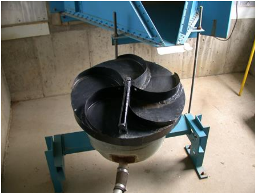
Figure 2-2 Commercially available Coshocton wheel sampler, a type of rotational flow sampler (Open Channel Flow 2013)
