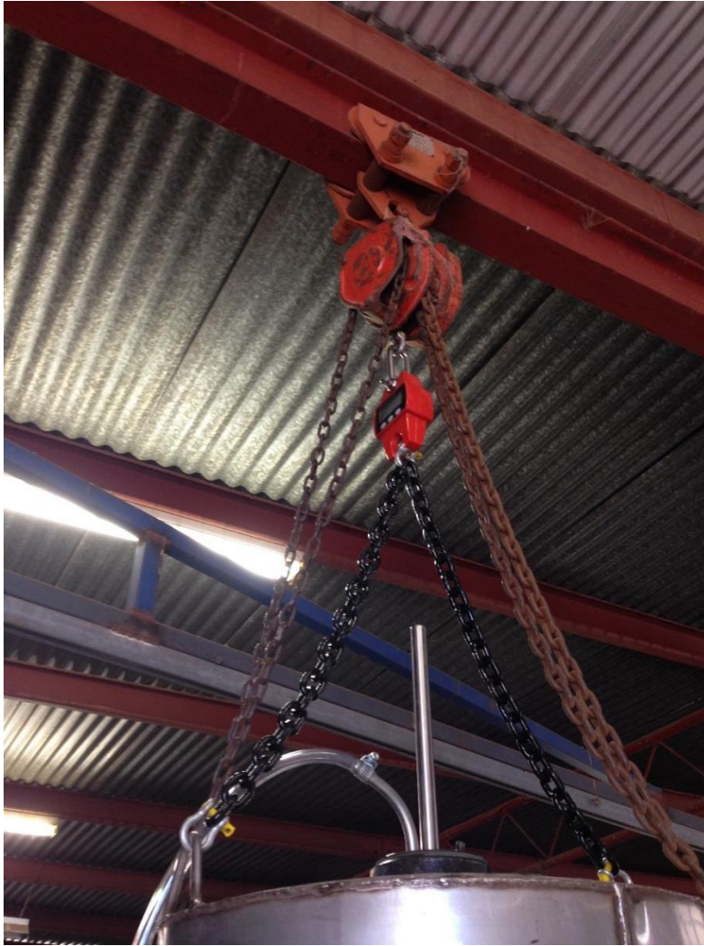
Figure 5-3 Crane scale rigged in position
