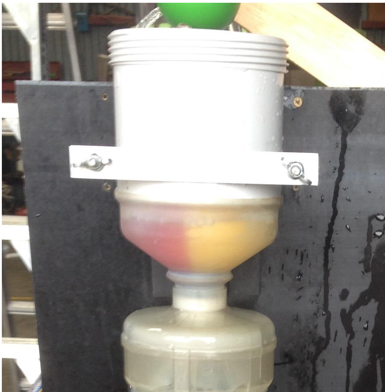
Figure 7-1 Ball shown in position that would cause leakage
