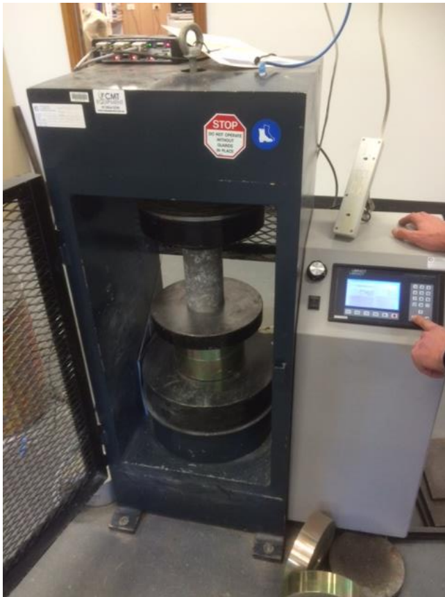
Figure 5-7 Sample setup for Compressive Strength Test
