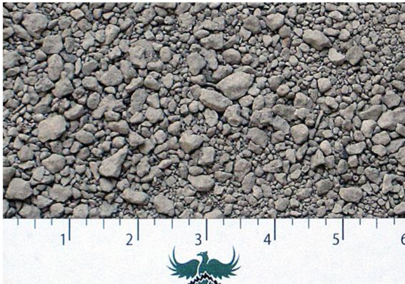
Figure 2-5 Blast Furnace Slag before grinding process ( www.phxslag.com )
