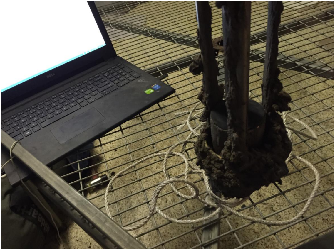
Figure 44: Photo from testing showing the clay sticking to the proctor hammer; reducing the compactive effort per blow
