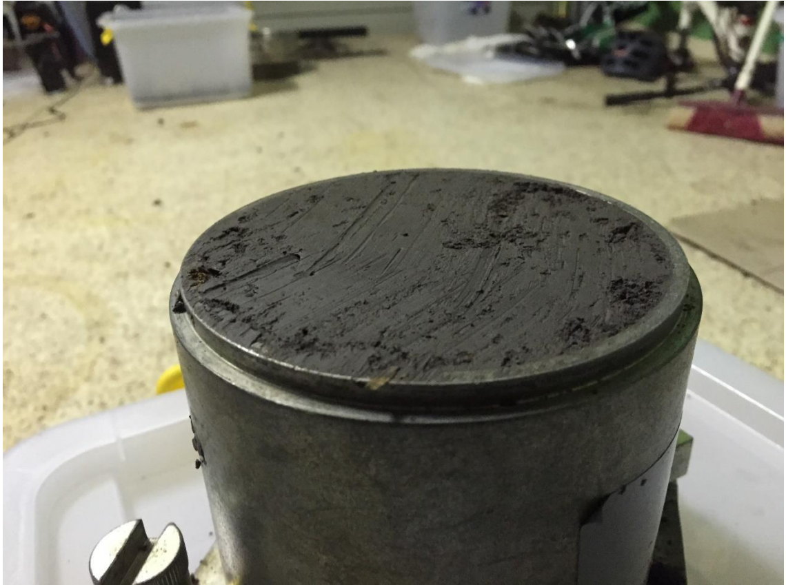
Figure 43: Surface of the soil after proctor compaction has occurred and the sample has been cut at the level of the mould
