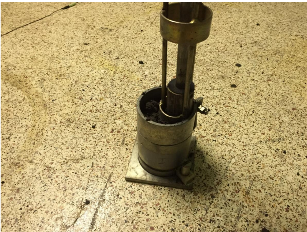
Figure 42: Image showing the application of the proctor hammer to the soil (before first blow)
