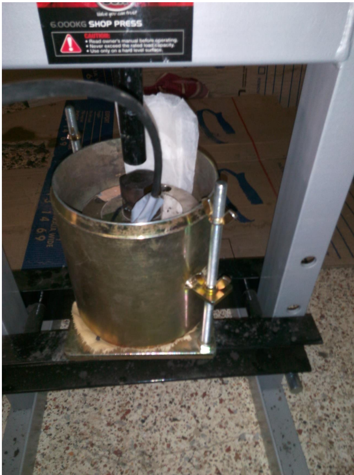
Figure 45: Picture showing the uniaxial compression test
