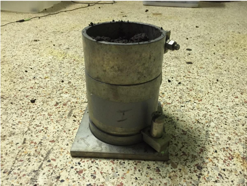
Figure 41: Image showing the proctor mould filled with uncompact soil
