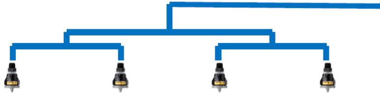
**Figure 3–14: A schematic drawing showing how the water supply hose was repeatedly divided in an identical manner for each of the sprinklers.**
