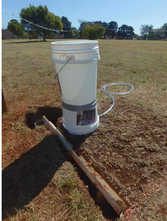
**Figure 3–8: The ‘bucket infiltrometer’ used as a reserve sprinkler infiltrometer,.**
