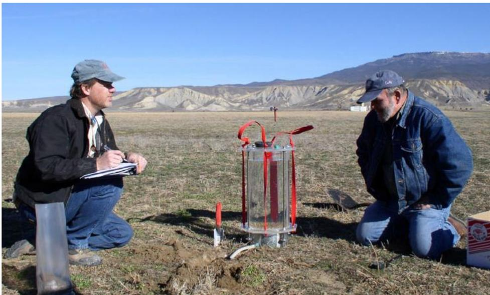
**Figure 3-7: A Cornell Sprinkler Infiltrometer in use (Molacek et al. date unknown).**
