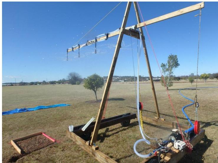
Figure 4–7: Photo of the mobile rig with sprinklers running. Note the flowmeter and pressure gauge at the bottom right.
