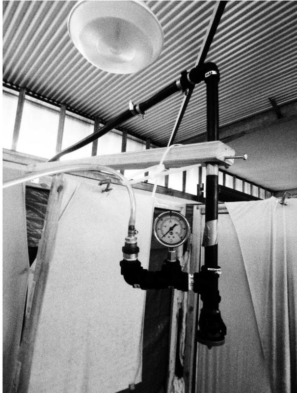
**Figure 3-5: Sprinkler head set-up, with the pressure line to primary pressure gauge and the secondary pressure gauge shown.**
