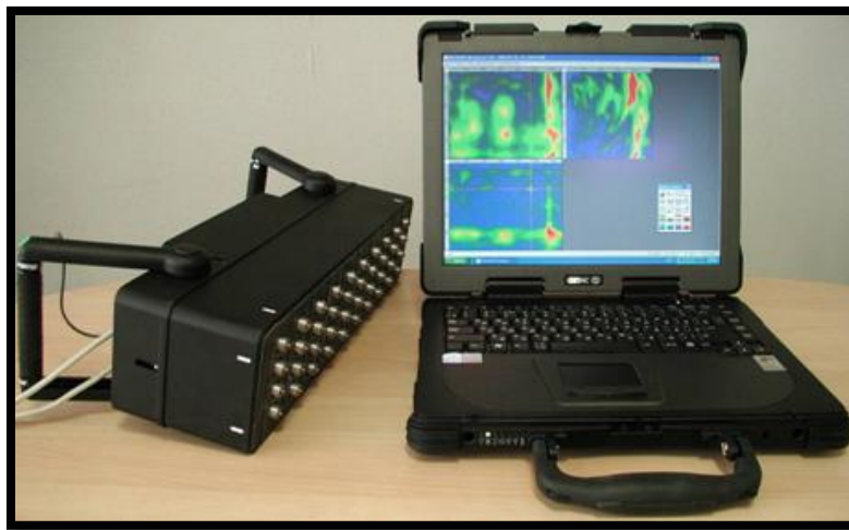
Figure 1: Low-frequency ultrasonic tomograph for concrete testing (BISHKO, SAMOKRUTOV et al. 2010)
