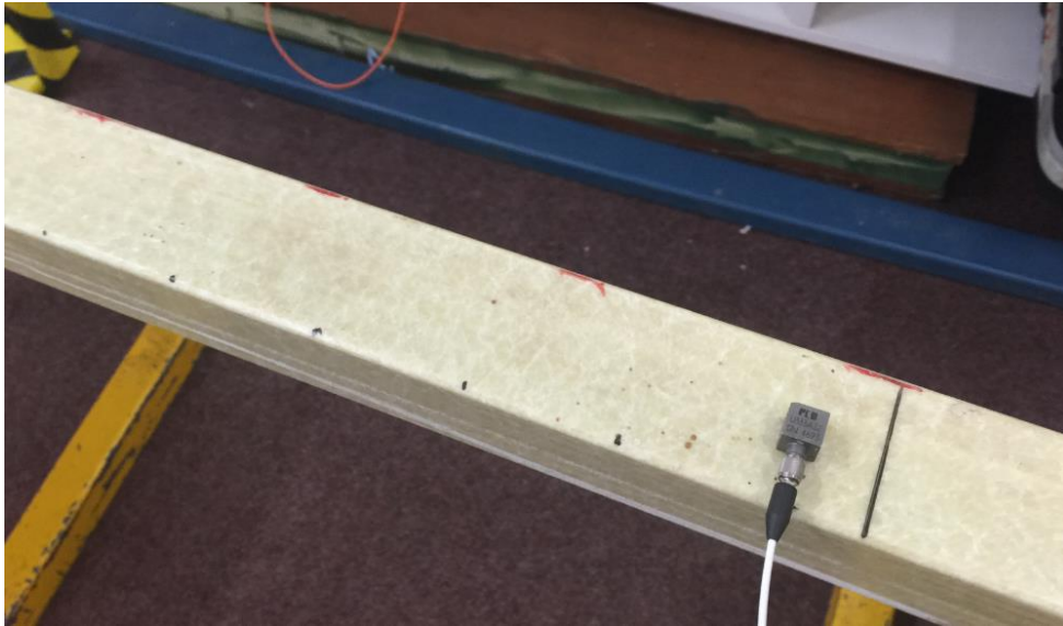
Figure 26: USQ supplied marked composite beam with accelerometer fixed in place
