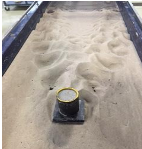
Figure 5.19 Three collars upstream after 2hr testing
