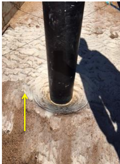
Figure 5.3 Upstream view of erosion after initial testing of 30 mins.
