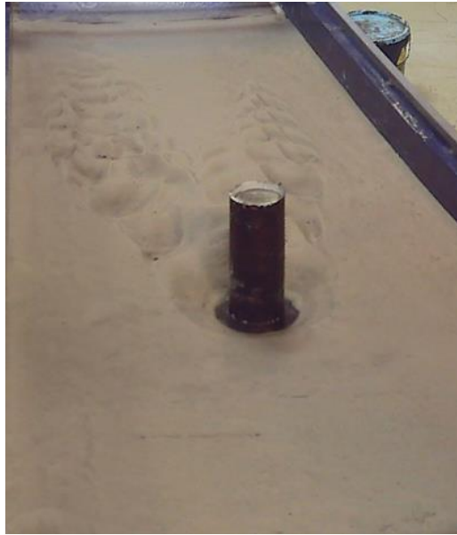
Figure 5.4 Erosion around control pier after 2hrs of testing
