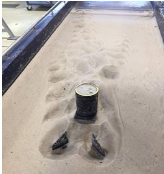
Figure 5.9 Inward vanes & attached plate upstream photo after 2hr testing
