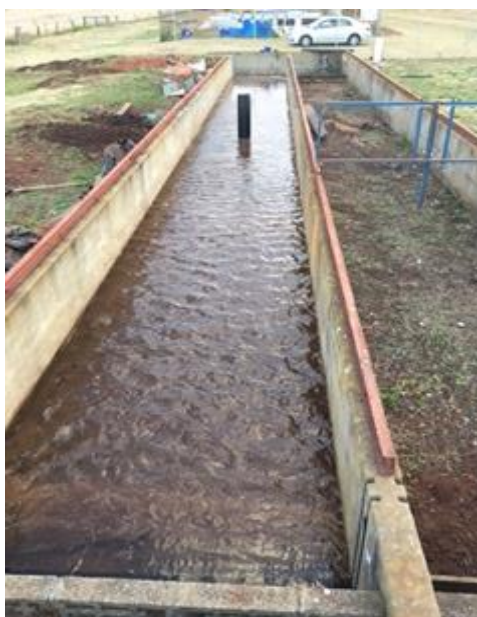
Figure 5.1 Large flume showing water flowing in the initial trial
