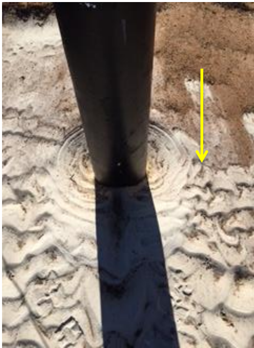
Figure 5.2 Downstream view of erosion after initial testing of 30mins.
