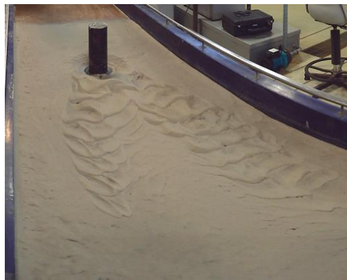
Figure 5.5 Erosion behind control pier after 2hrs of testing
