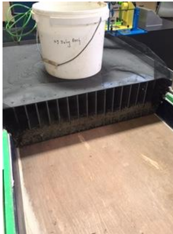
Figure 4.16 Baffles and Fly Screen Mesh for Laminar Flow
