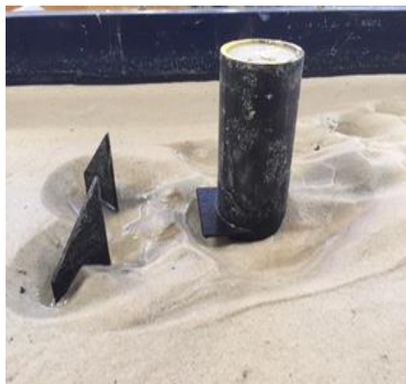
Figure 5.10 Inward vanes & attached plate side view photo after 2hr testing
