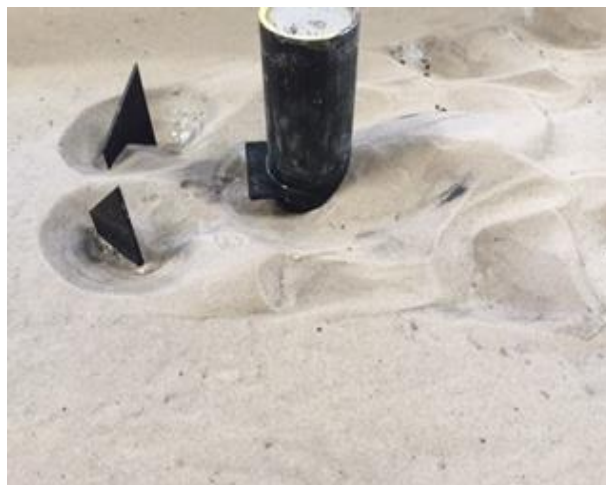
Figure 5.15 Outward vanes & attached plate side view photo after 2hr testing
