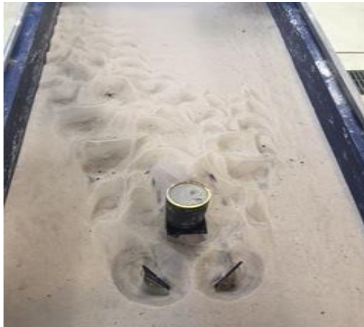
Figure 5.14 Outward vanes & attached plate upstream photos after 2hr testing
