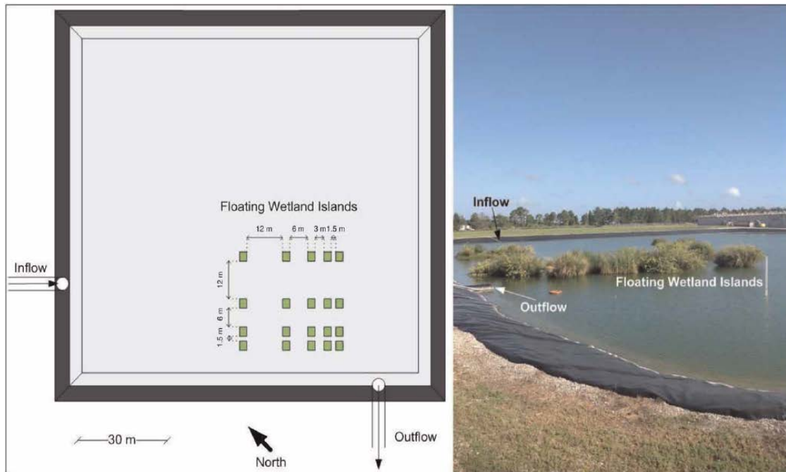
Figure 2.6-3 Pasco County Floating Treatment Wetland
