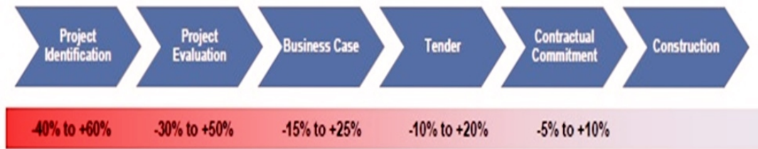
Figure 2.1: Anticipated Cost Estimation Accuracy During the Project Lifecycle (Source: Evans and Peck 2011)
