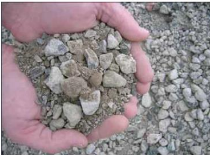
Figure 2: Crushed Concrete (Department of Victoria Roads 2011)
