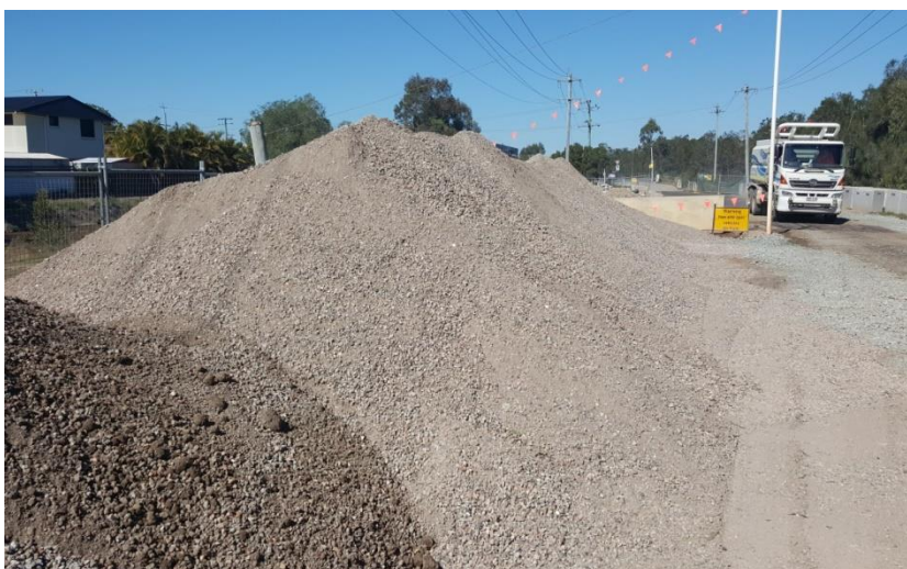
Figure 16: Crushed Concrete Stockpile
