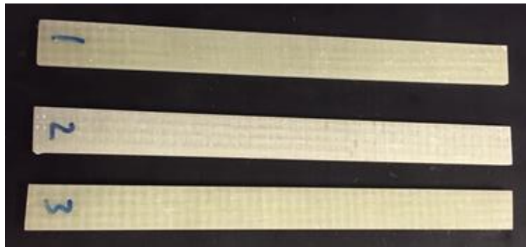
Figure 47: Material Property samples 12 ply 3 x (25 x 250)
