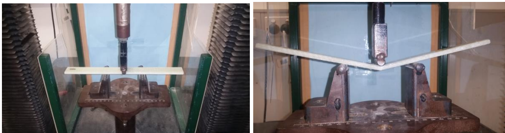
Figure 53: Flexure Test Pre and Post Test
