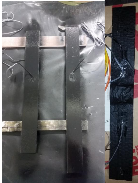
Figure 71: All three Samples Sprayed Black in preparation for thermographic testing
