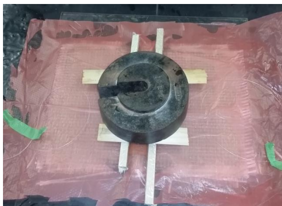
Figure 62: Controlling the shape of the 2 nd Tensile Sample
