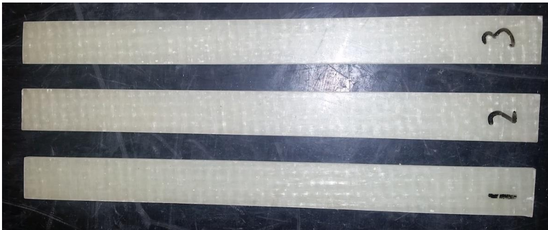
Figure 52: Three Samples Tested in three point bending
