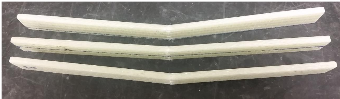
Figure 56: Flexure Fracture at Outermost Layer.
