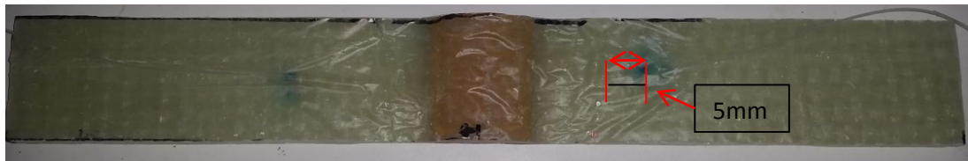
Figure 37: Placement of FBG
