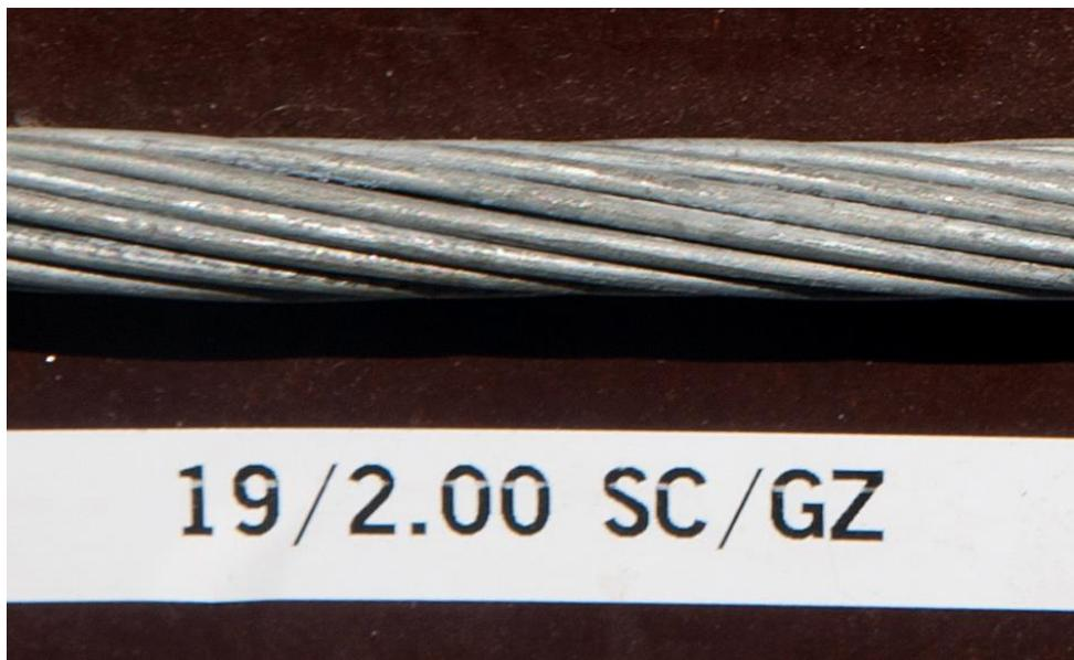
*Figure 19: A close up photograph showing the typical surface characteristics of the actual galvanised steel conductors tested.*
