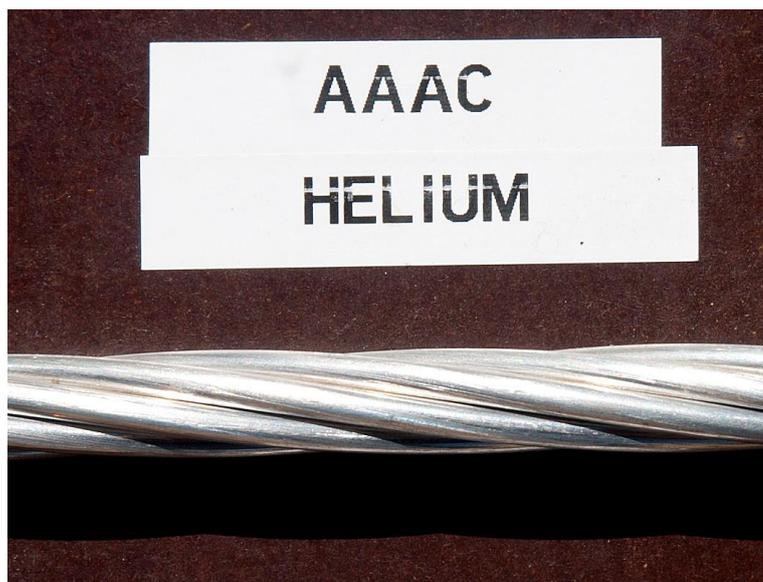
*Figure 21: A close up photograph showing the typical surface characteristics of the actual aluminium and aluminium alloy conductors tested.*
