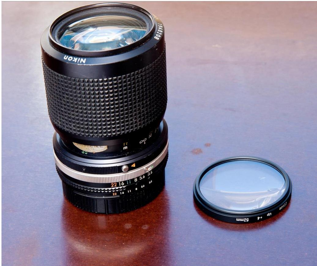
Figure 16: The original Nikkor 35-105mm lens on left and 100mm achromatic lens on right
