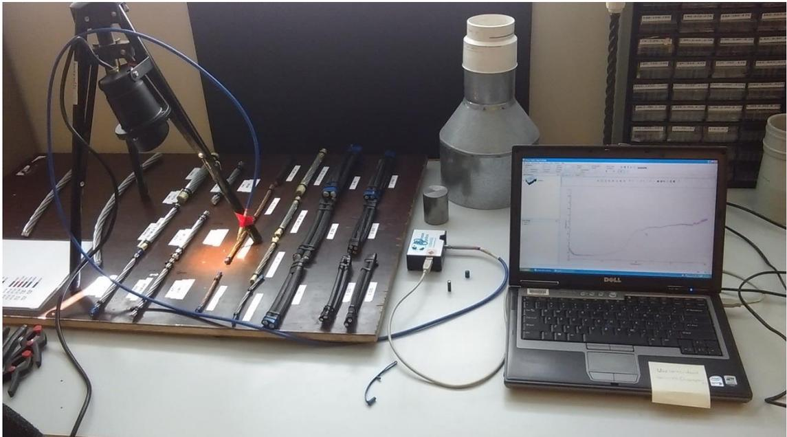
Figure 14: Actual setup for spectral measurements using an Ocean Optics USB 4000.
