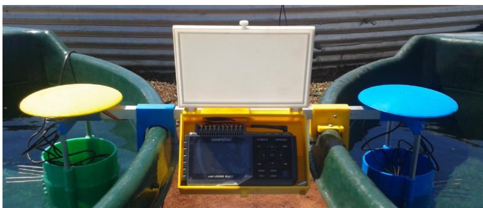
Figure 3.15: Test Rig support the data logger & thermocouple vessels
