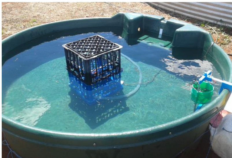
Figure 3.25: Imposing a cold surface film was achieved by including a bilge pump in one tank
