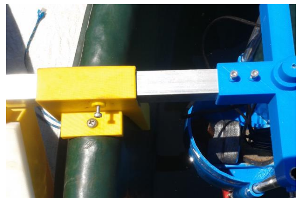
Figure 3.23: A single self-tapping screw held the test rig in position
