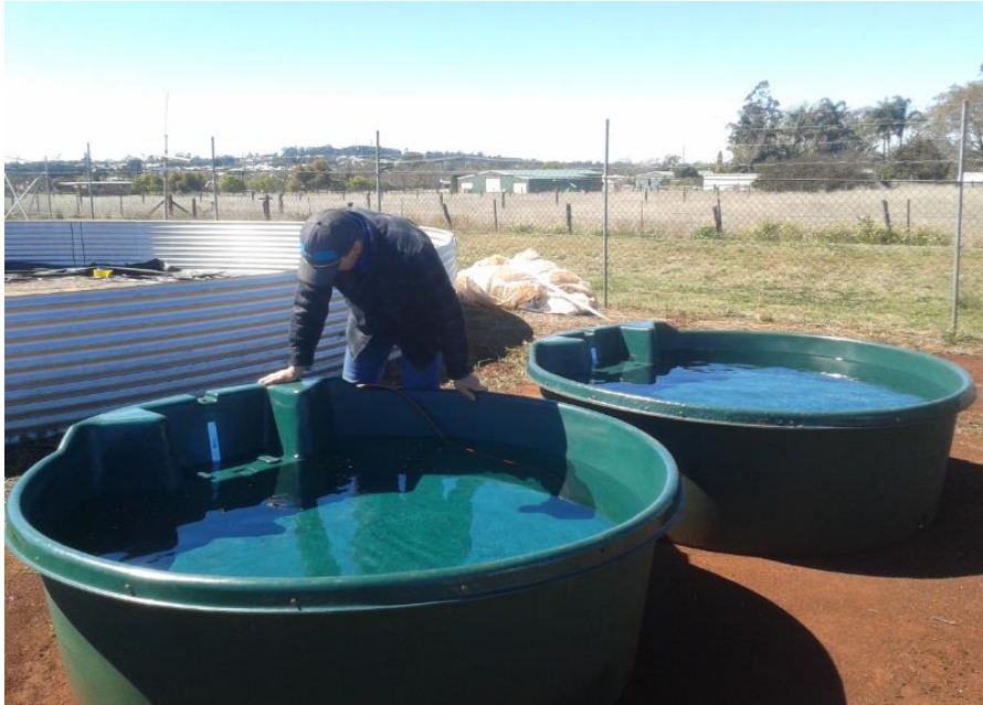
Figure 3.27: Monitoring evaporation loss in the tanks
