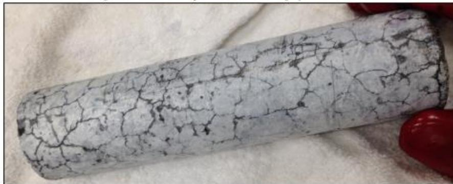
*Figure 4.2 – ASR replication, cracking after 11 weeks.*
