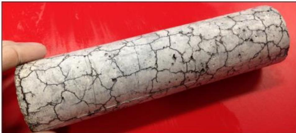
*Figure 4.3 – ASR replication, cracking after 16 weeks.*
