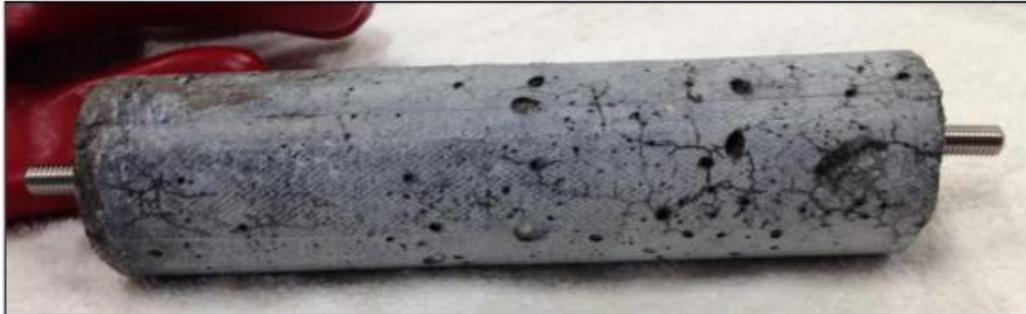
*Figure 4.1 – ASR replication, cracking after 7 weeks.*
