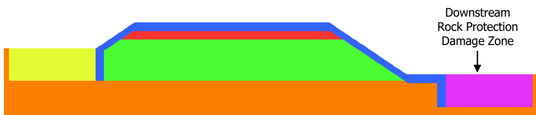
Figure 4.35: Downstream Rock Protection Damage Zone
