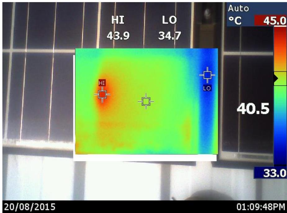
Figure 4.8 - Early cell failure signs 8°C hot spot approximately, less than 10% cell coverage.
