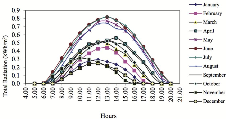
Figure 2.11 - Example of average hour solar irradiation over 12 months (Ekren, 2011).
