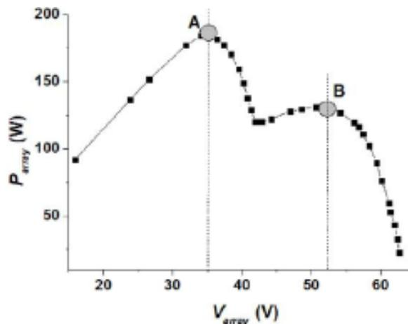
Figure 2.26 - P-V plot with the module covered (Hu *et.al*, 2013).
