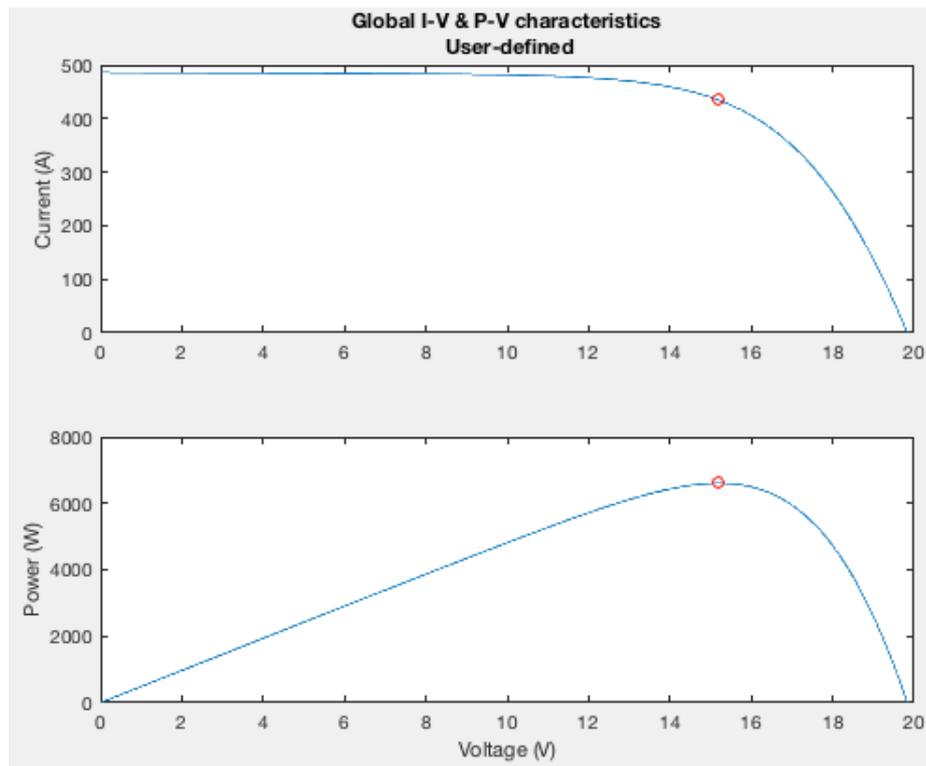
Figure 5.2 - Total output of 36 x dirty panels @ 42°C.
