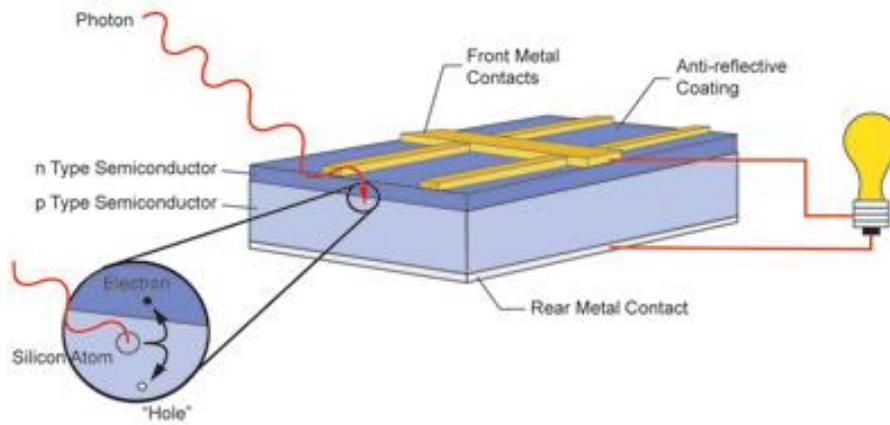
Figure 1.2 - PV effect basic diagram (Viridian, 2016).
