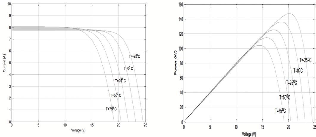
Figure 2.17 - (Left) I-V plots at set temperatures and allocated irradiance (Right) P-V plots Module's P-V plots at set temperatures and allocated irradiance (Krismadinata *et.al*, 2012).
