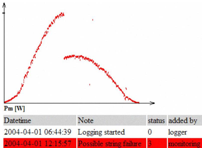
Figure 2.21 - Data showing how detections are logged (Kolodenny *et.al* 2008).
