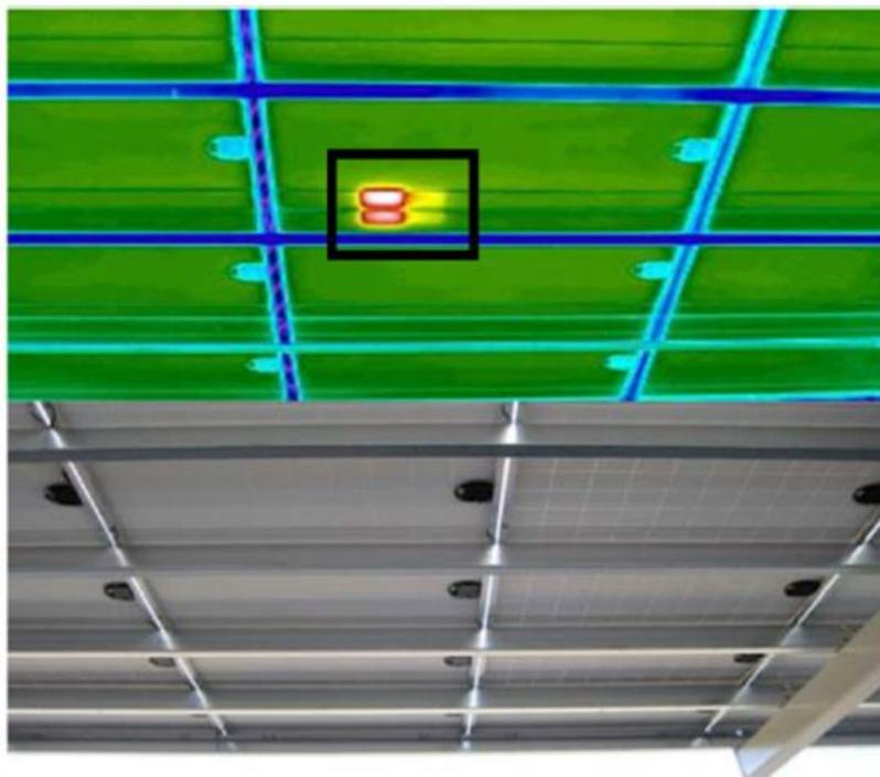
Figure 2.23 - Overheated cells taken from underneath an large PV structure (Denio, 2011).
