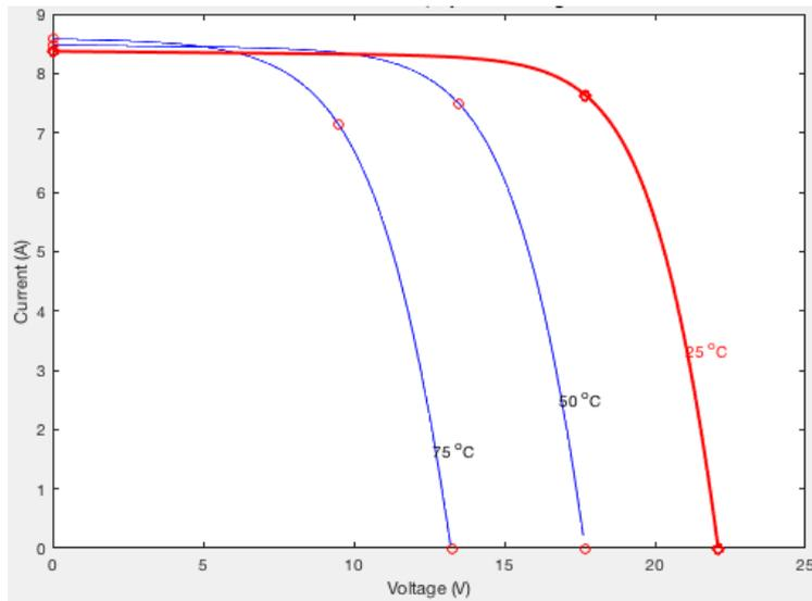
Figure 3.7 - Kyocera KD135GH-2PU I-V output MATLAB model @1000W/m<sup>2</sup> at various cell temperatures.
