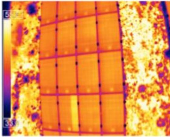
Figure 2.7 - Failed bypass diode, Thermography 1/3 of panel failed (Tsanakas 2016).
