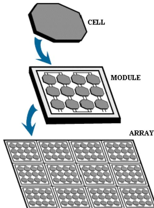
Figure 1.3 - PV array deconstruction diagram (NASA Science, 2016).
