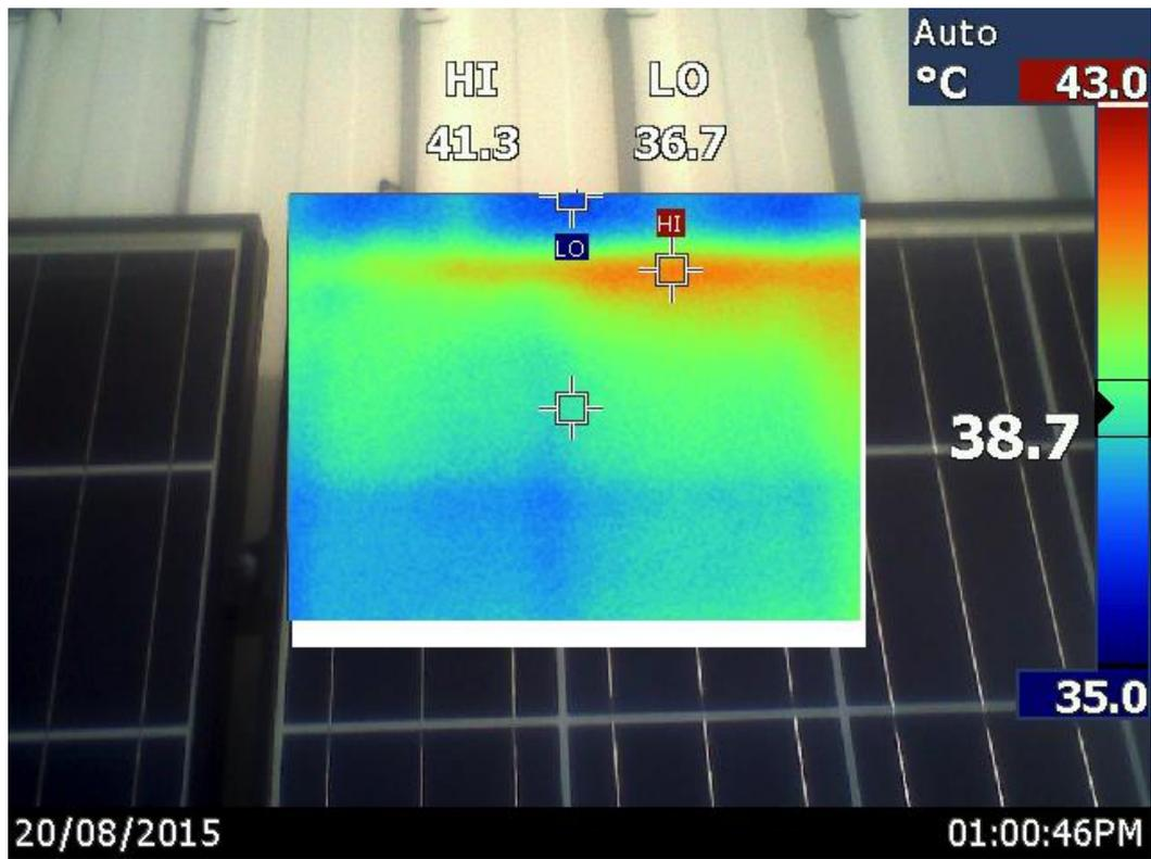
Figure 4.5 - Effects of ingress and dirt on array.
