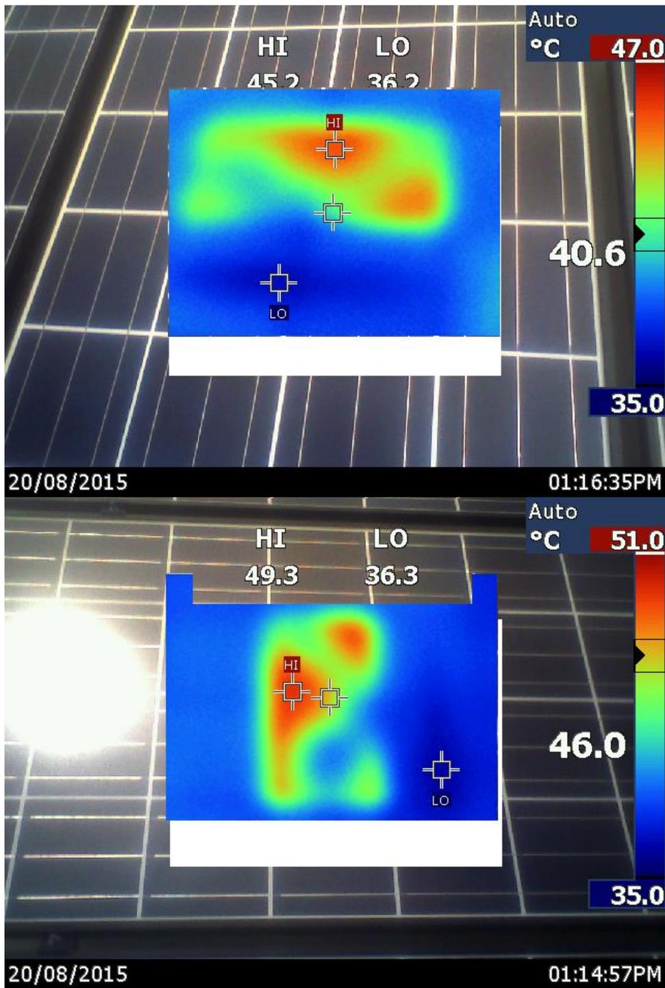
Figure 4.10 - Two images of the 2<sup>nd</sup> detection dual cell failures – 13.3°C max hot spot, approximately 50% cell coverage.
