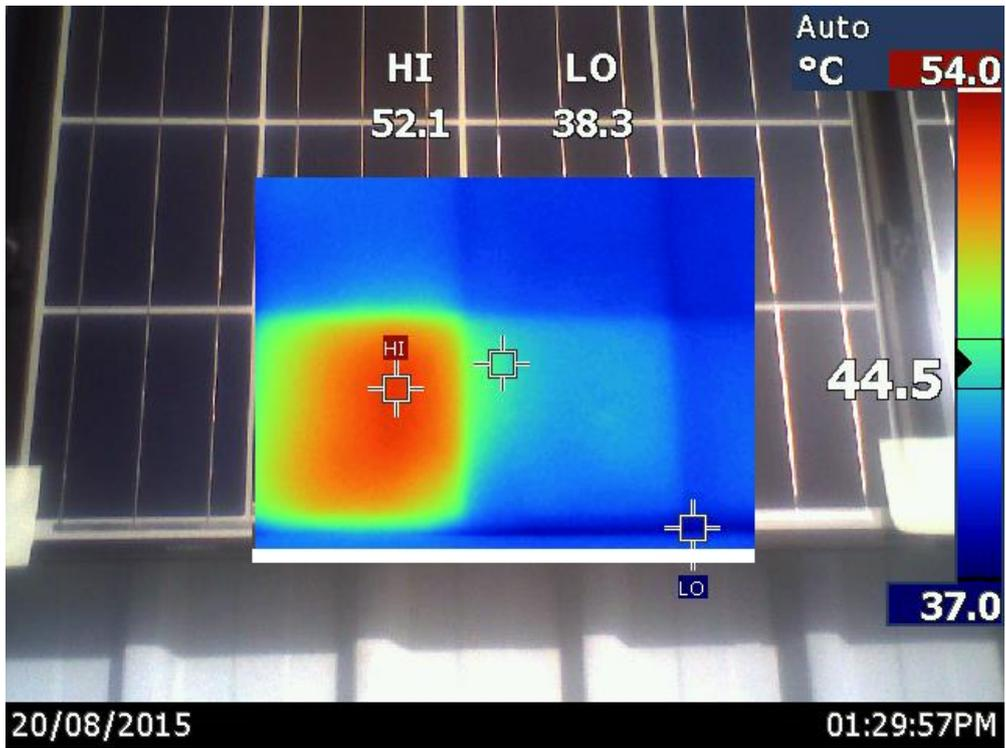
Figure 4.13 - 5<sup>th</sup> detection 16°C hot spot approximately 95% cell coverage.
