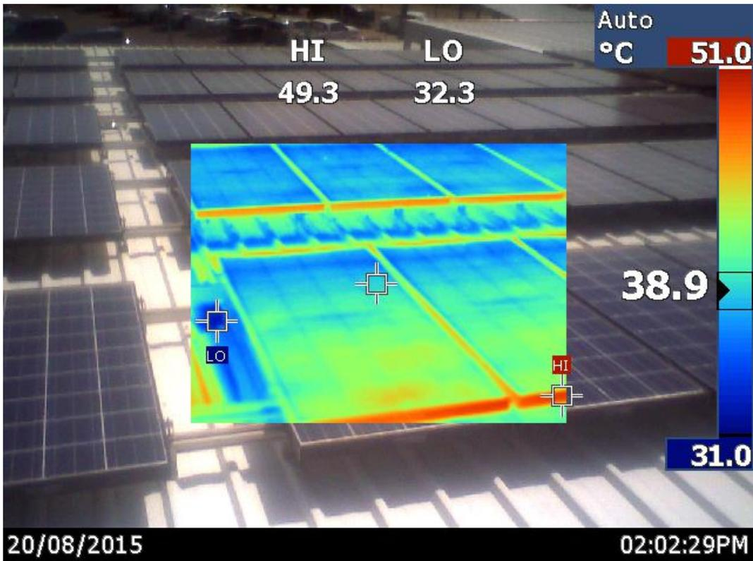
Figure 4.3 - The infrared image and photo image are out of sync.
