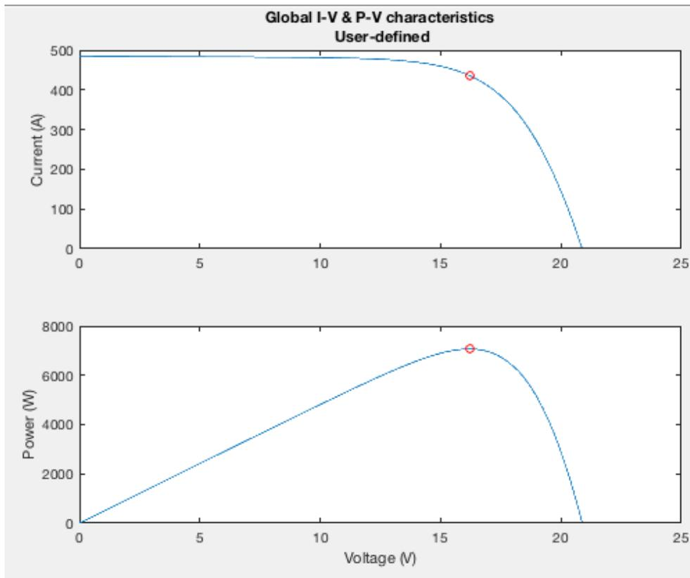
Figure 5.1 - Total output curves at 61°C hottest single cell model.
