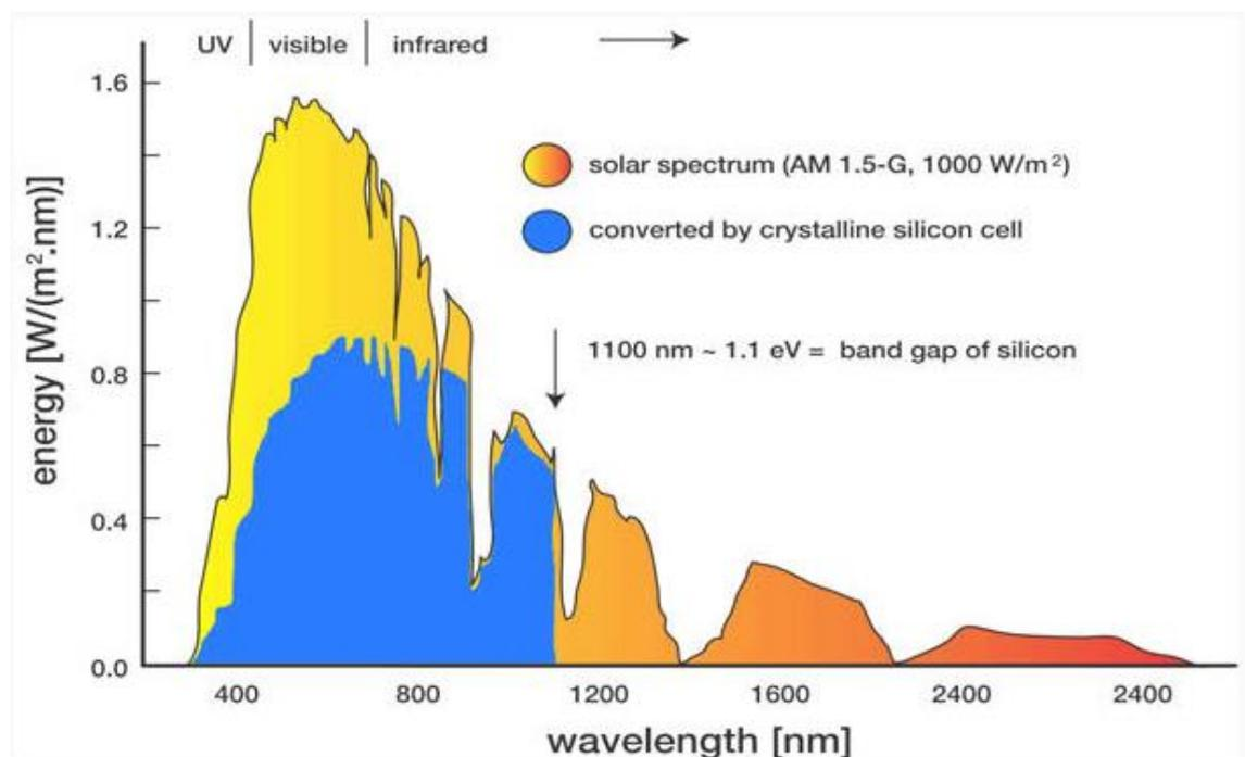
Figure 2.3 - Typical crystalline silicon cell wavelength conversion spectrum (Viridian, 2016).
