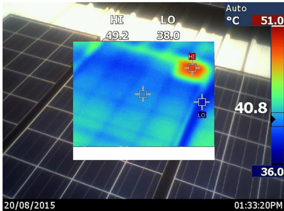
Figure 4.15 - Same 6<sup>th</sup> detection from distance hot spot stands out.
