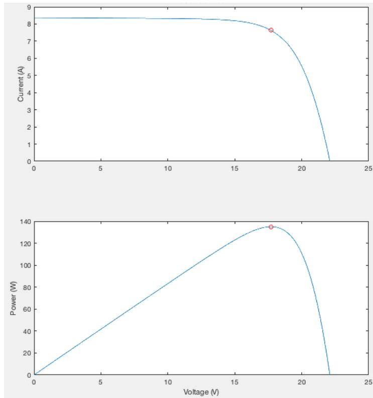
Figure 3.1 - Single panel @1,000W/m<sup>2</sup> at 25°C – 135.04W.
