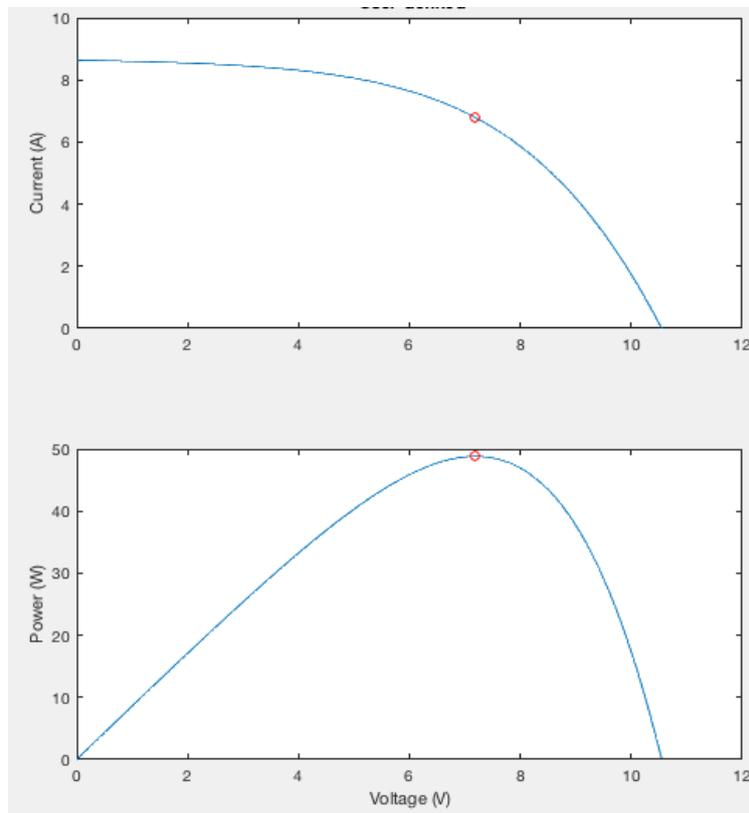
Figure 3.10 - Single panel @1000W/m<sup>2</sup> and 100% panel 90°C – 48.80W.
