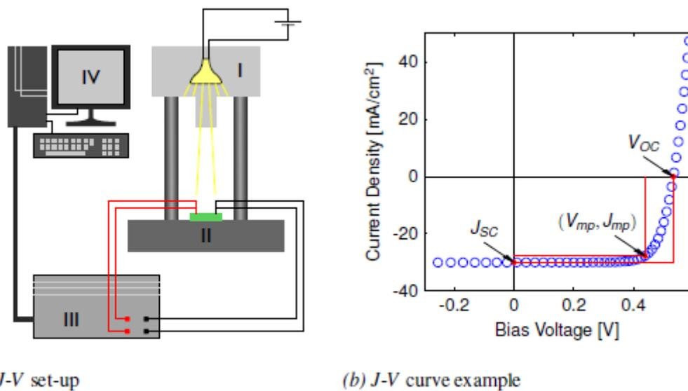
Figure 2.15 - (a) A schematic drawing of a typical J-V measurement set up (solar simulator); (b) and a typical illuminated J-V characteristics. (Acta Universitatis Upsalensis Uppsala, 2008).
