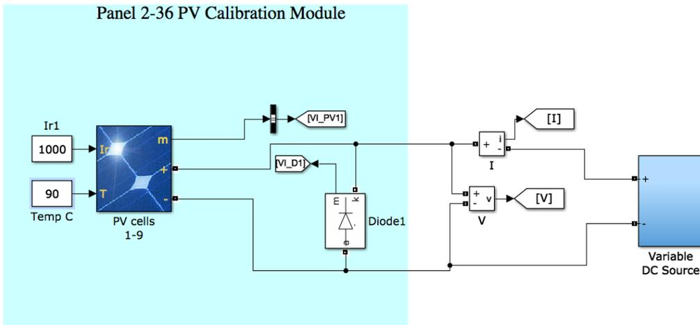
Figure 3.11 - Panel 2-36 calibration model.
