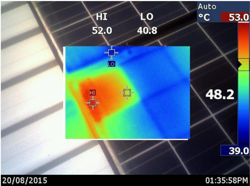
Figure 4.14 - 6<sup>th</sup> detection - 16°C hot spot approximately 95% cell coverage.
