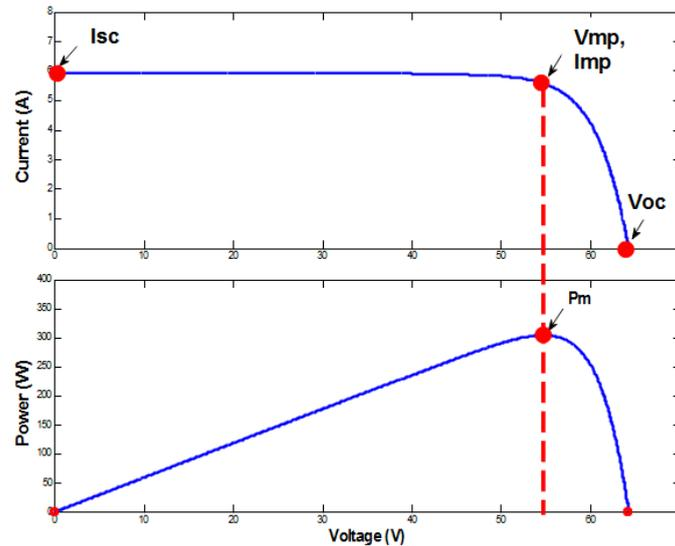
Figure 2.31 – P-I and P-V curve showing maximum power point relationship (Mathworks, 2016).
