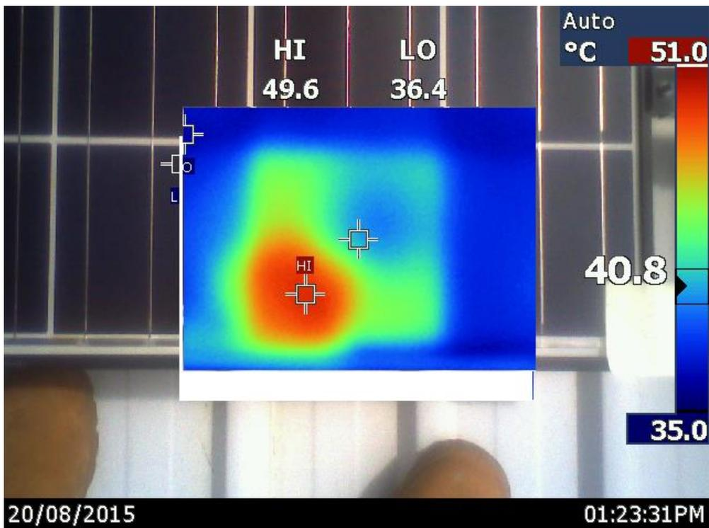
Figure 4.12 - 4<sup>th</sup> detection 13.6°C hot spot 40% cell coverage.
