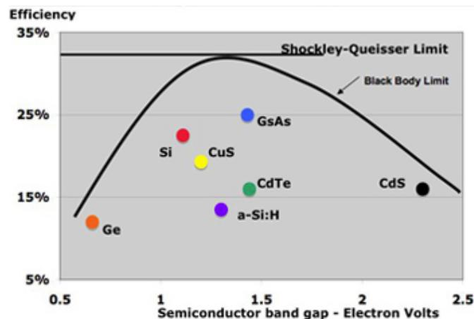
Figure 2.1 - Panel type efficiencies and Shockley-Queisser limit for a single junction cell (Solar Central, 2016).
