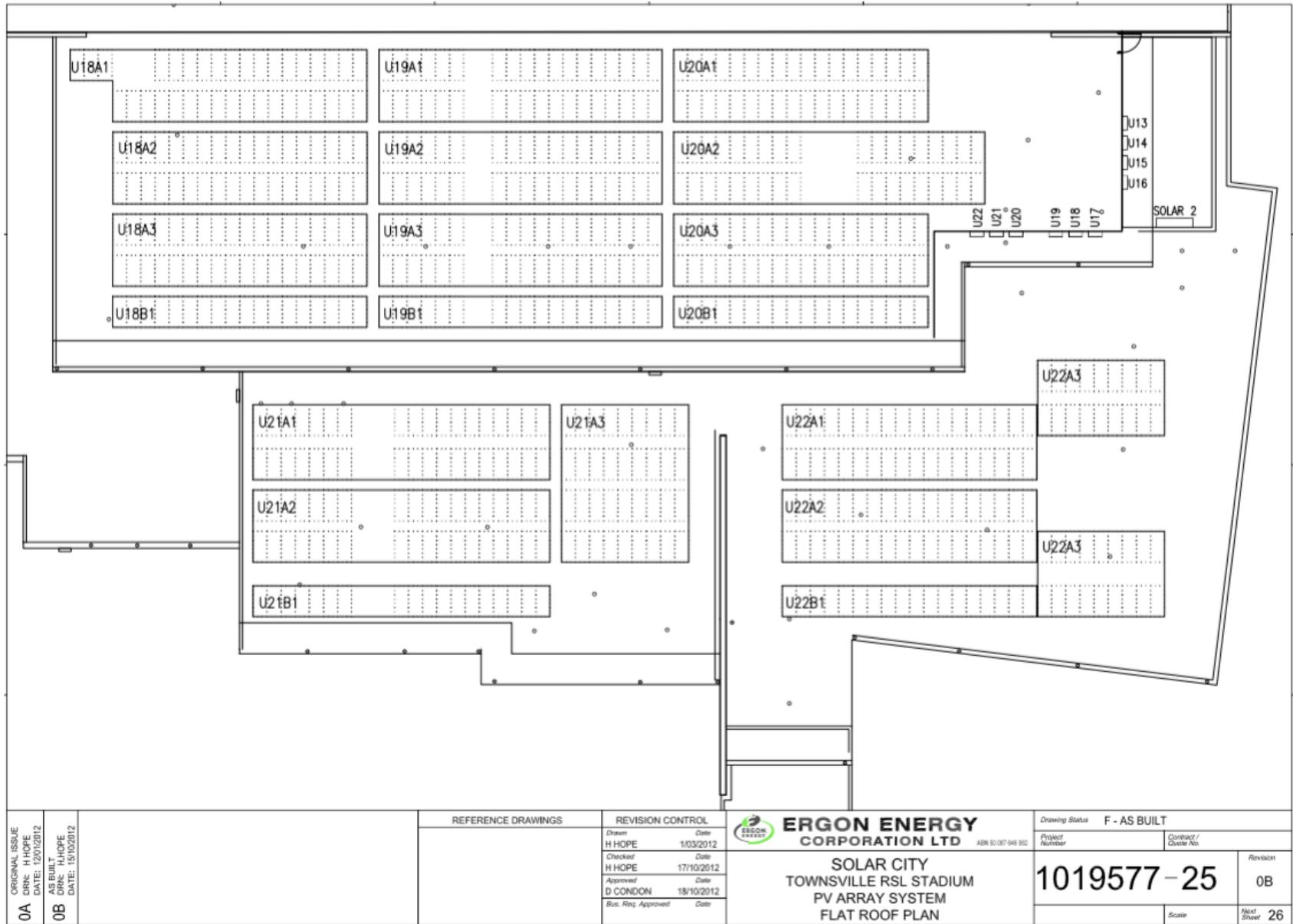
Figure 0.5 - Panel and inverter layout Townsville RSL Stadium flat roof plan.
