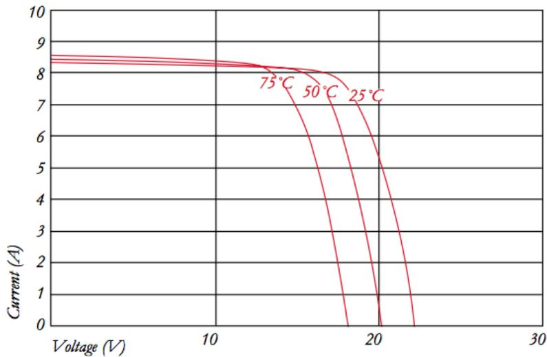
Figure 3.8 - Kyocera KD135GH-2PU module I-V data sheet characteristics @1000W/m<sup>2</sup> at various cell temperatures (Kyocera, 2010).
