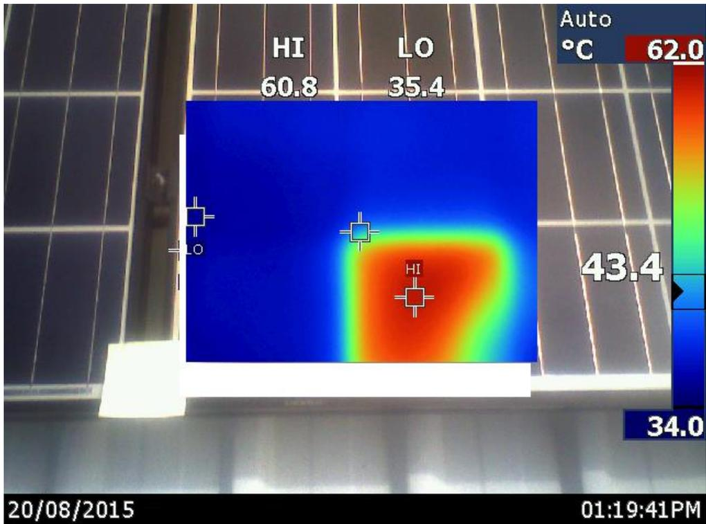
Figure 4.11 - 3<sup>rd</sup> detection – 24.8°C max hot spot 90% cell coverage.
