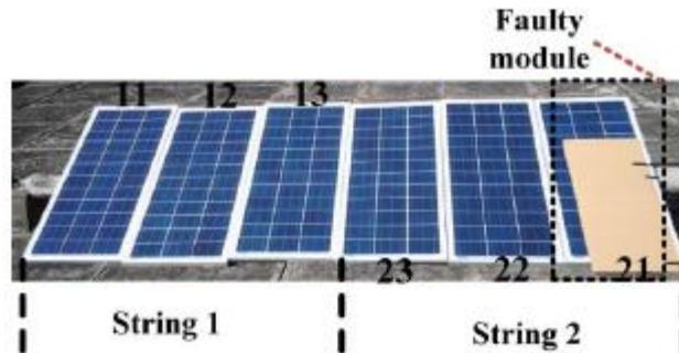
Figure 2.24 - Simulation of faulty panel using a shade shield (Hu *et.al*, 2013).
