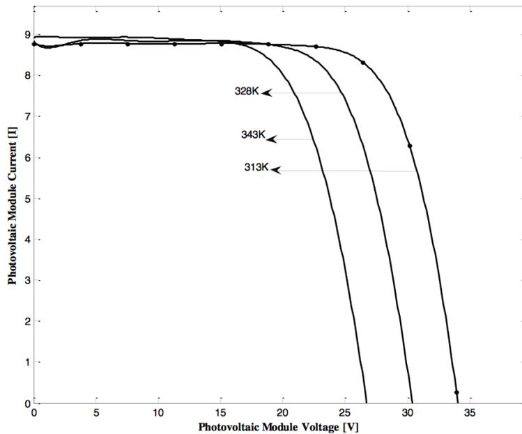
Figure 2.19 - Temperature effects on I-V curve (Savitha, 2014).
