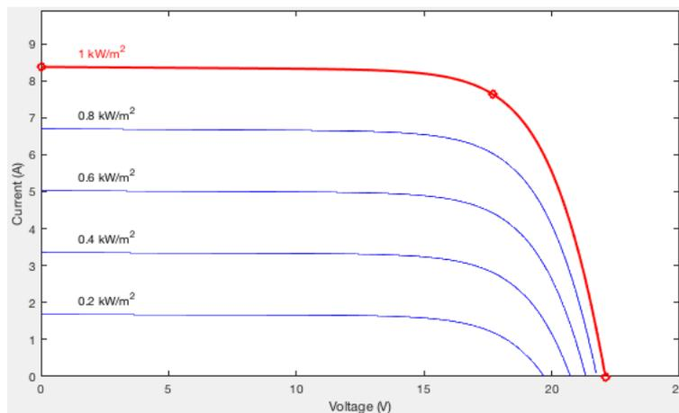
Figure 3.5 - Kyocera KD135GH-2PU I-V output MATLAB model @25°C and multiple irradiances.
