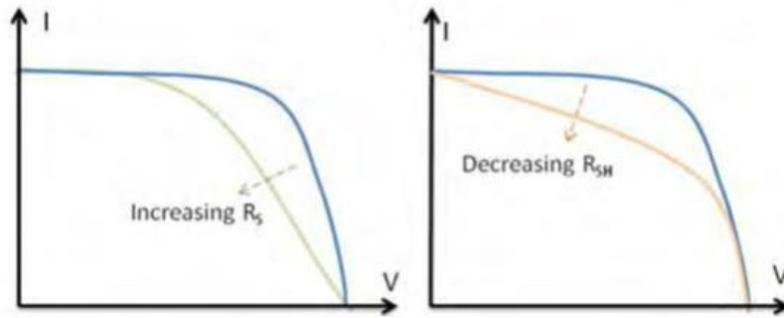
Figure 2.14 - Resistance effects on the I-V curve. (J.O.Odden, 2014).
