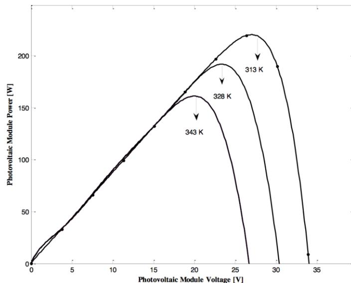
Figure 2.20 - Temperature effects on P-V curve (Savitha, 2014).
