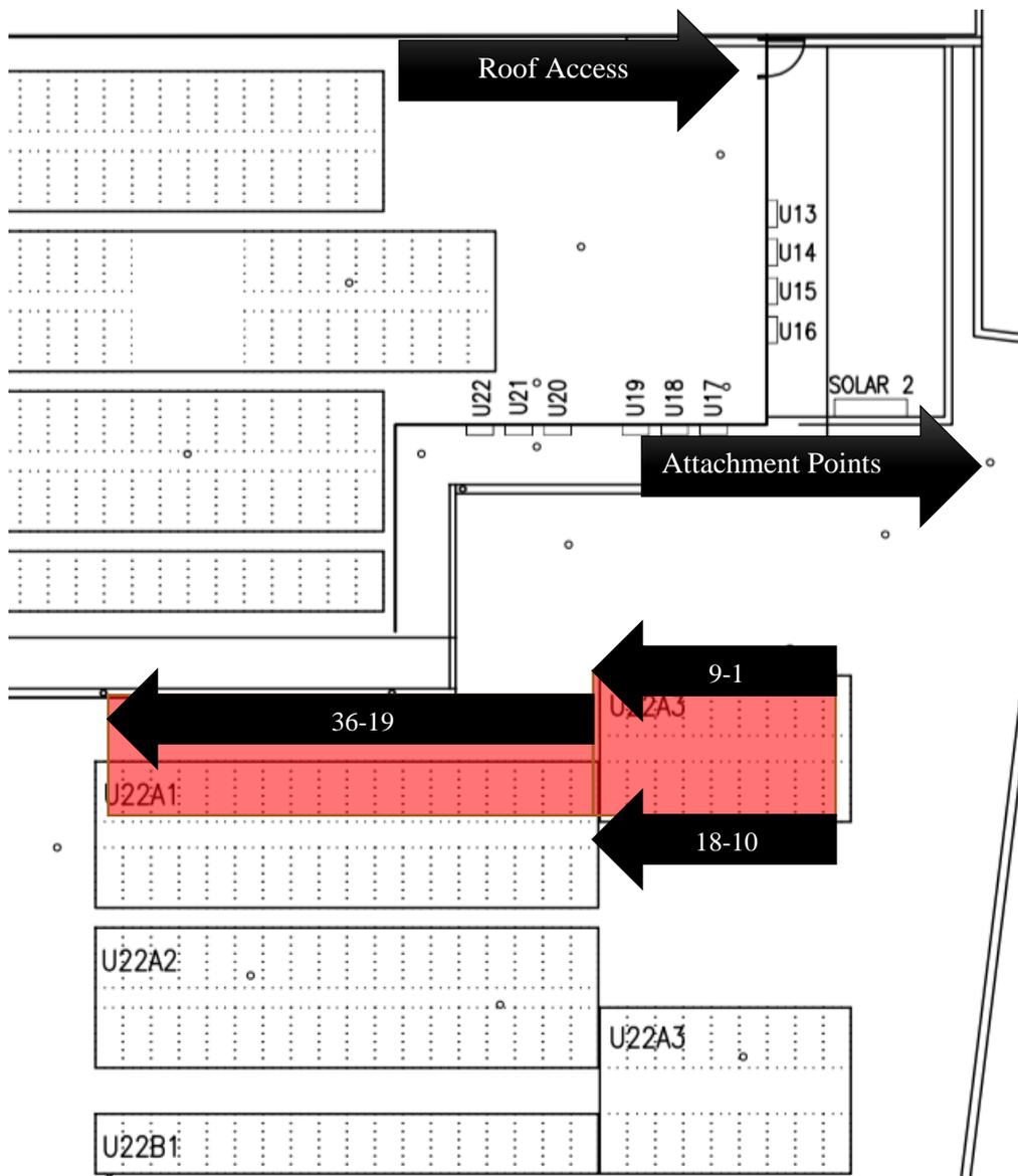
Figure 4.1 - Zoom of layout (Red) indicating the 36 panels scanned, access and attachment points (Appendix B full size).
