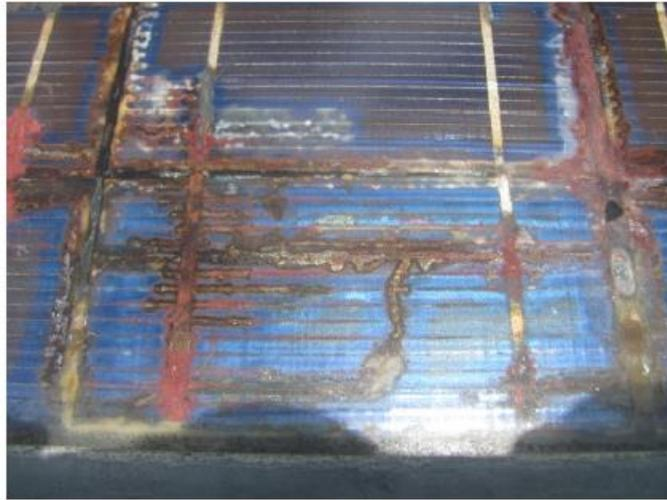
Figure 2.29 - 85/85 cell degradation after 3500 hours in harsh conditions (Wohlgemuth *et.al*, 2010).
