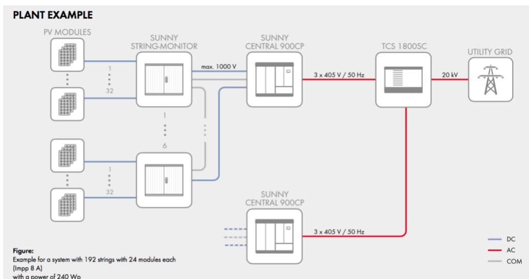
Figure 2.30 - Sunny string-monitor plant example diagram (SMA, 2016)
