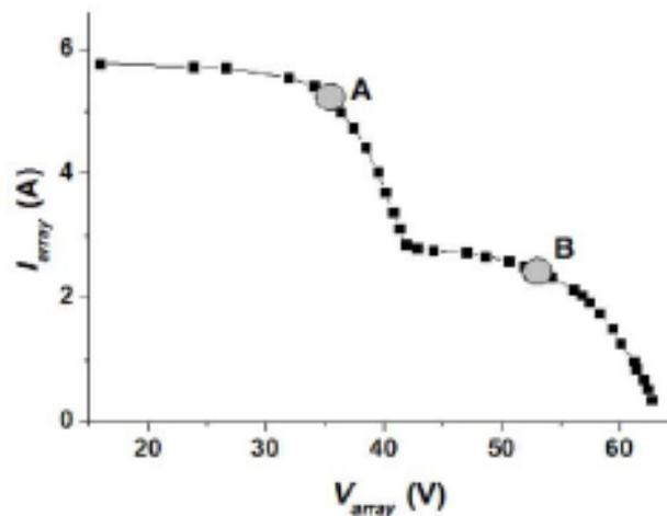
Figure 2.25 - I-V Plot with the module covered (Hu *et.al*, 2013).
