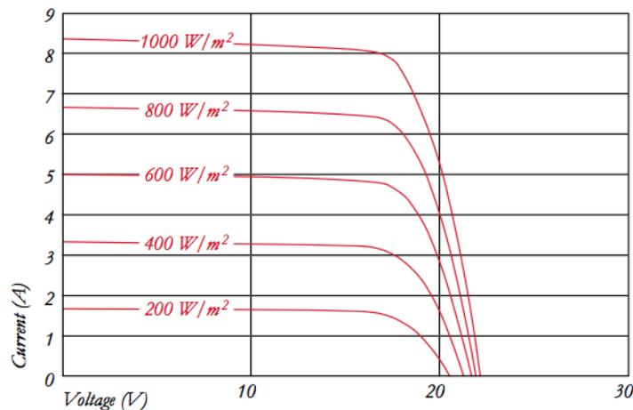
Figure 3.6 - Kyocera KD135GH-2PU I-V data sheet characteristics @25°C at various irradiance levels, (Kyocera, 2010).
