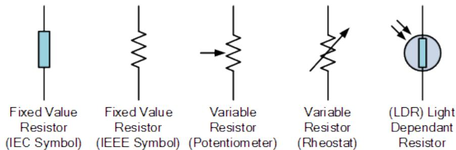
Figure 1.1 - Resistor symbol types (DC Circuit Theory, 2016).
