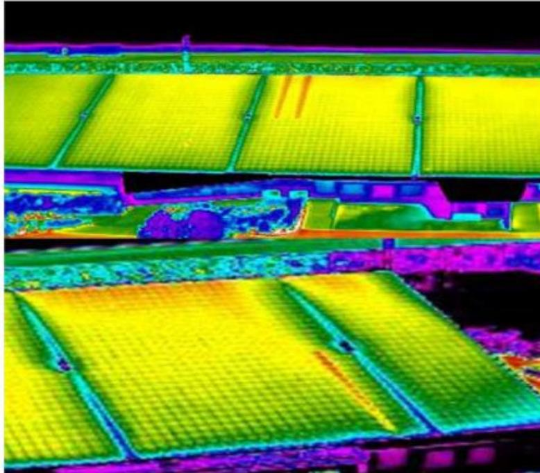
Figure 2.22 - Multiple panels with increased temperatures in this large PV system (Denio, 2011).
