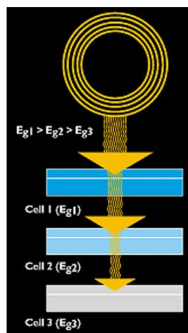
Figure 1.4 - Photovoltaic multi-junction layers (NASA Science, 2016).
