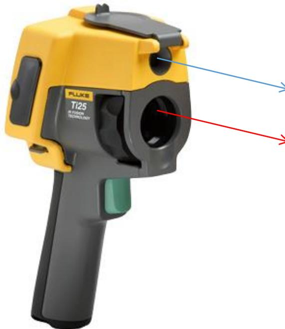
Figure 4.2 - Fluke Ti25 infrared thermal camera showing the top visual camera (blue) and bottom infrared lens (red) (Fluke, 2010).
