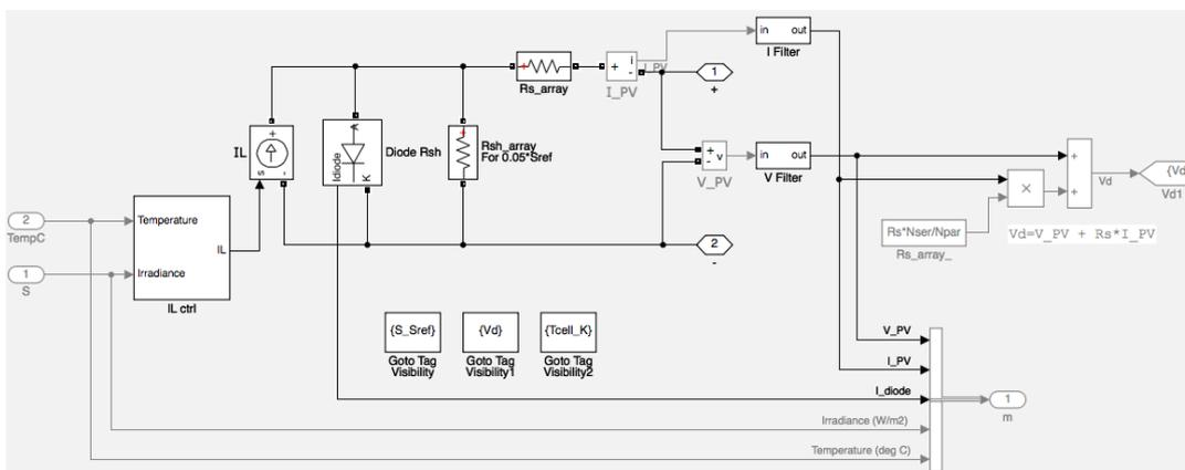
Figure 2.33 - Detailed Simscape PV array logic (Mathworks, 2016).
