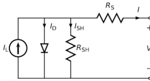
Figure 2.16 - Circuit model, using a series and parallel resistance and a single diode (Eitner *et.al* 2010).
