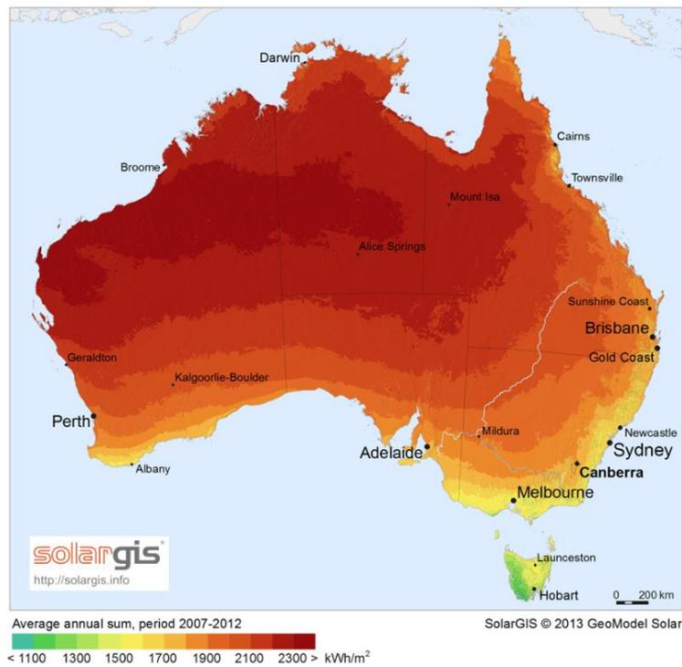
Figure 2.13 - Australia average global horizontal irradiation – (SolarGIS, 2013).
