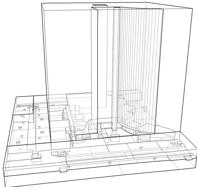
Figure 4.3 Wireframe model of the stratum lots excluding the bridge.
